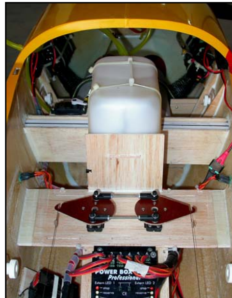
This general view shows the dual Rx Nicads and Powerbox installation, fuel tank fixing and hi-amp extension cables and sockets fitted into the fuselage sides for the ailerons.
