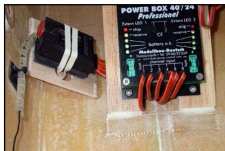
(above) NiCad packs are fitted to plywood plates on a thin rubber sheet, and secured with cable-ties.
