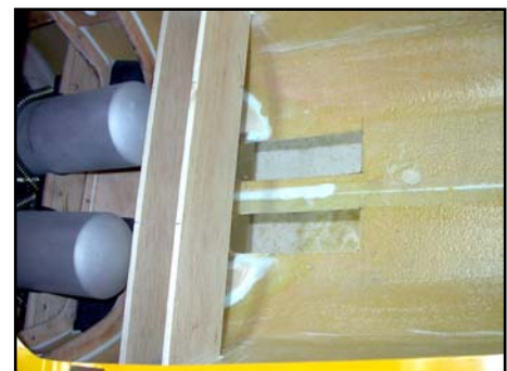
(below) Don't forget the 2 slots to allow the warm air from the mini-pipes to exit the fuselage.
