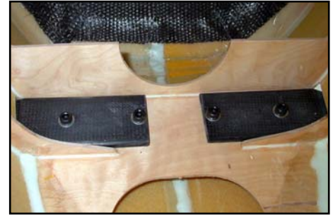
(above) Note: This photo shows the older type of front bulkhead, for the single mini-pipe system !
