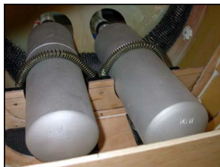
(above) Muffler mounting shown on a 'dummy' bulkhead for clarity
