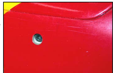
(above) Counterbore the 4 holes for the canopy bolts so that the heads sit against the plywood plates in the fuselage.
