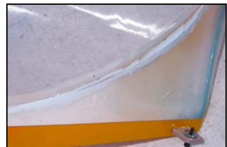
(above) Finally secure the canopy to the frame with an epoxy and microballoons mixture inside.
