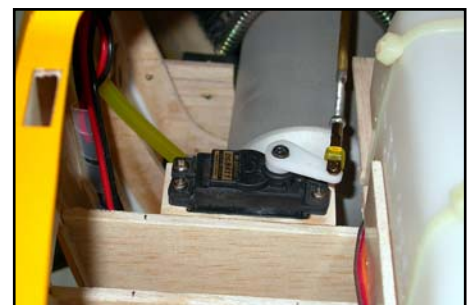
(above/below) Throttle servo mount assembled from milled plywood parts, and glued to the front of spar box on left of the fuel tank.
