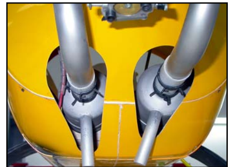
(above) Ensure enough cooling air can enter around the mini-pipes. Make the holes at least 12mm (1/2") bigger than the exhaust diameter.
