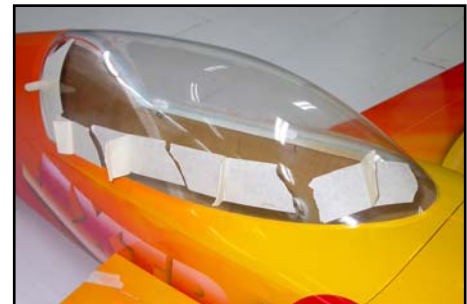
(below) Use masking-tape handles to pull the clear canopy tightly against the canopy frame while gluing it in position with a few small drops of thick CA.
