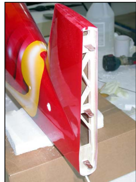
The lightweight fin-post has the phenolic rudder hinges already installed at the factory ensuring perfect alignment.
