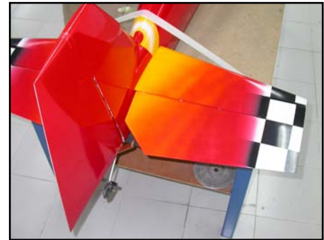
The lightweight fin-post has the phenolic rudder hinges already installed at the factory ensuring perfect alignment.
