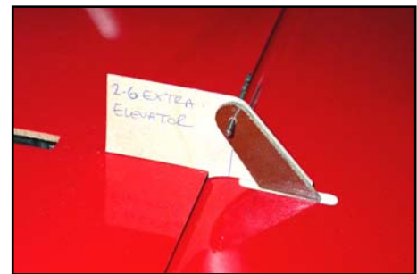
(below) Elevator horn alignment template from scrap plywood. Line is hinge axis. Use for both elevators to ensure same throws.
