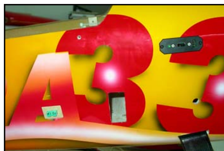
(above/below) Powerswitches are used for both the dual Rx & single Ignition Nicads, and fitted into the fuselage sides as shown here.
