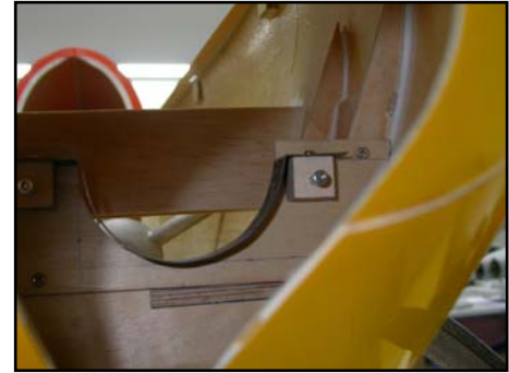
(below) Another view of the steel strip and blocks with M3 bolts taken thru' the firewall.
