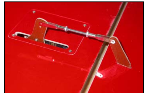
(below) The completed aileron linkage. Note locknuts used at both ends of linkage. Tygon safety tubes missing in this photo!
