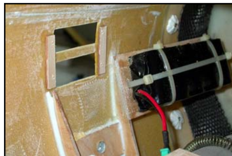
(above) NiCad packs are fitted to plywood plates on a thin rubber sheet, and secured with cable-ties.
