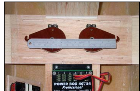
(above) Rudder horn roughed up with coarse sandpaper. Glue in with slow epoxy and milled fibre.
