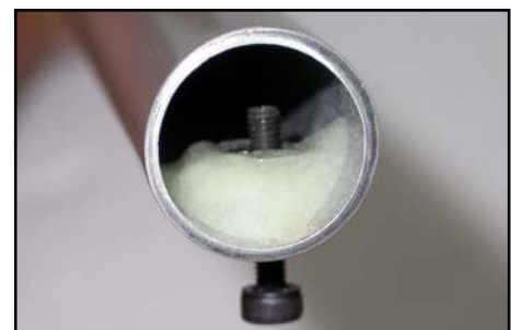
(below) M3 blind nut glued into elevator spar tube.
