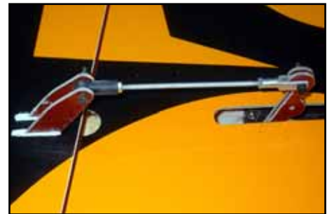
(below) An example of the linkage for the outer servo the SuperXtra wing, using the phenolic horns & linkage hardware supplied.
