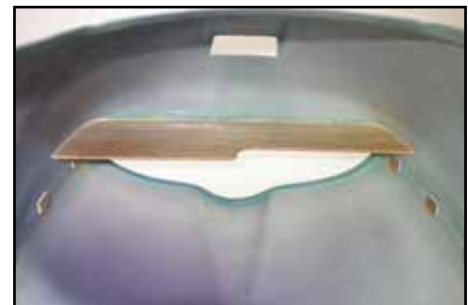
(above and below) A simple balsa sheet baffle will improve motor cooling considerably by making sure the air is directed through the cylinder cooling fins.
