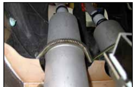
(below) View of the twin muffler mounting from behind.
