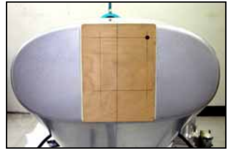
(above) Vertical centreline and the 1st hole to be drilled shown here. (below) The 4 holes for the motor mounting, and 1 for the linkage from the throttle servo.
