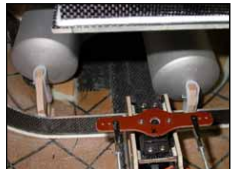
(above and below) For additional security, you can fit 'stops' behind both mufflers, so that they cannot move backwards. These are easily made from teflon tube and 6mm plywood blocks as shown.
