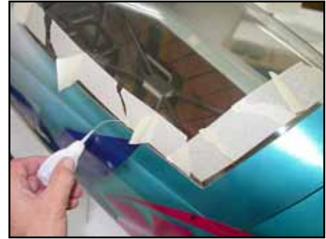
(above) The canopy is glued in place with CA, using masking-tape handles to pull it into place.
