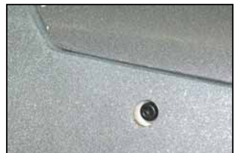
(above) Counterbore the 4 holes for the canopy frame bolts so that the heads sit against the plywood plates in the fuselage.
