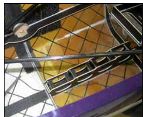
(above) Notch the ends to fit into the slots in the formers. (below) Completed Rudder tray and sub-formers glued in the normal position, with rear former in line with rear wing dowels.
