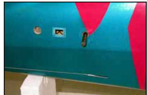
(above) Shows the pull-pull rudder cables in the slots, the carbon anti-rotation pin, hole for the 20mm \varnothing tube spar and the hole prepared for the servo extension cable connector mounting.
