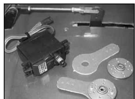
(below) You must use aluminium discs on the servos, especially if using the 8511/9611 servos, fixed to the C-ARF phenolic servo arms with at least 2 bolts each.
