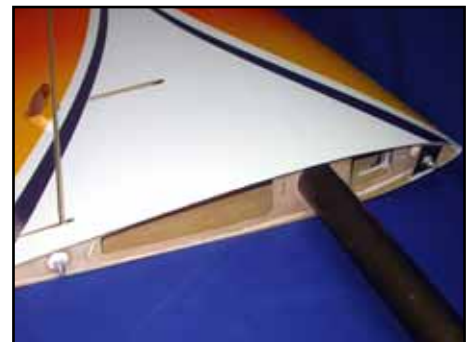
The internal structure of the new SuperXtra wing, before the carbon reinforcement & roving are added above & below the spar during the joining process.
