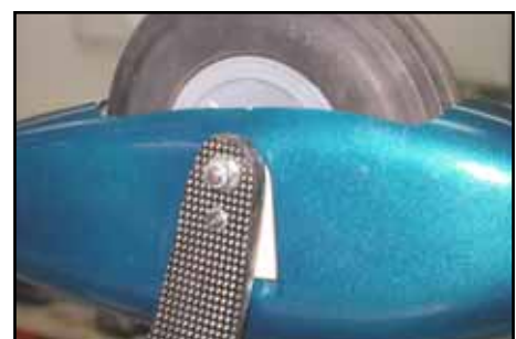
(below) View of leg showing M3 bolt and M6 axle bolt with locknut.
