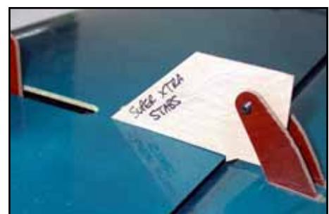
(below) Horn template for outer horns is made using the inner elevator horns for identical throws.
