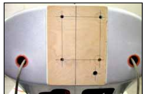
(above) Vertical centreline and the 1st hole to be drilled shown here. (below) The 4 holes for the motor mounting, and 1 for the linkage from the throttle servo.
