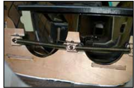
(above) View of the muffler mounting from the front, taken through the firewall.
