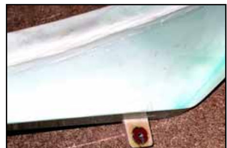
(above) The canopy frame is held onto the fuselage with 4 plywood tongues and M3 bolts/blind nuts. Notice canopy finally glued in with epoxy and microballoons mixture.
