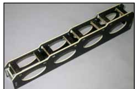
(above) Glue plywood doublers to the bottom of the servo rails. (below) The completed rudder servo tray is light and very stiff.
