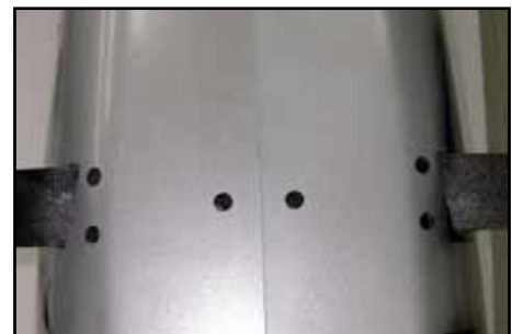
(above) The main legs are bolted in place through the bottom of the fuselage with 6 x M6 bolts.
