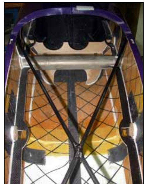
(below) The SuperXtra is 95% pre-fabricated, with all the main bulkheads, tuned-pipe supports, carbon bracing etc, installed at the factory. Below is a general view of the cockpit, muffler mounts and R/C gear area - as it is shipped.
