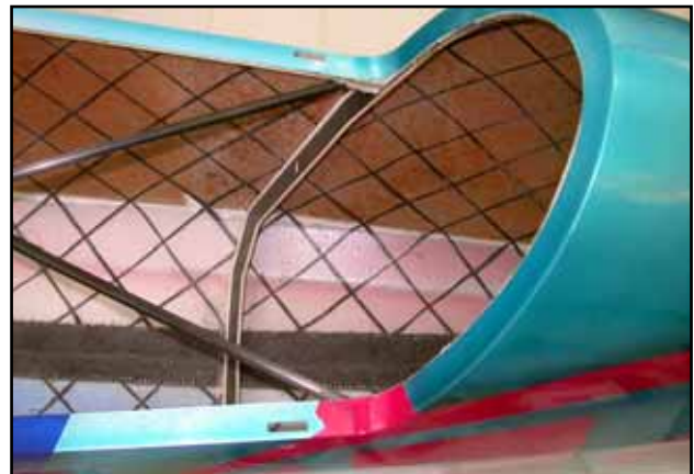
(above) The fuselage is manufactured using the 'Diagon-technique' with carbon tows to give exceptional torsional stiffness combined with extremely low weight.
