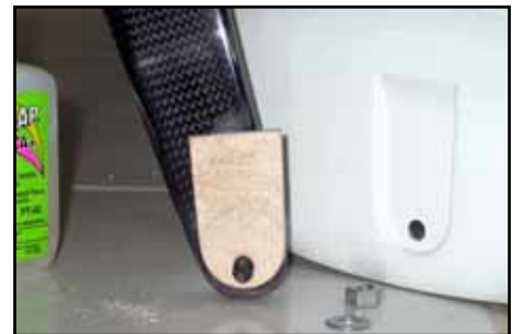
(above) Milled plywood part glued to carbon landing gear leg.
