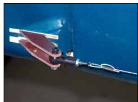
(below) Pass rudder cable thru' crimping tubes 2 times for safety.
