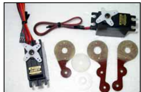
(below) The 3 phenolic servo arms, prepared before gluing and screwing in position.
