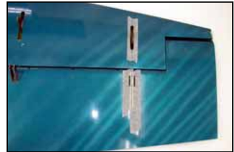
(above) Slots cut in elevator for outer dual control surface horns. (below) Add 1.5mm scrap ply to the bottom of the horn alignment template for correct positioning of outer elevator horns.
