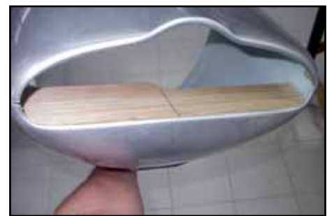
(above and below) A simple balsa sheet baffle will improve motor cooling considerably by making sure the air is directed through the cylinder cooling fins.
