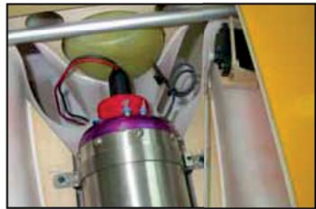
(above) This is an alternative position of Vector Thrust system servo.
