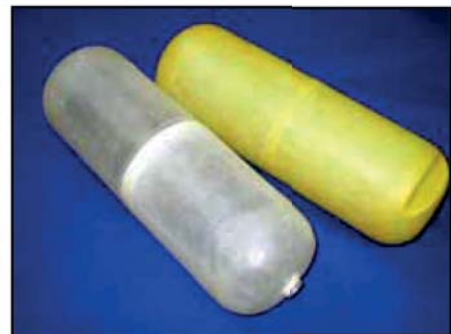
(above and below) The new kevlar and glassfibre tanks for the New Rookie, with capacities up to 3.2 litres, both have fuel baffles to prevent fuel surge.
