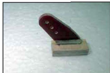
(above/below) Prepare the bottom of the phenolic horn as shown, and glue into the 2 slotted plywood parts securely.
