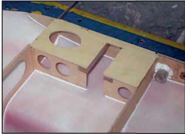
The plywood landing gear mount is now even stronger than the original Rookie, and is aligned with a jig in the mould before joining.
