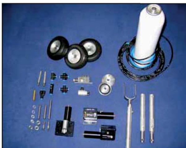
(above) The C-ARF landing gear set that is available as an option for the new Rookie.
