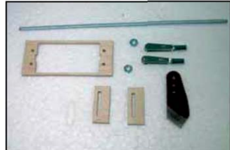
(above) The parts supplied for speedbrake linkage and servo mounting.
