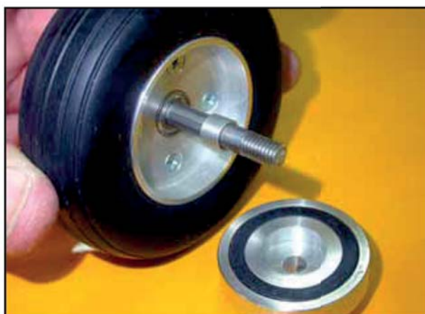
(above) Don't forget to install the short aluminium tubes between the wheel and brake drum.
