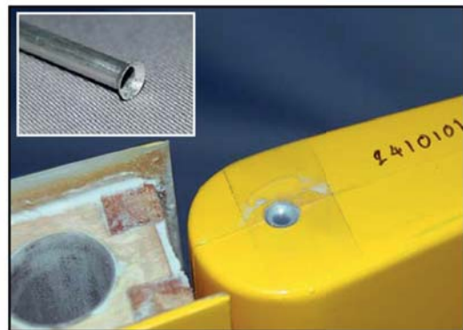
(above) Bell/splay one end of each tube, countersink the hole in the root end of the elevator, & use clear tape to fix the tube in position during final assembly.
