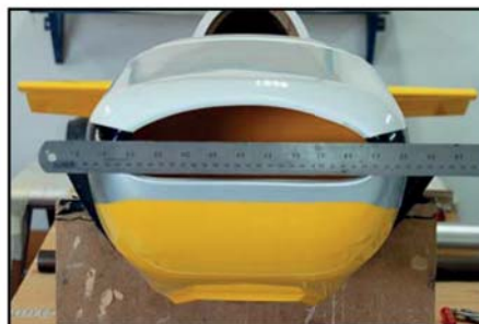
(above) Check cowl opening is parallel to stab or wing tube, and tape in position.
