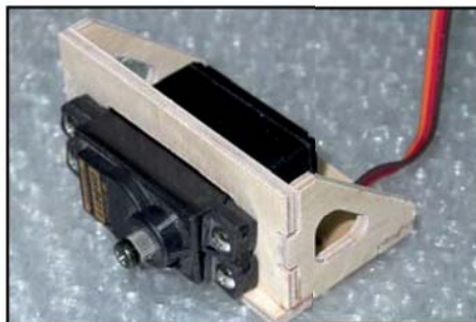
(above) Throttle servo mount assembled from milled plywood. (below) In the 3W set-up this was glued to the top of the fuselage
