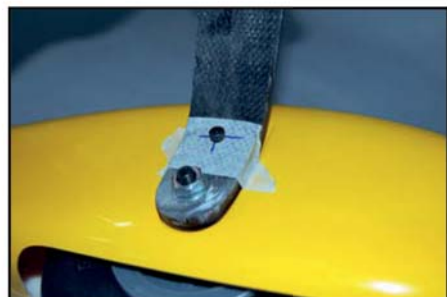
(above) The moulded dimple in the bottom of the carbon legs. Drill a central hole of 6mm diameter. (below) shows the M3 bolt thru' the carbon leg, into the T-nut glued inside the wheelpant.
