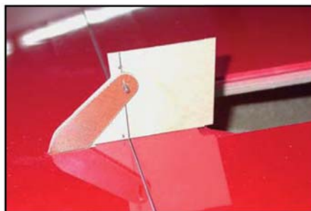
(above) The aileron horn template used to position the inner horns for gluing in place. The line is perpendicular to the hinge axis.
