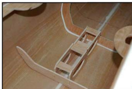
(above) Rudder tray and sub-bulk-head shown in the (optional) rearwards position.
