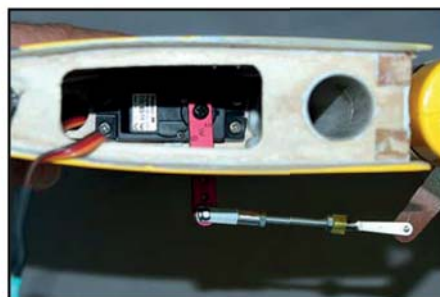
(above) Servo is screwed into the milled cutout in the inner rib.
