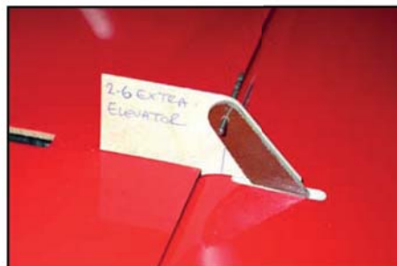
(above) Elevator horn alignment template from scrap plywood. Line is hinge tube axis. Use for both elevators to ensure same throws.
