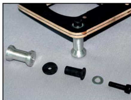
(above) Shows the order of assembly of the anti-vibration mounts in the carbon-ply mounting plate.
