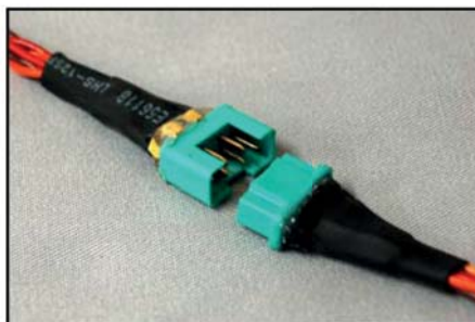
6-pin MPX connectors are used for extension leads, with one half mounted in the fuselage sides.
