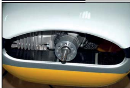
(above/below) Baffle installed in the cowl for the 3W motor.
