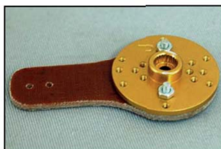
(above) If you use the phenolic servo arm extensions, you MUST bolt these to metal servo discs.
