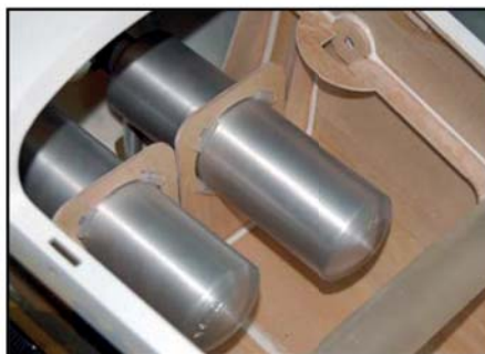
(above) Plenty of room to install a pair of MTW 75K cans in front of the wing tube, supported with the milled mounts supplied in the kit. (below) Typical cnc milled plywood canister/tuned pipe mount & hard silicone tubing included in the kit to suit \text{Ø} 49\text{mm} pipes, and both \text{Ø} 70\text{mm} & 80\text{mm} canisters.
