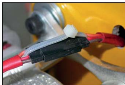
(below) Secure the connectors between the motor & ignition unit. (below) Fit barbs to all brass tubes and fuel connections for safety. Easily made from a paper-clip, soldered onto the brass tubes.
