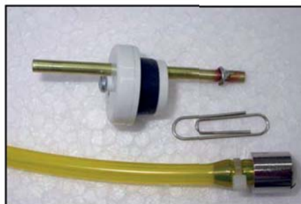
(below) Secure the connectors between the motor & ignition unit. (below) Fit barbs to all brass tubes and fuel connections for safety. Easily made from a paper-clip, soldered onto the brass tubes.
