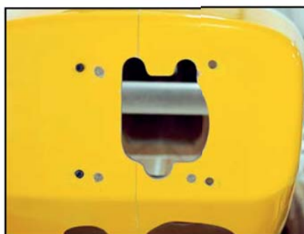
(above) Shows the cutout for the 3W carb, and also the holes from the DA-100 mount plugged with 6mm hardwood dowels.
