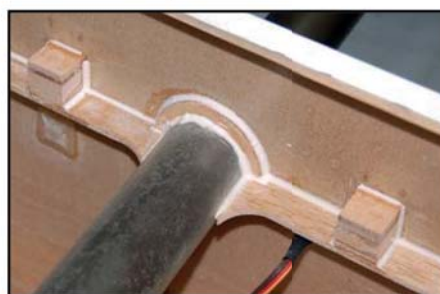
(bottom) Tank base is fixed to the blocks with 4 of the large sheet-metal screws, and washers.
