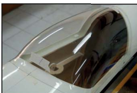
(above) Mark centrelines on the clear canopy at front and back and visually check that it is straight. (below) Duct-tape handles used to pull clear canopy against the canopy frame while gluing it in position with a few small drops of odorless-CA. Remove canopy and secure the edges of the clear canopy with a bead of epoxy to trap it in place (see above)
