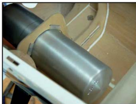
(above) A single 80mm Ø canister (TD110K shown) can be fitted - but you may need to use a cross-over header to get the correct length. (below) You can sand shallow notches in the forward landing gear mount, if necessary, for exhaust system clearance.
