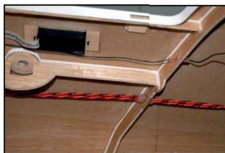
(above) PB Switch mounted in fuselage side, with ply reinforcement. Antenna wire and stab extension cables are routed thru' silicone protection sleeves and fixed securely.
