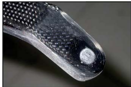
(above) The moulded dimple in the bottom of the carbon legs. Drill a central hole of 6mm diameter. (below) shows the M3 bolt thru' the carbon leg, into the T-nut glued inside the wheelpant.
