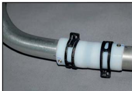
(above) Prevent the canisters or tuned pipe moving forwards or backwards with 2 small sheetmetal screws thru' the teflon coupler. (below) Rear pipe mount is secured with two M3 bolts and T-nuts to a 3mm thick plywood plate glued securely to the fuselage side behind the rear cockpit bulkhead. (only 1 T-nut shown here)
