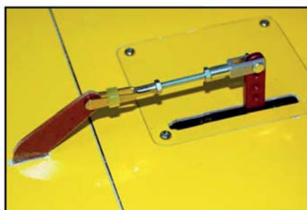
(below) Inner aileron horn. Clevis hole is 23mm from aileron surface.
