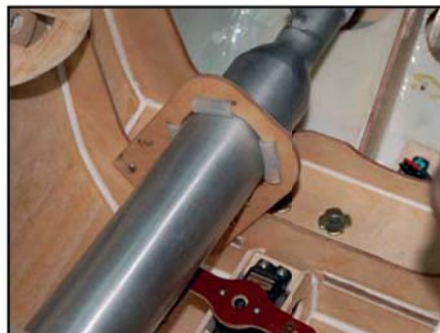
(above) Front pipe mount is screwed to back of LG mount.
