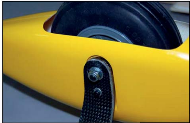
(above) Completed wheel pant. (below) Position of Ø 4.8mm hole for C-ARF optional tailwheel.
