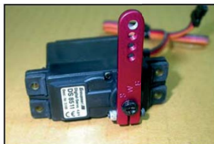
(below) The alternative is full metal servo arms, such as these SWB 'Double-Loc' types that we use on most of our factory planes.
