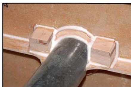
(above/below) Make 4 blocks from the balsa & plywood parts - and glue securely into position.
