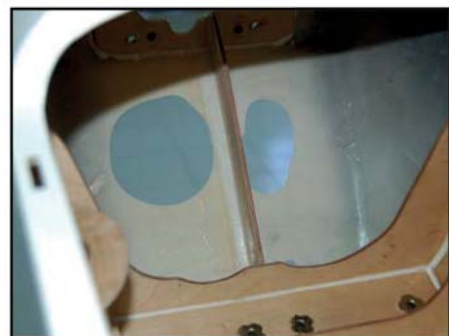
Glue the plywood brace securely between the firewall & LG mount. (below) The milled plywood firewall brace is supplied in the kit.
