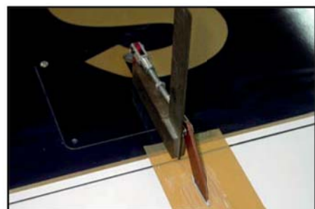
(below) Make sure control horns are perpendicular to aileron surface and parallel to servo arm.
