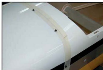
(below) Secure with 9 equally-spaced M3 x 12 bolts, into T-nuts glued inside the fuselage.
