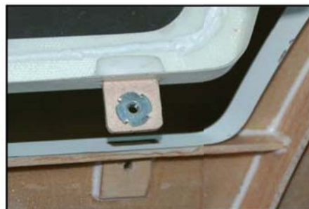
(above) The canopy frame is secured to the fuselage with 4 tabs, M4 bolts and T-nuts, all finished at the factory for you. Also note the bead of epoxy to secure the canopy to the inside of the fibreglass frame.
