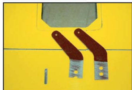
(above) Aileron horns must extend into the wing by at least 18mm (3/4"). Inner & outer horns shown.
