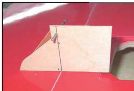
(below) Same template, with an extra hole drilled exactly 7mm higher, for installing outer horns.
