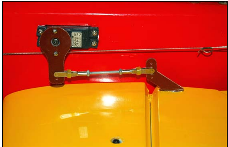
(above) Completed stab servo & linkage, also showing the position of the M3 stab securing bolt, recessed into the bottom of the stab. Note positions of clevises on the horns for the maximum mechanical advantage.
