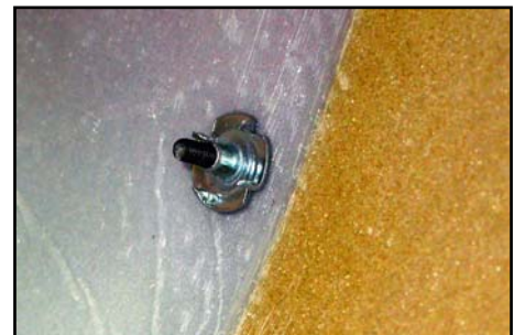
(above & below) Tack glue the T-nuts in position with a small drop of thick CA first. When cowling is correct, secure all the T-nuts with a drop of, fairly wet, epoxy and microballoons mixture as shown.
