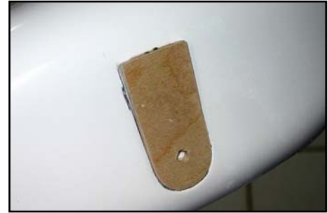
(above & below) Glue the milled plywood reinforcements to the inside & outside of the wheelpant as shown. The inside plate will have an M3 T-nut glued to it later.
