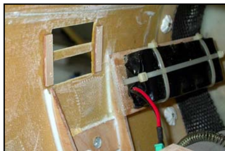
(below) Powerbox, Receiver and switch location in the Extra 300SX.
