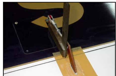
(below) View of aileron linkage, with servo using metal disc, C-ARF phenolic extension arm and the included hardware.
