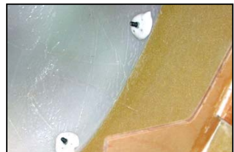
(above & below) Tack glue the T-nuts in position with a small drop of thick CA first. When cowling is correct, secure all the T-nuts with a drop of, fairly wet, epoxy and microballoons mixture as shown.
