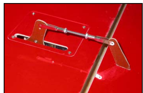
(below) View of aileron linkage, with servo using metal disc, C-ARF phenolic extension arm and the included hardware.
