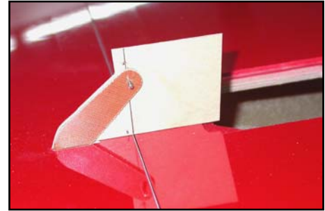
(above) The aileron horn template used to position the inner horns for gluing in place. The line is perpendicular to the hinge axis.
