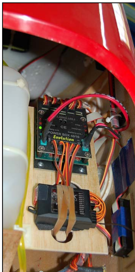
(below) Powerbox, Receiver and switch location in the Extra 300SX.
