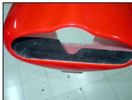
(above/below) 2 views of sample engine baffles; the top one for a DA-100 and the bottom for a 3W.
