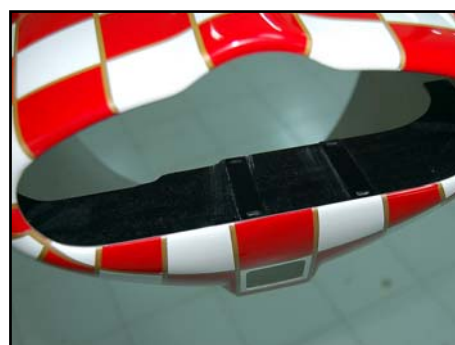
(above/below) 2 views of sample engine baffles; the top one for a DA-100 and the bottom for a 3W.
