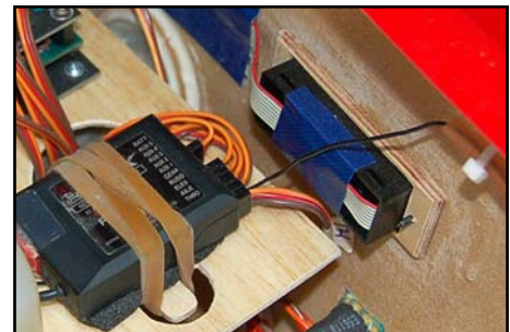
(above) 3mm plywood reinforcing plate glued inside the cutouts in the fuselage sides for switches.
