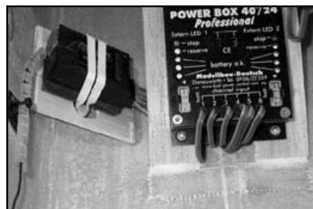
(above) The Powerbox can be screwed to the plate behind the rudder servos if using a DA-100.
