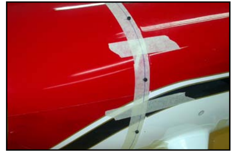
(above) Cowling is secured with nine M3 bolts, into T-nuts fitted in reverse, glued inside fuselage with a thick micro-balloons mixture.
