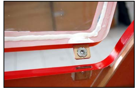
(above) The canopy frame is secured to the fuselage with 4 tabs, M4 bolts and T-nuts, all finished at the factory for you.
