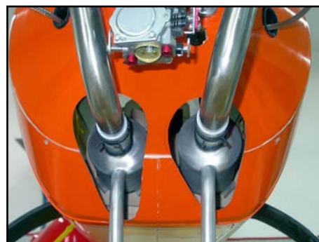
(above) Cut large enough holes to insert the cans through the motor-dome, taking note of the cooling requirements mentioned here.
