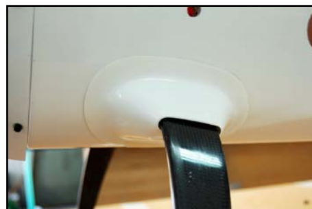
(above) Fibreglass leg Cuffs are secured to fuselage with a little clear silicone adhesive, allowing easy removal if necessary.
