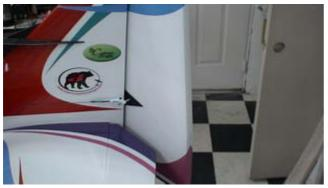
to mount a tail wheel, so drill through the bottom of the fuse into the hard point installed, to mount the tail wheel. The rudder however does not have a hard point; it will have to be added if you want a tiller arm attachment there.
