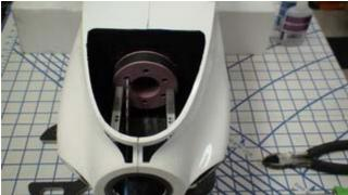
using an applicator or a brush, apply the glue to the firewall.
