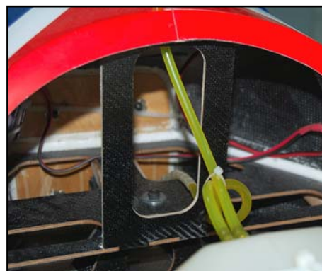
(above) Glue the landing gear upper support bulkhead in position with epoxy & micro-balloons after finally fixing the tank base into position.
