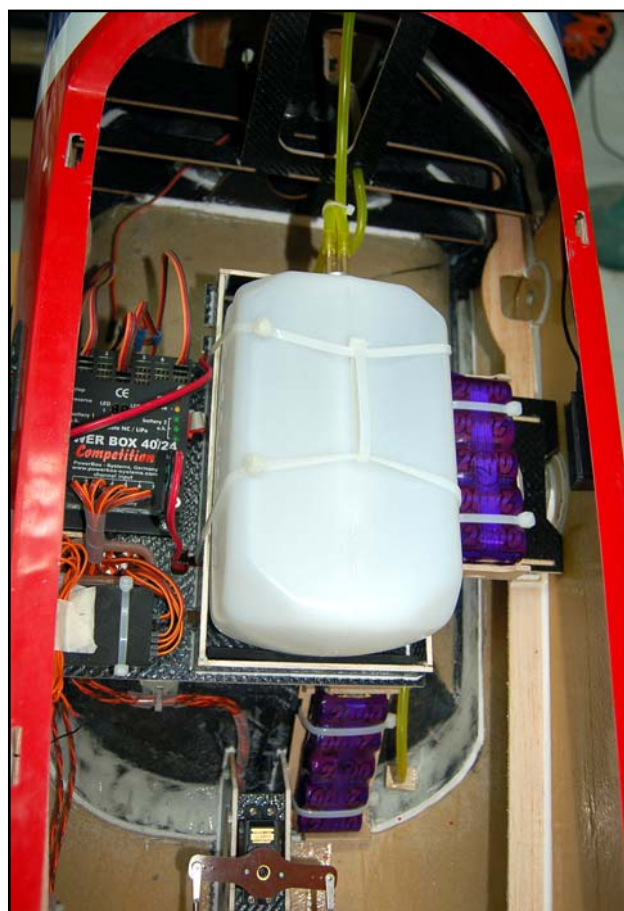
(above) A general view of the R/C installation, showing fuel tank base, Rx, Powerbox, and dual RX batteries. Ignition battery is located inside the motordome.
