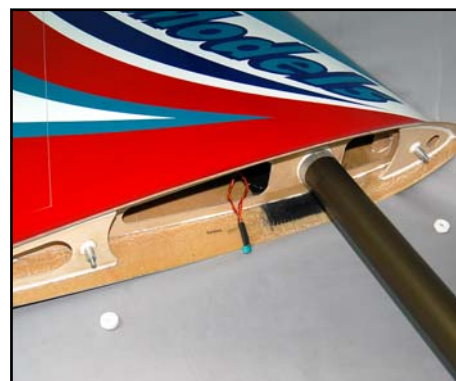
(below) The wing root, showing the 50mm Ø 6061 alloy wing tube and the aluminium anti-rotation dowels in the root rib.
