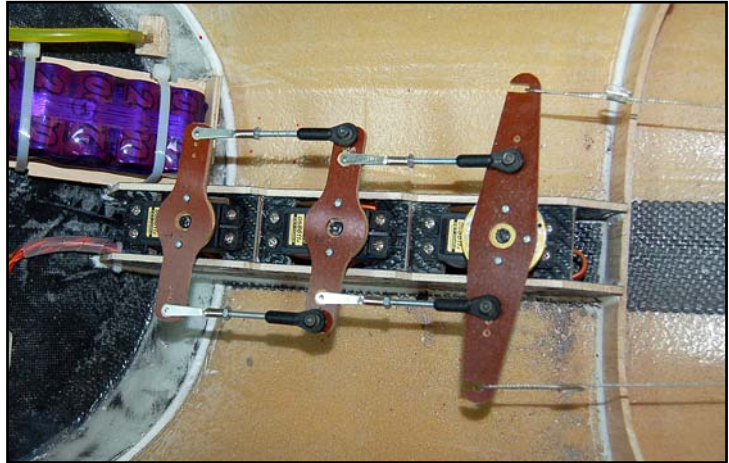
(above) Rudder servo tray glued into the fuselage between muffer compartment & rear cockpit bulkhead. (below) The slots for the cables are immediately in front of the rear bulkhead, 230mm from the back of the fin.
