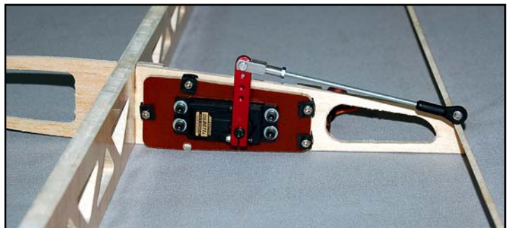
(below) Back view of the inner ganged servos, showing the lock-nuts that secure the servos, and the grommets and brass ferrules fitted around the perimeter of the mounting plate. Note that the 1.5" SWB arm has been sanded a little for a good fit of the clevis.
