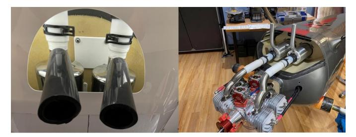
• If you are going to use stock mufflers please just install them to your engine and cut the two holes into the lower cowling
