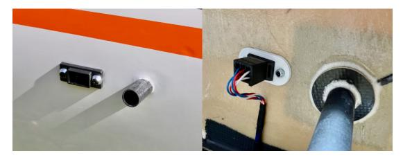
• As shown in the picture before you can use a Multiplex plug as well as other types of connectors for the wing (plugs, screws and washers not included)
