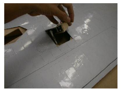
Take out the hatch and assemble the servo mount. The photo shows, which parts to use. Make sure that you glue the milled wood parts very well to the hatch cover. Use CA glue first, and then fill excessively with epoxy and milled fiber to get a strong bond. To sand the surfaces with a rough sandpaper is mandatory and not further mentioned in this instruction book.
