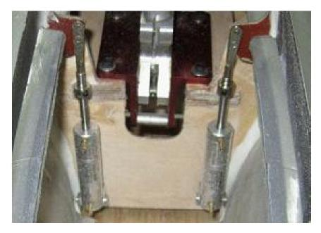
The gear door cypinders (we recommend Robart #165) are mounted to the front gear former. Determine the correct position of the mounting holes, and predrill these holes with a small drill bit.
