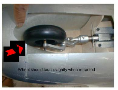
Check the movement of the gear carefully, check the angles and, especially, the fit of the wheel inside the air intake, when retracted.
