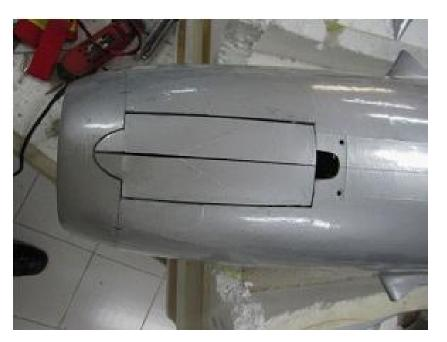
Finally, when the glue has set, move the gear doors and see if they lock anywhere. If so, sand carefully in this area, until they move
