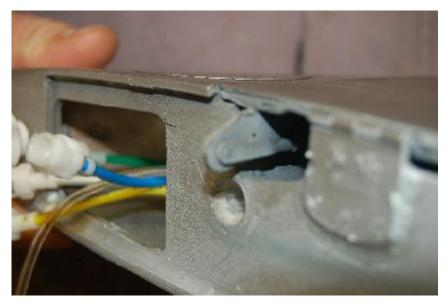
Note that the control horn sticks out of the root rip toward the fuselage when the gear door is closed. Make sure to gernerate enough clearance in the root rib and also you will have to grind a hole in the root rib on the fuselage to allow the control horn to stick in when the wing is mounted to the fuselage.
