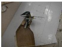
A slightly easier job is mounting the main gear door to the strut. The M3 threads are in already, and you now have to adjust the length of the brass tubes, which are used as spacers between strut and gear door.
