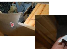
The nose hatch needs to be cut as shown in the rear to give the clearance for the pianopins that hold the center engine hatch.
