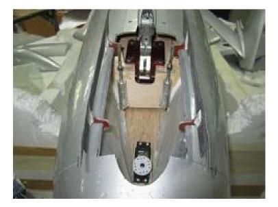
The front air intake duct and the nose gear formers are already pre-installed. The nose gear unit is preassembled already. Still you might better take off the strut, so that you can mount and handle everything easier. Fit the assembled nose gear unit into the fuselage. Mark the holes with a pencil.
