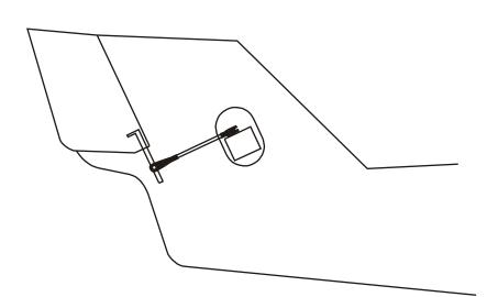
You will have to cut some areas of the rudder fin and the one-piece-stab to accept the rounded leading edge of the rudder. These cutouts could not be molded in for production reasons.
