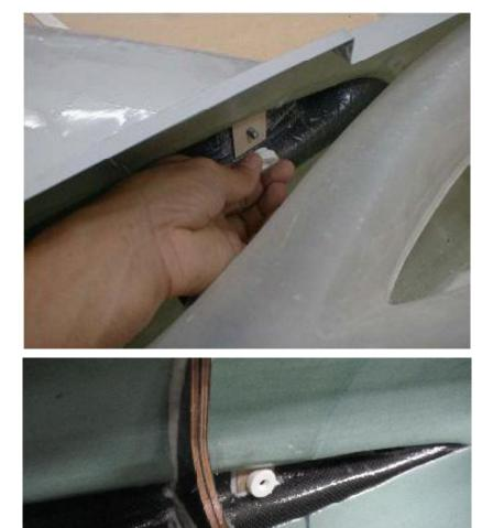
The wing rods are slighly different in length, the longer ones go in the front, the shorter ones in the back.
