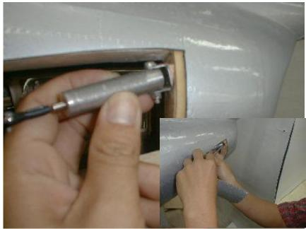
Now install the air cylinder for the speed brakes.
