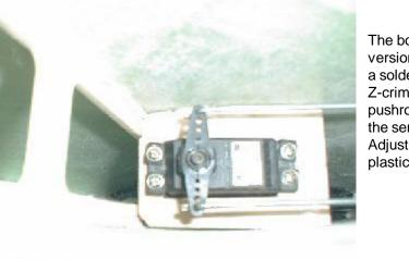
The bottom photo shows a version which does not call for a soldering iron... you can also Z-crimp the ends of the pushrods and connect them to the servo horn by this method. Adjustment is still given by the plastic ball links.
