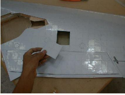
Your MiG-15's flaps are already precut and hinged with a special nylon elastic hinge. The flaps are stiff already, but will need some more rib and spar structure, especially to mount the scale inner surface plates. This gives a sophisticated scale impression on the plane on the ground, when the flaps are down.
