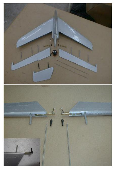
The elevator servos are hooked to a hidden torsion linkage, which does not interfere with any scale ambitions in regards to static judging. This torsion linkage is glued into the elevator controls.
