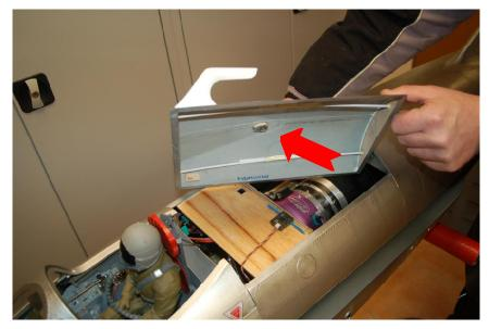
Therefor a blinde nut gets glued into the center hatch with a pice of scrap balsa or plywood.
