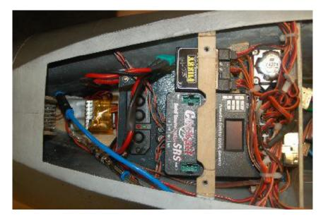
Here are some ideas, how to fit the electronic hardware into your plane. As this plane is not a beginners project, we must leave it up to you, to install all the components you are going to use. We gave you servo specs, recommended engines, fuel cells, and more, at different sections of this instruction manual already. At the end all is your decision, based on all your experience and preferences.
