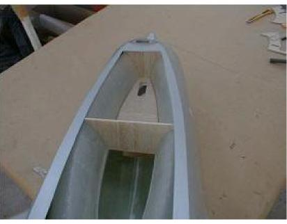
Glue in the radio compartment floor and the top part of the rear nose gear formaer which will complete your RC Box. The front former can be glued in now, but if you decide to do a landing light, leave it out for now.
