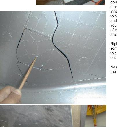
Cut out the styrene parts and sand the shape, so that they fit on the gear doors well. Glue them on with a few drops of CA glue.
