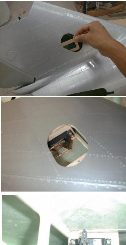
The rudder servo is mounted upside down in the rudder fin. Place the servo mount (3mm milled plywood) in the fin. Make sure that the rudder linkage can connect the torsion linkage of the rudder and the servo horn in a straight line and perpendicular to the rudders axis of rotation. This essential need gives you the right position for the servo mount.
