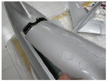
Start with fitting the rear hatch to the fuselage. Sand the rear end of the hatch and the fillet of the rudder fin so that everything fits nicely. Do not worry to sand off some material in the vertical frame areas, especially rounding corners, the fiberglass is thick enough in these areas.
