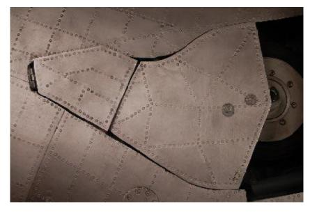
When you move the strut now in and out, you must check if the outer gear door hits and looks against the main gear door. If so, you will have to readjust the outer gear door again a very little bit, or move the main gear door down a little.
