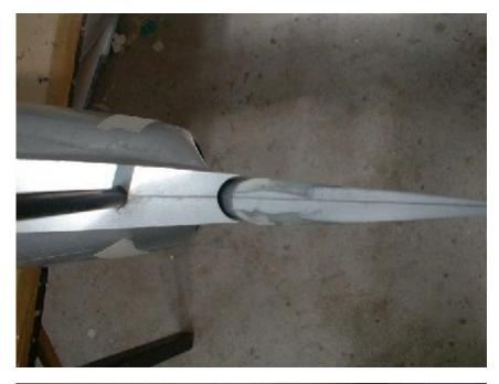
Now install the Robart hinges into the rudder. You have done this with the ailerons successfully, so go ahead and do the same thing with the rudder now.
