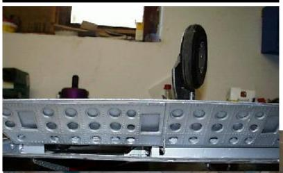
The bottom photoshows the intermal construction of your wings, so that you will get a better understanding where everything has to be placed. It shows the landing gear mount and the rib, where to place the aileron servo.
