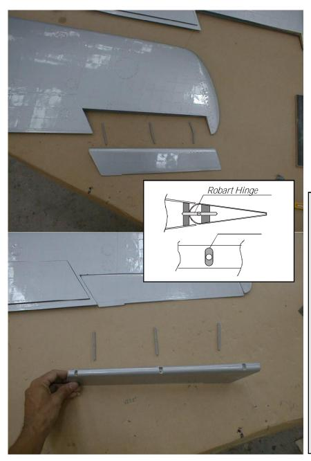
Installing the ailerons is an easy job, installing the servos is a little bit more delicate....
