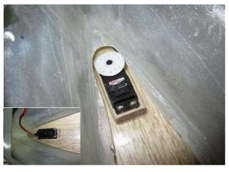
The nose gear steering servo gets mounted in the front edge corner of the nose gear compartment. The cutout in the former is already prepared.
