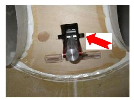
The cylinder of the retract unit will stick into the fuselage as shown. This gives easy access to the air nippels later.
