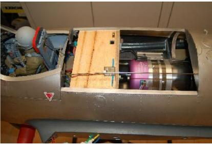
The center hatch which covers the engine is locked by two piano wires running all the way from the small hatch at the nose into the rear hatch which we permanently glued on in an earlier stage.
