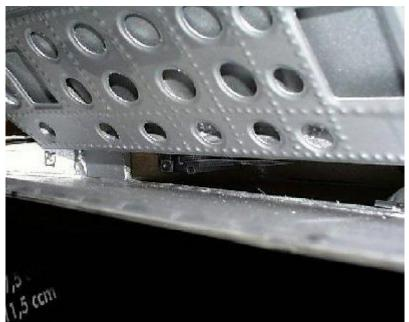
See the photos of a finished flap. If you install the vacuum formed sheet you should prepare it with the holes shown in the photos. The effect you get is 100% realistic. Us a few triangle balsa wood ribs to stiffen the vacuum formed sheet. But make sure that these ribs are placed in the areas between the holes.
