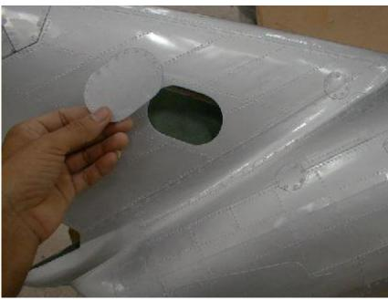
At that time you can install already the frame, to mount the hatch lateron. 2 scrap pieces of thin plywood do the job, just glued in on the top and bottom radius of the hand hole. Use 2 sheet metal screws, one each at the top and bottom radius to fix the hatch.
