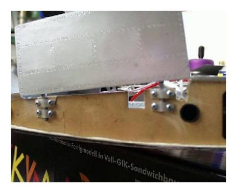
Now, we are installing the gear doors. The hinges are mounted to the outside of the root rib. Therefore the half round cutouts must be filled with plywood.
