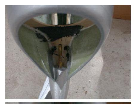
These photos show, where to cut or drill the holes for the linkage to pass the rudder post. These holes should be fairly large, so that the linkage does not bend ot lock at any position.
