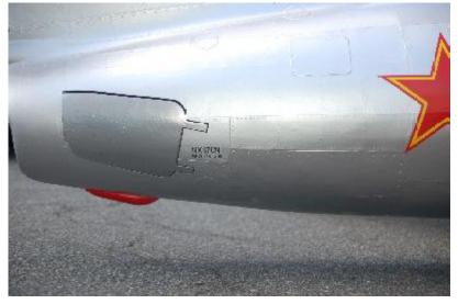
If you do not want to operate the speed brake doors in flight, you can skip this whole chapter 8. But a plane that scale should definitely have the speed brake doors working, and they are very efficient too.
