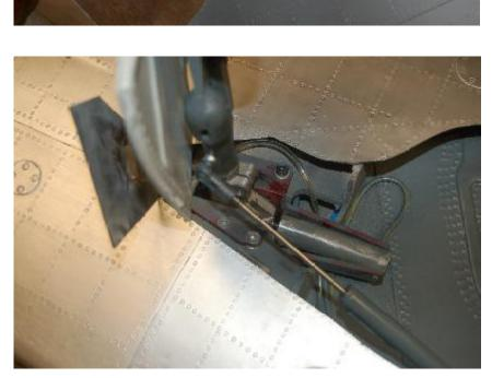
Before you finally drill the holes, assemble the gear with strut, wheels and brakes, and check how it fits in the gear wells. If necessary, you might have to grind the cutout in the mounting platform another few milimeters, and move the gear slightly more out.
