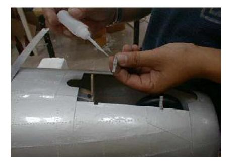
Be very careful with the CA glue on the hinges, as said before, it makes the plastic weak. Only apply glue to the hinge tips. The rest will be filled with epoxy, after the correct position is confirmed.
