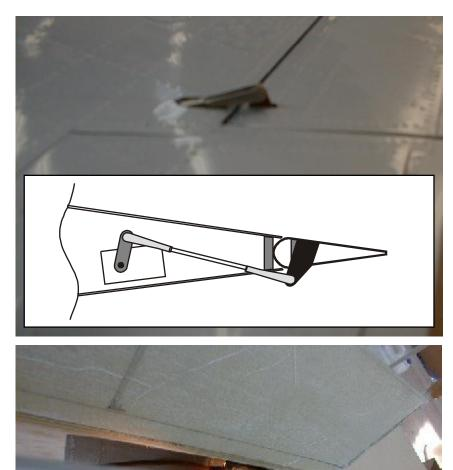
top side of the ailerons. Then glue in the control horn with 5 minute epoxy, so that the hole is approx. 6-8mm above the aileron surface (1/4 - 3/8th"). Make sure the horn is placed exactly perpendicular to the axis of rotation.
