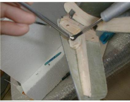
In general, the sloppier this mount is, the better it will work. Don't worry about clearance in this mount, as the cylinder also must move slightly up and down, not only in and out.
