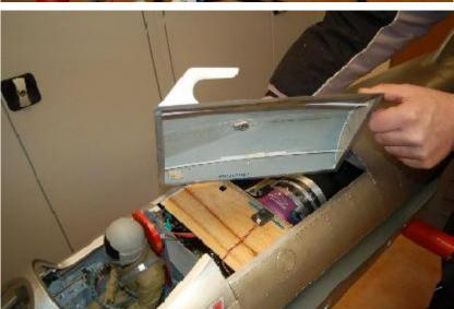
It is recomended to glue the plastic support rails to the hatches on various points for support. You do not need to glue them all the way through.
