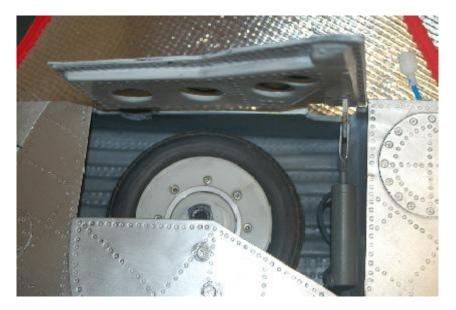
The cylinder is mounted to the front spar, just in top of the wing tube sleeve. the control horn is placed at the very front end of the gear door, so the root rib must be cut out in this area.
