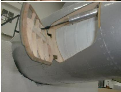
Further detailing is left up to you. We recommend at least cover the frame with the 0.8 mm plywood sheet.
