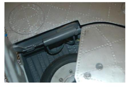
The Robart #165 cylinder is mounted with an M3 Screw to the plywood support wich gets glued to the spar in the correct position so completely open and close the gear door.
