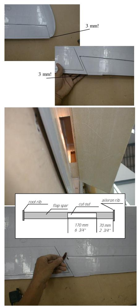
When you trial fit the ailerons to the wings please check on the photos left hand side. The trailing edge of the aileron steps back 3 mm from the wing tip, and the trailing edge then continues in one line to the trailing edge of the wing. The little trim tab on the aileron steps out of this line again about 3 mm.
