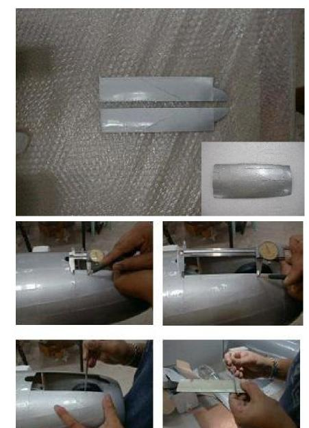
Mark the position of the hinges atboth gear doors and fuselage.
