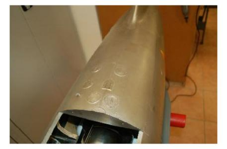
This rear hatch now gets glued on the fuselage permanently. Use 30-min Epoxy and milled fiber for the glue joint.
