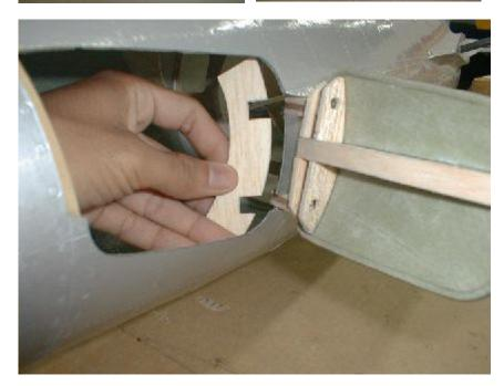
Next step is to frame the inside of the speedbrake doors. Milled balsa parts are supplied with the kit. Follow the photos to install these frames in the fuselage.
