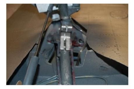
The support ar cylinder is not only a dummy for the characteristical scale look, it is s real active cylinder which is needed to safly opperate the landing gear as the strut and wheel are quite heavy for the smal sylinder of the retract unit itself.
