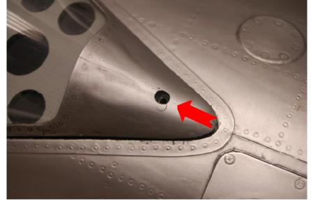
Cutting out the canopy works best with a very sharp X-Acto knife. The layup in this area is very thin, so be careful not to cut into the frames.
