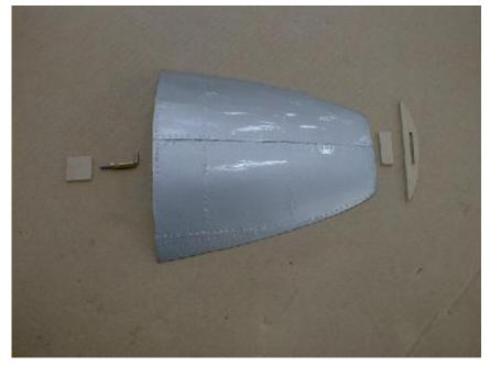
The nose hatch is a small challenge only. The 3 milled plywood parts have to be glued in place Also glue in the hatch latch. Make sure that the slot for the latch is long enough, so that you can release the hatch easily. The pin must disappear in the hole completely, when you pull it back.
