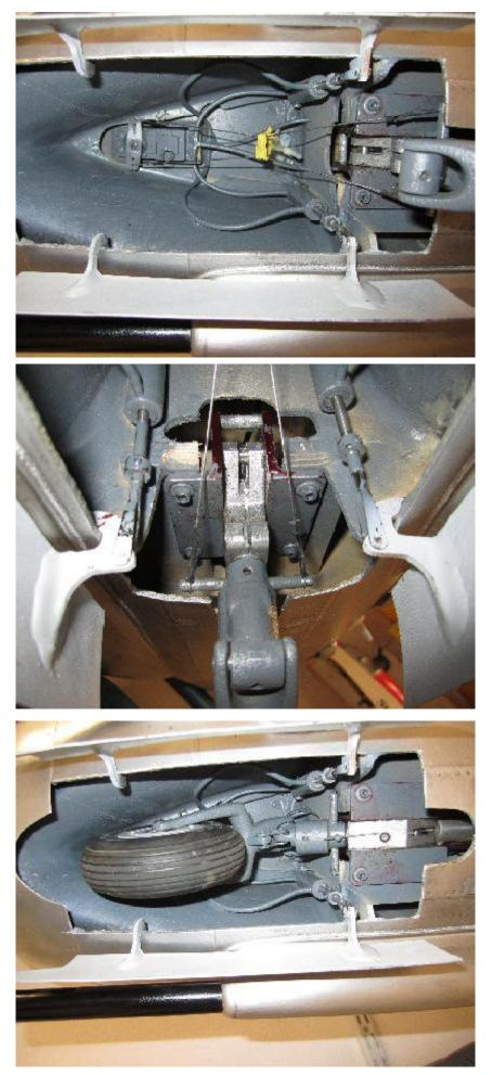
As the nosegear will get it's steering connection with two pull-pull wires, the servo will have to be mounted at an angle, therfore a plywould block of 9mm should be glued under the rear mounting as shown in the previous picture.
