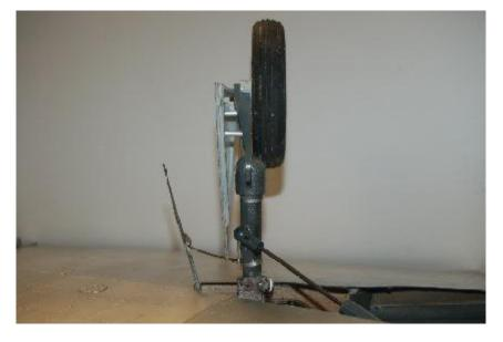
After it is confirmed that the gear fits the gear well, mark the position of the holes for the mounting screws with a pencil, and take the gear out.
