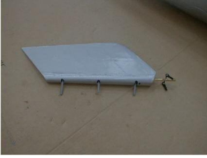
To recall, drill the holes with a 5 mm drill bit, open the holes in the fiberglass with a small round file to ret oval slots, and insert the hinges with epoxy glue. (Do NOT use CA glue!!!)
