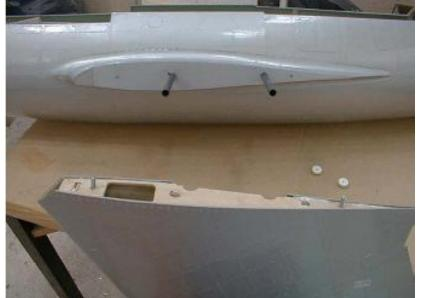
The wings are already allinged and the mounting is already installed in the factory.
