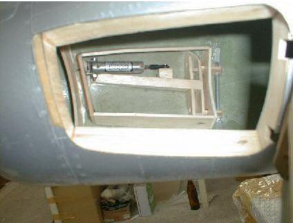
The speed brakes should open approx 45 deg. So you determine the fix point where to mount the ball of the ball link inside the door. Reinforce this area with another balsa block and mount the ball with a small sheet metal screws.
