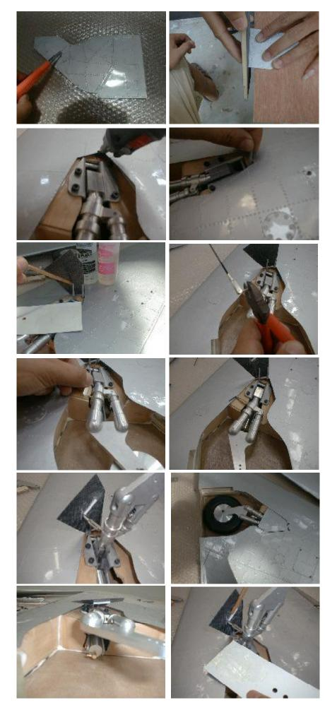
When the movement of the gear units is exactly as you want it to be, get started with the outer small gear door. The angles of this small gear door are very complicated as well. Basically, it is hinged with 2 Robart hinges, and connected to the strut by a 2mm rod, which has a clevis on on the strut side, and a 90 deg. bent angle on the door side, which slides into a plastic tube, which has to be glued to the door in the exactly right position and angle.
