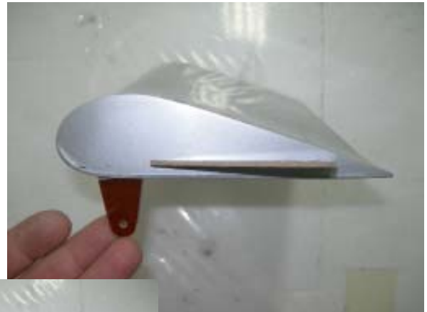
Inner flap: M3 bolt or all thread stud glued in.
