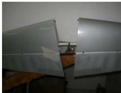
Make sure that the torsion linkage stays in during the whole joining process.
