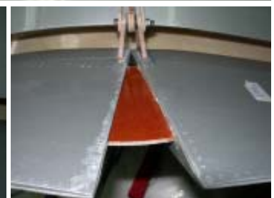
Allow flexing of flap hinges!
