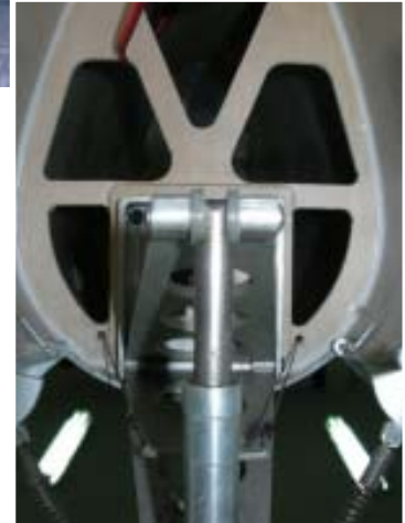
Here you see the springs mounted between the tail gear and the door control horns.
