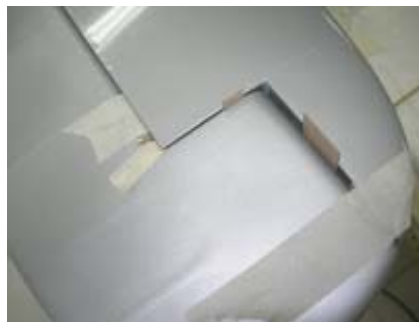
Use 0.8mm plywood as spacers between the edges of the counter balance surface of the elevator, to make sure nothing locks up. Make sure the root surface is matching the fillet with symmetrical gaps on both sides.
