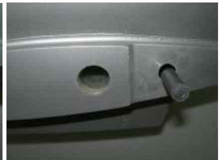
Center of torsion linkage is 38 mm behind rear edge of stab tube
