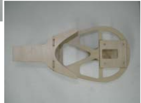
Assembled wooden framework for tailgear
