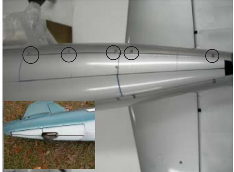
Slot the fuselage in the hinge area like on the main gear doors. 3 hinges for front door, 2 hinges for rear door.
