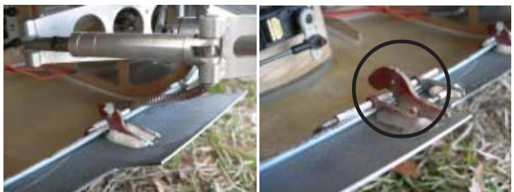
Close-locks for front and rear door and connection pin between both doors
