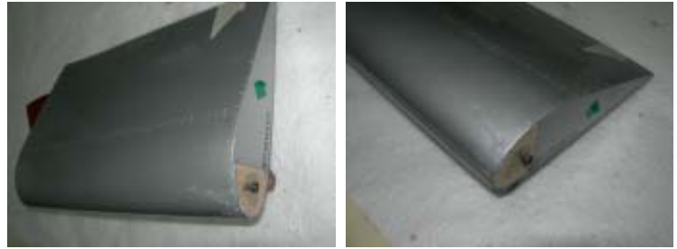
Inner flap: M3 bolt or all thread stud glued in.
