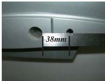
Center of torsion linkage is 38 mm behind rear edge of stab tube
