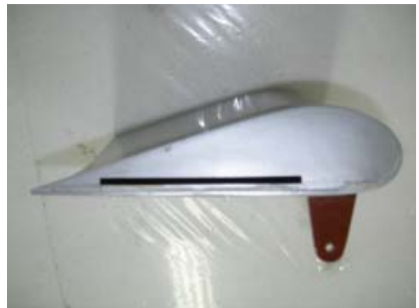
Middle flap: Slider glued into inner flap - middle flap slotted.
