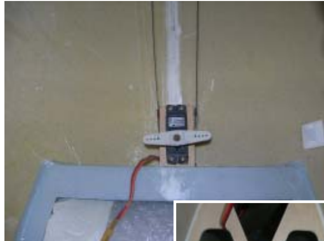
Position of tail gear steering servo and location for the pull/pull wires to the tail gear control horn.
