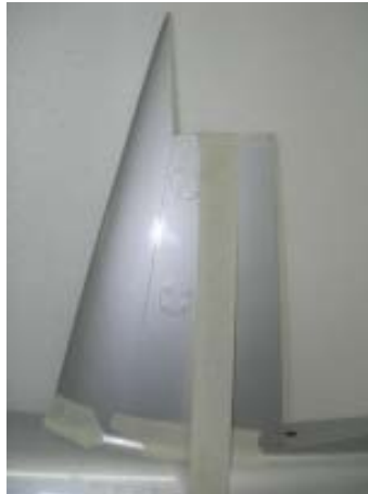
Process of gluing the rudder fin to the fuselage and installing the main fin spar.
