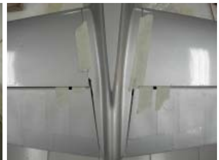
Use 0.8mm plywood as spacers between the edges of the counter balance surface of the elevator, to make sure nothing locks up. Make sure the root surface is matching the fillet with symmetrical gaps on both sides.
