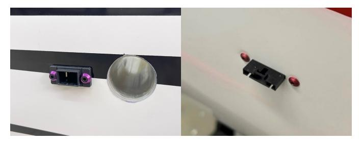
• As shown in the picture before you can use a Multiplex plug as well as other types of connectors for the wing (plugs, screws and washers not included)
