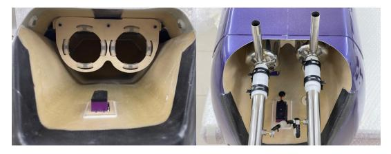
${\tt I}$  Installation of the KS 3086s canisters mounted at the rear end of the gear mount {\tt I}
