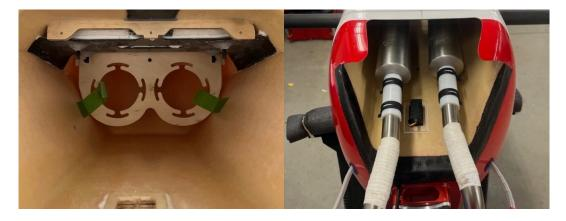
↓ Installation of stock mufflers ↓
