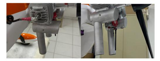
• If you want to install your ignition switch or smoke pump on the muffler compartment later you need to install some wood plates at youre prefered positions from the inside of the muffler compartment
