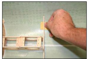
If you need to move the rudder tray forward to obtain the correct C of G, you will need to make 2 new mounting formers to use on the existing tray. Use 3mm ply for this.
