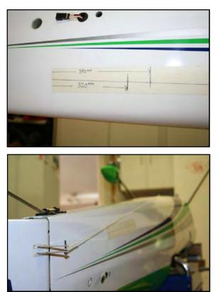
You can double check the exit measurement by running the string along the bottom of the fuselage. Flip the model upside down, and directly underneath the servo draw the servo arm measurements onto so masking tape. Remember this measurement is dependent on which servo arms you use.
