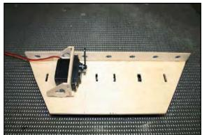
Once you have your ignition/battery tray assembled and trimmed to fit neatly inside the engine dome, tack it in place with CA and kicker.
