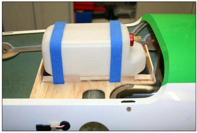
Run your fuel line to the engine taking care to ensure that it doesn't rub against the fibreglass or plywood structures. Where you run the fuel line is partially dependant on which engine you choose, and exhaust system fitted. Please view the pictures below for where the fuel and vent lines were run during our build. All of our fuel lines were held in place with self adhesive clips and where the line passed through the fuselage rubber grommets were used.
