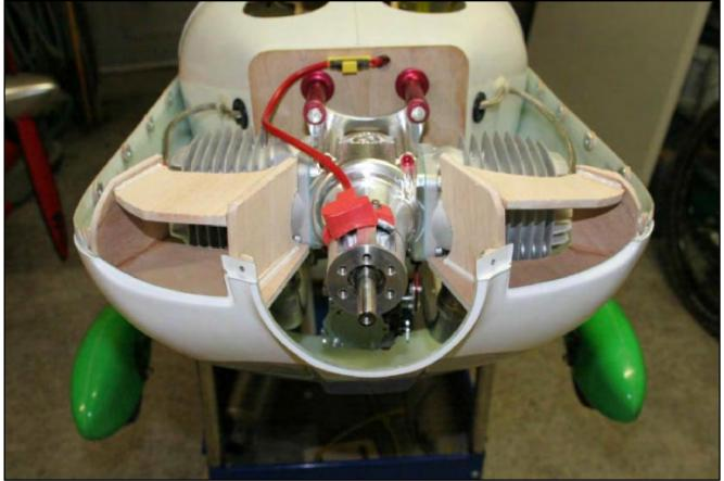
To ventilate the fuselage you will need to cut some cooling slots. The fuselage material is easy to cut out, using your Dremel. Finishing with a sanding drum will keep the process simple and tidy. Where you place the slots is again dependent on the final fit out and components used. But as you can see from the picture there is ample room for a sufficient number of ventilation slots.
