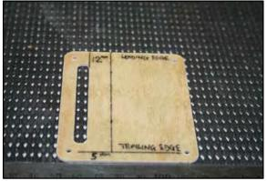
servo mount. Don't forget to give the surface of the hatch a light sand before applying the epoxy. Set aside and allow epoxy to set.
