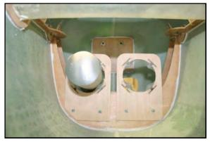
mounting plate. Keep in mind when drilling the mounting holes, not to drill into the carbon undercarriage legs! Place the mounts to suit your canisters, there is no need for definitive measurements here, whatever suits your needs! There is plenty of room to move them around to suit.
