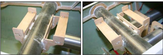
It's good practice to place some thin foam between the fuel tank and the tray. Ensure that any foam you use doesn't lift the tank too high as the tank may then hit the canopy frame. Fit the tank tray to the saddle using the 3mm cap head bolts. Secure the tank in place with the Velcro strap supplied.
