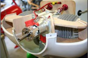
0.5mm ply. The balsa is easily shaped to your requirements and is also very light. The ply is added as the top layer when most of the shaping is done to add strength and a tough surface. Use some card to get the basic shape you require, and then trace the shape onto the balsa. The thin ply can be easily cut with scissors and the final shape trimmed with a sanding block. We used medium CA to glue the ply to the balsa.
