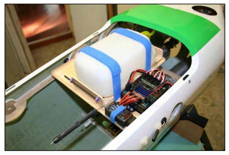
Clearly you can fit your RX batteries to the tank tray if you so desire. It is advisable to use the onboard components of the model to aid in achieving the desired C of G. Obviously you may elect to use ballast to obtain the correct C of G, but keep in mind a light model will perform better than a heavy model. Our suggestion is to work toward the lightest overall flying package and avoid adding ballast where possible.
