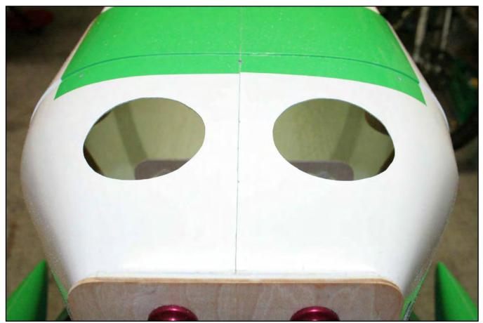
To aid in access to behind the engine dome, you can cut some access holes into the top of the dome. Please do not cut the seam line or the reinforcing join fibreglass band. Stay around 25mm either side of the seam line. The size of the access holes hole should be no greater than 80mm.
