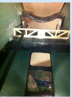
To attach the carbon linkage to the elevator use also the plastic ball link and M3 stop nut.
