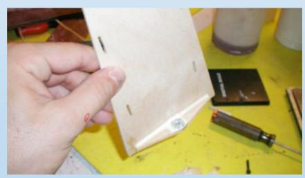
Then slide the front former on to the front tab of the battery floor, add some 30 min epoxy to the area which will contact the inside skin of the nose cone and place the tray in the right position, as seen on the photo. After the 30 min resin has cured, take the tray out and fill the bond with some more resin.
