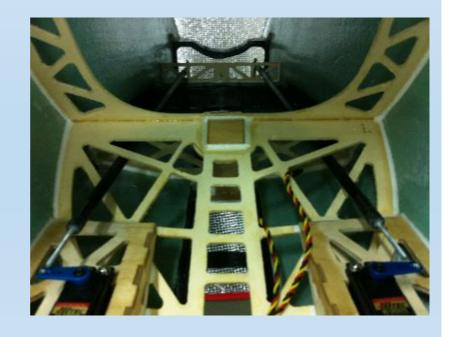
To attach the carbon linkage to the servo use the plastic ball link and the allen screw M3 x 16 and the stop nut.
