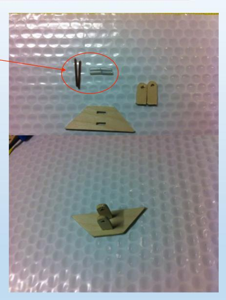
Use the 2mm steel wire as hinge wire for the front gear door and secure it with the Festo tubing as shown.
