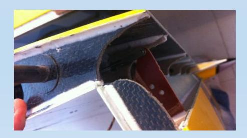
The landing gear should fit moothly into the gear mounts. Connect the airlines to the cylinder and slide it in the slot.
