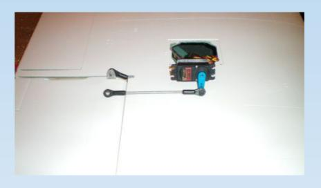
Please make sure your servo arm is mounted so that the servo centers perpendicular to the linkage, which connects servo and control horn on opposite sides (diagonally across the wing section). That way you almost do not need any slot in the wing surface. Then mount the servo with the 2.9 x 13 mm sheet metal screws into the ply rib.
