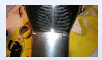
The tail fairing and thrust tube support on the rear end might need to be cut 4-8 mm but please check you trust tube in a trial assembly first. Sand the fiberglass tail fairing if necessary. The tube needs to slide easily over. If the fit is too tight, it will be difficult to take the rear part of the fuselage off and back on, in case you have to remove it for transport or maintenance.
