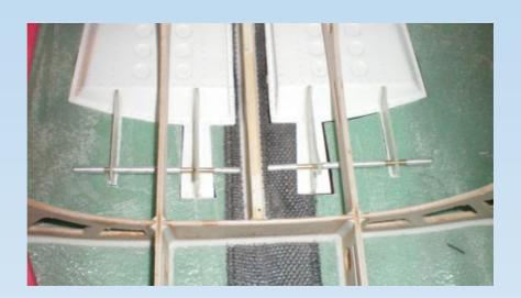
Then gue the aluminum tubes in with thickened 30 min epoxy or a 24hr resin and cotton flock.
