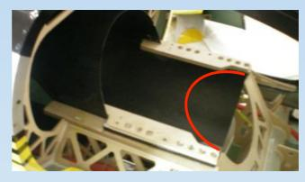
The trust tube, which is to be purchased separately, has already 4 holes drilled in the front edge ,you just have to slide it over the ducting. Sometimes you will have to sand the duct area a little down because there are manufacturing tolerances during spot welding process.
