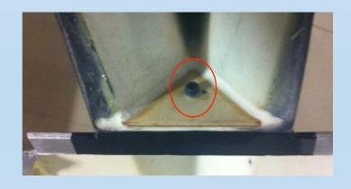
NOTE: You must protect the servo wire from rubbing against the fiberglass by using a rubber grommet!
