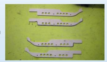
The two lower ones, which later ontact the duct surface, need to be rounded as you see here. Trial fit until they sit flat on the duct mount surface.
