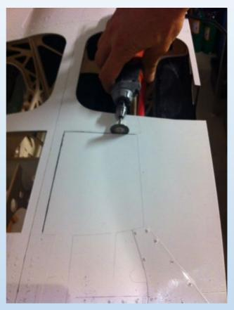
Sand around the edges, trial fit the speed brake doors and make sure they have enough clearance around.
