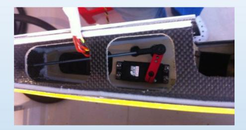
The flap horns are installed for you at the factory. You only need to install the servo and linkage. The length of the servo arm should be 1.5 in (35 mm). The linkage is made from an M3 x130 mm threaded rod.
