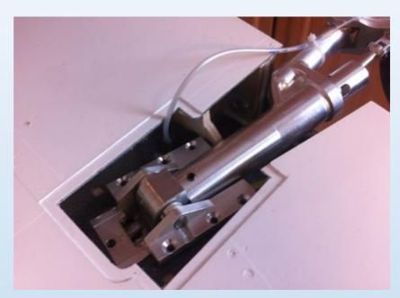
To screw the landing gear in place use 6x counter sunk sheet metal 3.5x 22 mm. It is recommend to drill holes into the wood rails with a 2mm drill before you inserting the screws.
