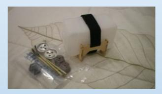
The main tank is very easily installed on to the milled wood former in front of the wing tube. A fiberglass pan is already part of the kit.
