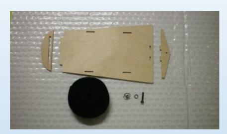
First glue the vertical former on to the battery floor and push the M3 T-nut in.
