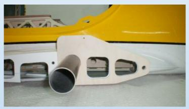
The center of gravity is quiet easy to check, just use the jig which we provide in our kit Check it with full hoper tank but empty main tank and extended landing gear.
