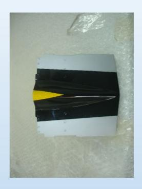
The tail cover gets connected to the fin with an M3 x 16 allen bolt and a 3mm washer.
