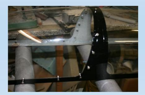
We provide in our kit a scale frame inlay. It will be very difficult to get it inside the canopy frame in one piece. So, simply cut it in two pieces and glue it in as shown on the photo.
