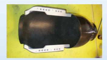
The duct is a standard part used on other CARF airplanes as well. This it needs to be adapted in length. The L-39's internal wood structure and the tight space from the intake to the engine, make it necessary to cut the ducting shorter, the estimated cut point is on the 4<sup>th</sup> hole in the wood support.
