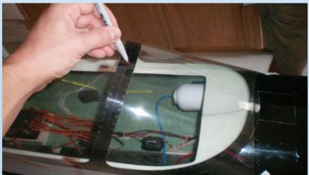
Cut now the front part around your mark. Use a pair of short, curved scissors or a diamond disk with a dremel. Make sure the room is warm, or warm up the material before you cut, to prevent splitting or cracking.
