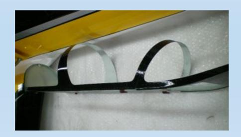
Roughly cut the front and rear of the canopy as molded, so that you can put it over the fuselage.
