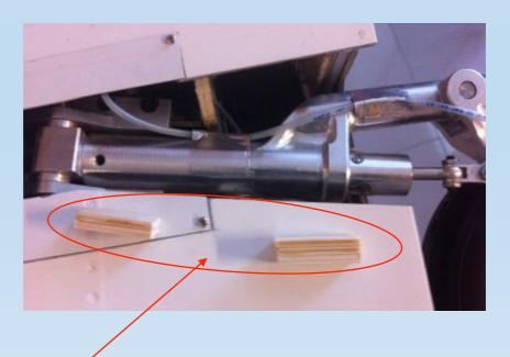
There are simple and more complicated ways to mount a fixed strut cover. We opted for the simple way and use wooden spacers between strut and gear door. We include plywood rectangles for that, use 2 layer on the outward point and 3 layer on the inward point.
