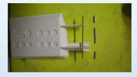
**Tip**: To align the speed brake doors perfectly with the surface of the fuselage, use some masking tape on the surfaces as shown, then use small balsa blocks 1.5 cm long and glue them on with a tiny point of CA glue.
