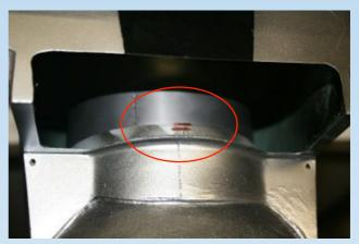
Secure the fairing during the curing process with tape.
