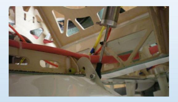
On gear door side you use the M3 aluminum ball link with the M2 x 15mm screw. To get the right opening angle of the door, pull on the ball link until the cylinder blocks. The gear door should be 90 degree open. Then glue the mount into the former, so that the gear door open position is always the end position of the cylinder. With the wheel collar you can now adjust the travel to close the door.
