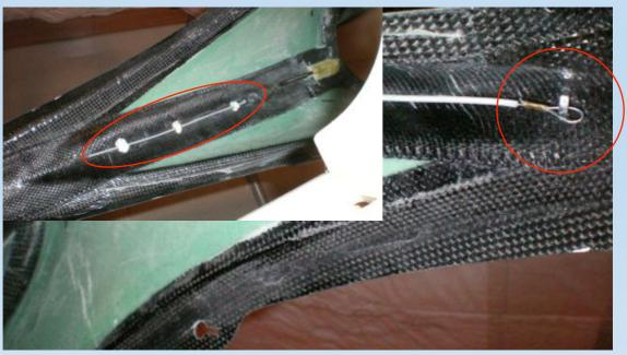
Use the white plastic sleeve to guide the steel wire. Cut the white tube approx 3 cm shorter than the steel wire, make a loop into the steel wire, (add an M3 nut in the loop) and place the end in an accessible place inside the fuselage. You must be able to reach it easily when one air intake is removed. Then glue the guide tube with 30 min epoxy on to the inner surface of the fuselage.
