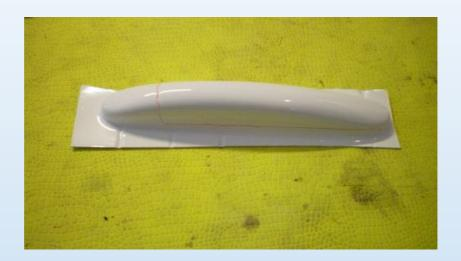
Cut the fairing as shown on the photos, make sure it will fit well to the fuselage and not foul the movement of the speed brake door. Then proceed with the gluing like the work steps taken when installing the flap fairings to the wing.
