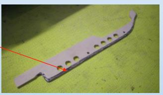
Roughen the gluing area and glue the wood parts with 30 min epoxy on the carbon ducting. Make sure they sit flush and are alligned to each other.
