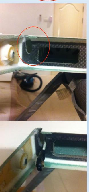
now you can close the servo hatch just drill 1.5mm holes and screw it with 4x 1.9 x 10mm sheet metal screws
