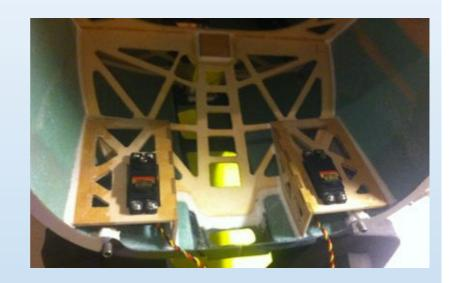
the carbon linkage to the elevator are finshed at the factory, just turn the ball links onto the threaded studs.
