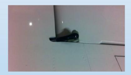
important on the one end of the aileron hinge brass tube you can see like a 90 degree bended 2 mm steel wire, here trough you have to secure the hinge tube with counter sunk sheet
