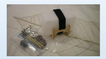
Use a very short 6mm festo tube for the clunk line. The clunk is placed in the cubic center of the hopper, it is not designed to move at all.
