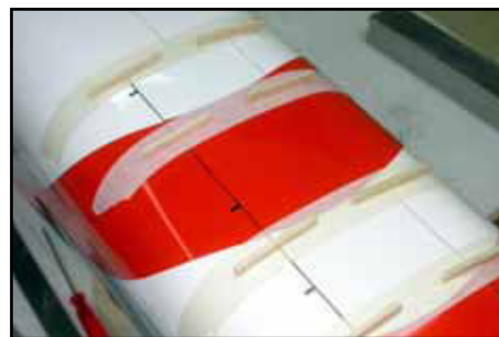
(above) Balsa sticks CA'ed onto tape to position door .
