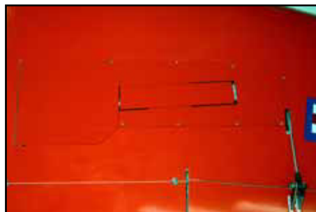
(below) Servo cover is fixed to ply tabs under wing skin with 8 sheet-metal screws (2.2 Ø x 10mm)
