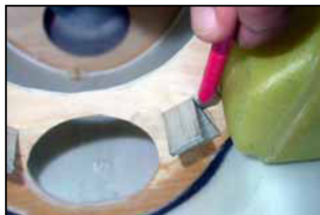
(above) Mark the final position of all 5 angles for later reference.
