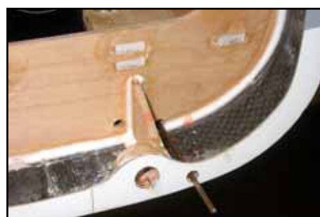
(below) Hinge wire is installed thru' a small hole in front fuselage flange and bulkheads.
