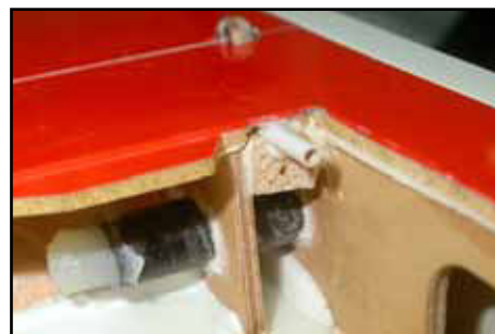
(below) Fit a hard balsa or ply support under back hinge tube.
