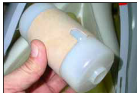
(above) Hopper tank located in plywood sleeve.
