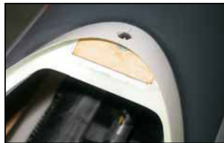
(above) The front of the canopy is secured with an M4 bolt, thru' a plywood plate into a T-nut in the fuselage - all factory finished!
