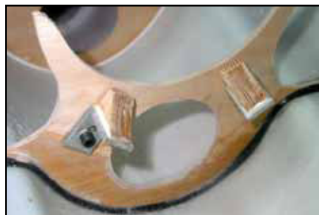
(above and below) Glue the shaped plywood blocks to the front angles with 30 minute epoxy and milled-fibre mixture as shown.
