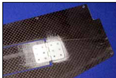
(above) Hinge glued to outer door and servo cover.
