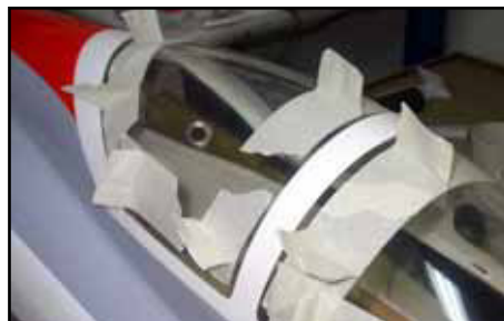
(above) Make plenty of tape 'handles' to hold the clear canopy in place while gluing into position.
