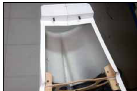
(above) The stabiliser is retained with two 6mmØ carbon pins at the back, and two M4 bolts at the front. All factory-finished.
