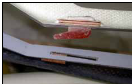
(below) The canopy frame is secured with 2 phenolic hooks into phenolic plates in the side-rails, and 2 location tabs.
