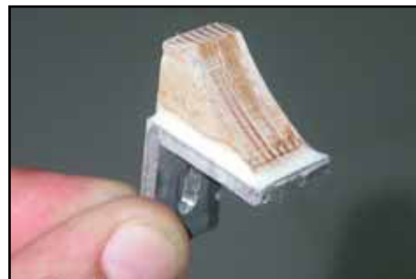
(above and below) Glue the shaped plywood blocks to the front angles with 30 minute epoxy and milled-fibre mixture as shown.
