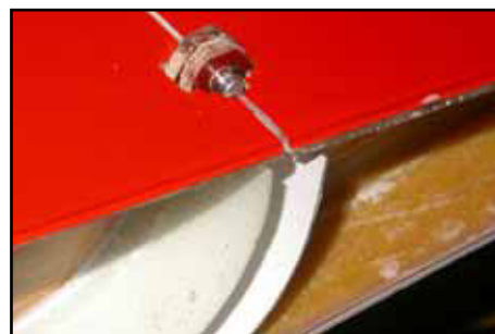
The centre of the hinge pin must be exactly on the hinge axis.
