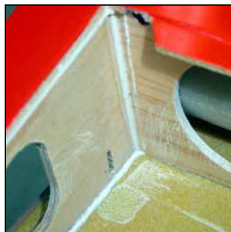
(above) Indentation and slot for door cylinder, and hole on back of balsa spar box for plastic tube.
