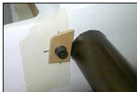
(below) Scrap ply and large washer under the bolt to pull T-nut into plywood inside the fuselage.
