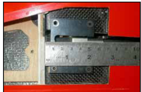
(above) C-ARF retract units are installed 5 - 6mm from the plywood rib outside the LG mount.
