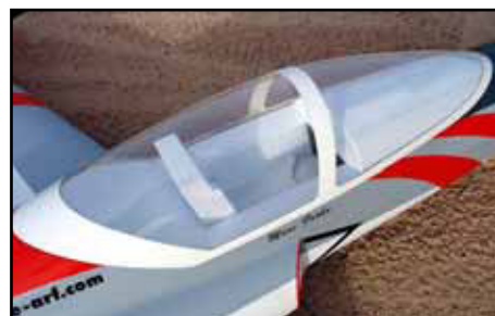
(above) Plastic cockpit tub dry-fitted into the cockpit. Add detailing and paint as required.
