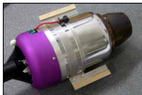
3mm ply packing on Jetcat P160 mount to centre it in bypass duct.
