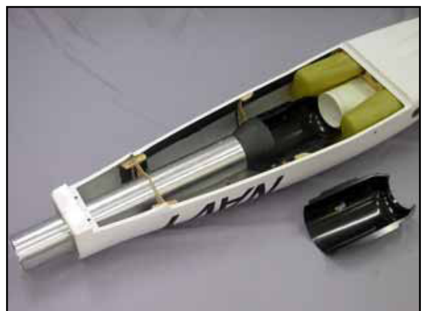
(right) A general view of the complete ducting system. The bypass, tanks and inlets are already installed for you - so is how the fuselage looks 5 minutes after you open the kit box !
