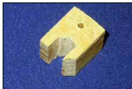
(above) Small block made from 3mm ply for the door cylinder.
