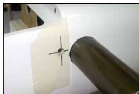
(above) 7.5mm Ø hole in fuselage for wing bolt T-nut, 13mm behind wing tube.
