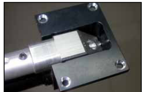
(above) Countersink the main retract mounting holes only. (below) 3mm ply packing strips.
