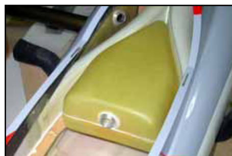
(above) The extra fuel tank can be installed above, or below, the plywood plate between the inlets.
