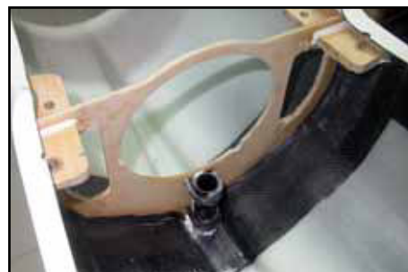
(above) The carbon tube spar must be glued fully into the fuselage tube, shown above. (below) Fin taped in place while gluing the carbon tube into the fibreglass tube in the fuselage
