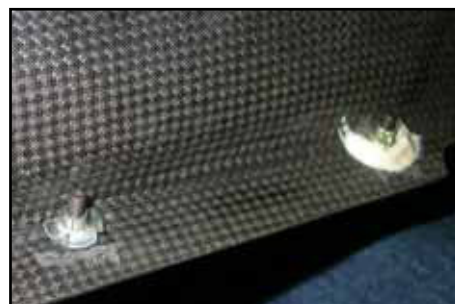
The T-nuts that secure the carbon cone to the bypass (above) and the engine mounting bolts (below) are glued on inverted, and then secured with a thick mixture of epoxy and micro-balloons.
