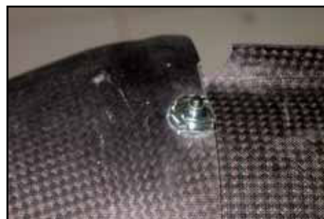
The T-nuts that secure the carbon cone to the bypass (above) and the engine mounting bolts (below) are glued on inverted, and then secured with a thick mixture of epoxy and micro-balloons.
