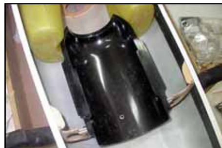
(above) The carbon bypass ducting is trimmed in the factory, and the 3 rear fixings for the upper half are already completed.
