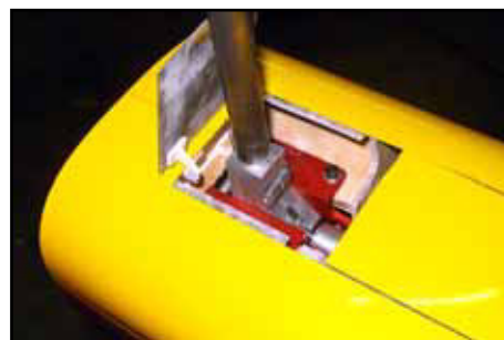
(above and below) A nice neat example of dual nose gear doors from Peter Agnew (Intairco), using offset door hinges.
