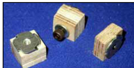
Laminate 3 blocks from the ply strip with thin CA, for exhaust mounting to the rear bulkhead.
