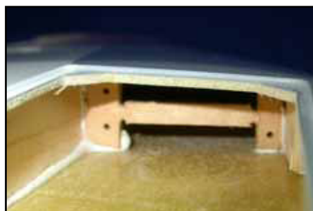
(below) Cut out the plywood bars across the servo holes, if not already done at the factory.
