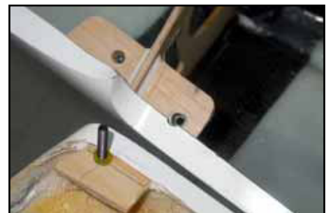
(above) Drill holes from the inside, fit the hatch and re-drill from outside to transfer holes to the ply plates in the fuselage. (below) Rear hatch fixing bolt & T-nuts. Also shows a Stab fixing plate and T-nuts, factory installed.
