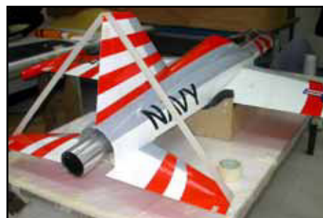
(above) The carbon tube spar must be glued fully into the fuselage tube, shown above. (below) Fin taped in place while gluing the carbon tube into the fibreglass tube in the fuselage
