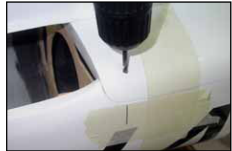
(above) Drill holes from the inside, fit the hatch and re-drill from outside to transfer holes to the ply plates in the fuselage. (below) Rear hatch fixing bolt & T-nuts. Also shows a Stab fixing plate and T-nuts, factory installed.
