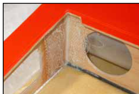
(above) Reinforce the joint between the back of the balsa spar box and root rib with fibreglass if not done at factory. Note the shape of the cutout in the wing skin for the inner gear door.
