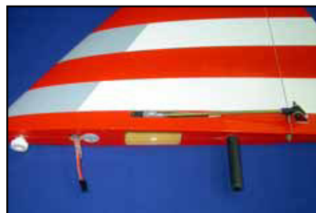
(above) Overview showing the plastic nut at the front and servo cable with spiral-wrap protection. (below) Plastic fairing shown glued over the rudder linkage.
