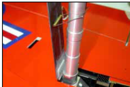
(below) A simple outer door connection - parts included in kit.
