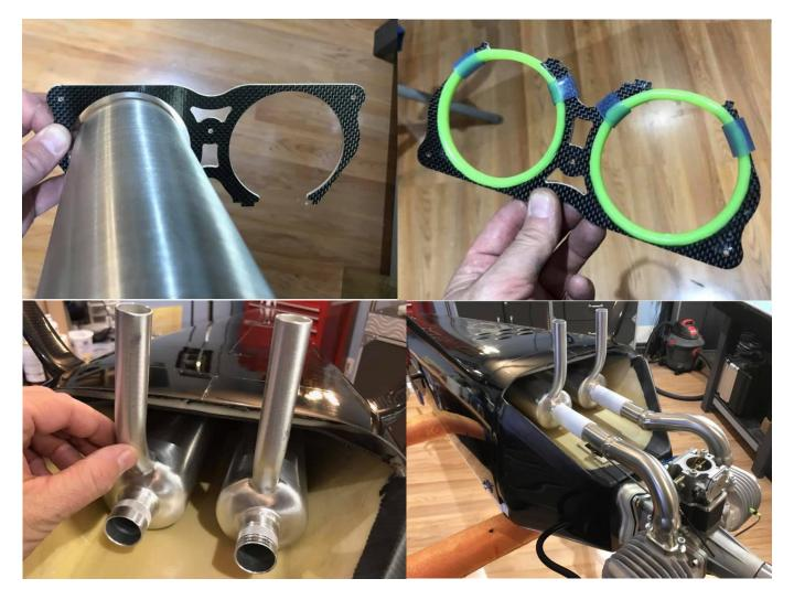
• If you are going to use stock mufflers please just install them to your engine and cut the two holes into the lower cowling
