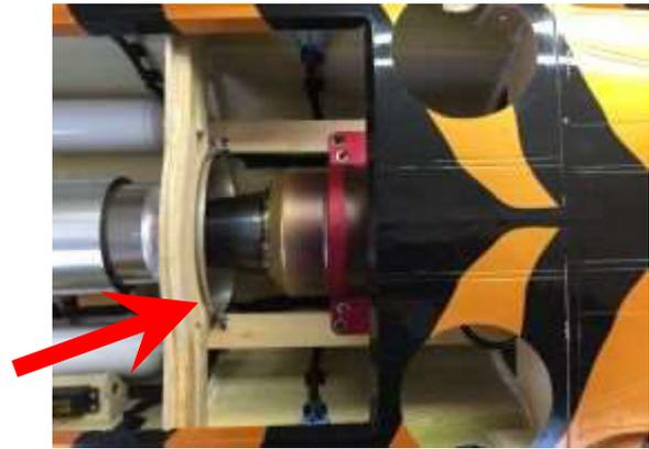
Depending on the engine type you might need 6mm spacers to center the engine in the thrust tube (JetCat's engine clamp is 6mm asymmetric, others are symmetrical).
