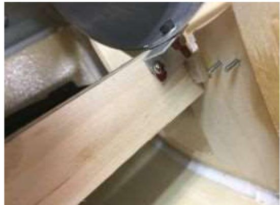
Mount the carbon entry cone with 2 aluminum brackets as shown in the photo. Please note: This is an important joint, use appropriate screws, make sure that nothing can come loose. If the tumble tube moves in the fuselage, the result can be catastrophic because there is a connection between the servos and the vector.
