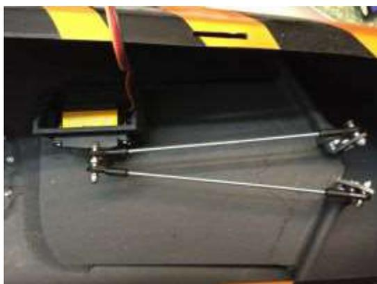
Use the panel line on the fuselage to adjust the neutral position of the canard.
