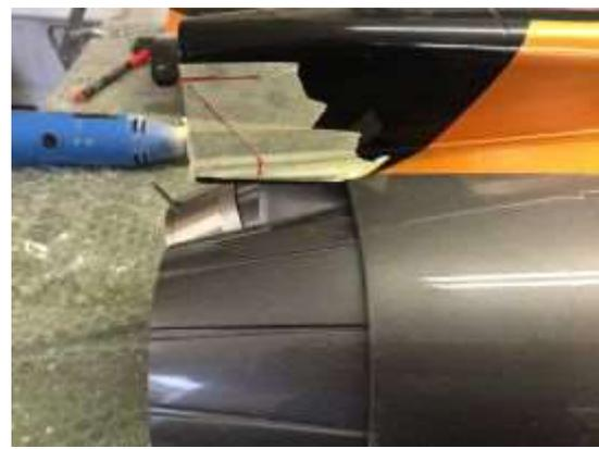
Cut 2 circular openings in the rear former to help to get the cooling air out of the fuselage.
