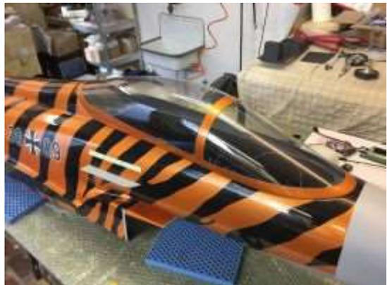
Paint the cockpit parts of and install the part with the pilot seat first, than the part behind.
