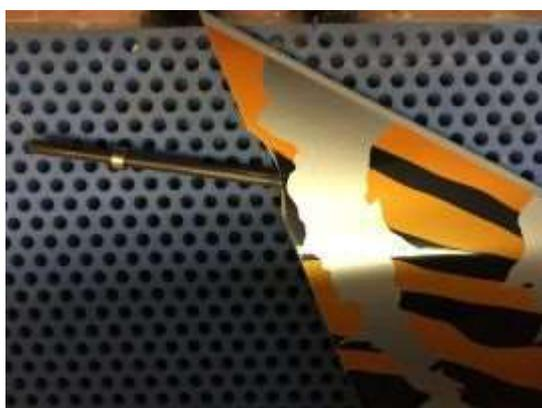
Mount the servo and the push rods as shown on the photo on the right. Attach the ball links to the aluminum control horn and clamp the control horn on the carbon axle.
