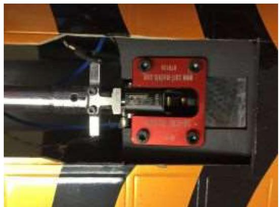
There are many options for nose gear steering, different gear types require different methods. Here it is shown an individual servo mount. A regular side mount is included in the kit, which can be used for the electron version.
