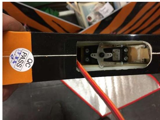
Then adjust the length of the threaded rods, solder the threaded ends on and install the linkages to the servo.
