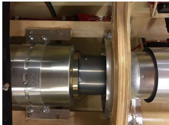
Additionally some scrap wood is needed to fill the gap in the connection between engine rails and rear former. The gap is so that the engine could be slid in from the rear during the assembly process. Once everything is installed, this slot must be filled.!!!
