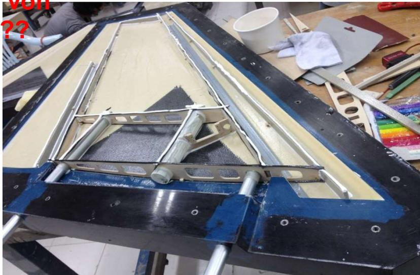
The fuselage and the wings are made of total area sandwich technology (TAVS) and are reinforced with carbon in the highly stressed areas. Carbon reinforced gear formers are installed and aligned.
