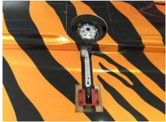
Grind a flat spot to the pin for the grab screws and fix the strut, secure the grab screws all with Loctite.
