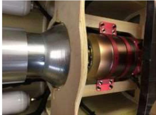
Always check the correct distance between nozzle of turbine and the beginning of thrust tube with your turbine manufacture.
