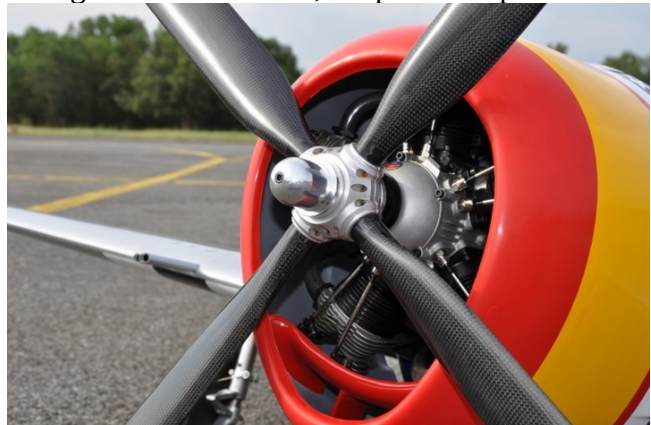
4 blade prop hub www.soloprops.com
