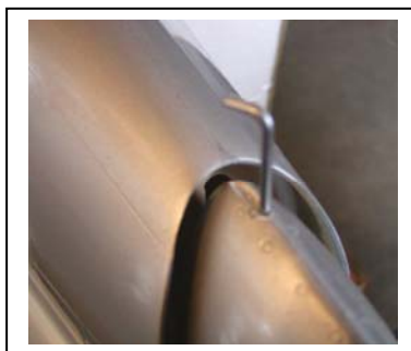
Rudder hinge pin is recessed into small slot
