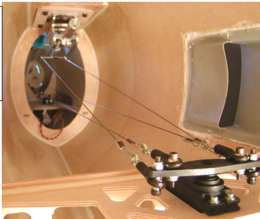
Rudder hinge pin is recessed into small slot
