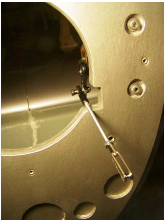
Throttle servo and pushrod installed
