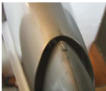
Rudder hinge pin is recessed into small slot
