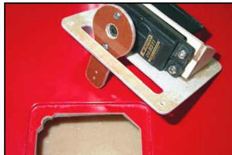
(above) Completed servo mount, with JR8511/8611 servo, also showing small radius needed in the wing for clearance of the mount.
