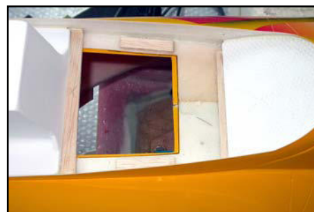
(above) Support the back of the main cockpit base with a small balsa stick.
