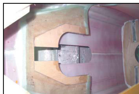
(above) The nosegear opening, and plywood mounting plates and fibreglass reinforcement are fitted in the factory.
