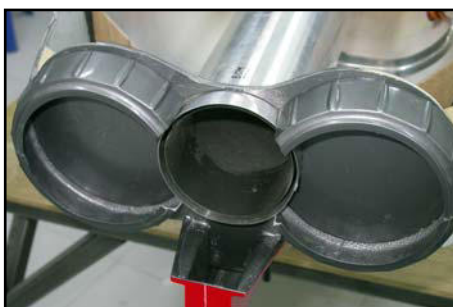
(above left) The dummy fibreglass exhaust nozzles are glued to the back bulkhead, with cut-outs to clear the thrust tube by about 2mm. Paint the rear bulkhead gunmetal or dark grey of your choice. Don't forget to drill a 25mm Ø hole in the centre of each dummy exhaust nozzle to prevent 'over-pressure' in the fuselage.
