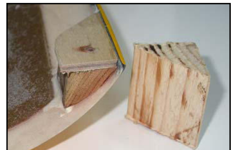
(above) Alternative method for reinforcing the plates in the hatch uses the supplied wood blocks.
