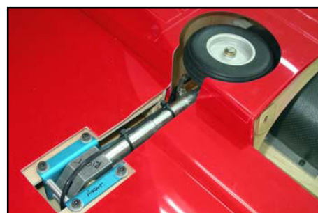
(above) Adjust the factory cut-outs in the fuselage to suit the scissor link on your oleo legs.
