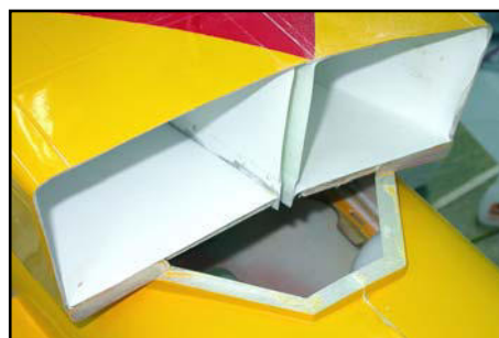
(above left) The dummy fibreglass exhaust nozzles are glued to the back bulkhead, with cut-outs to clear the thrust tube by about 2mm. Paint the rear bulkhead gunmetal or dark grey of your choice. Don't forget to drill a 25mm Ø hole in the centre of each dummy exhaust nozzle to prevent 'over-pressure' in the fuselage.
