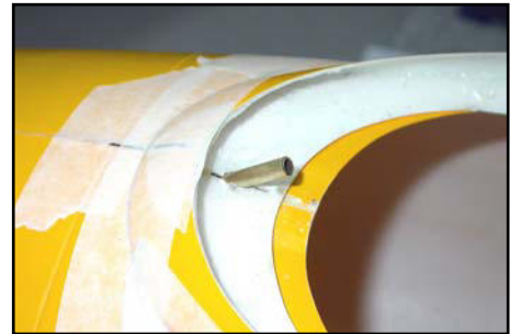
(above) The 35mm long brass tube (4mm Ø), secures the front of the canopy frame to the fuselage.
