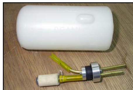
(above) Hopper tank made from a Sullivan R-10, with a felt clunk fixed to the feed tube in the 3-D centre of the tank.
