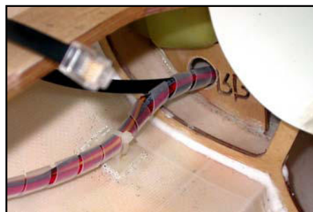
(above) Extension cables, retract tubes & turbine feeds protected in spiral-wrap, go through the milled holes in fuel tank bulkheads. Spiral-wrap is secured with a cable-tie onto a plastic mount.
