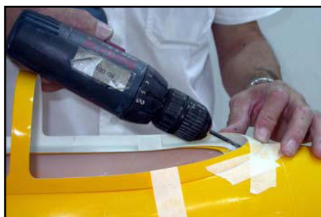
(below) Drill 4mm Ø through the front of the canopy frame and plywood part in the fuselage for the brass tube, at about 30 degrees angle.
