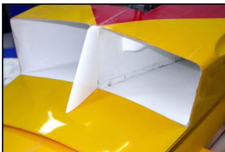
(below) The splitter plate between the inlets should be covered in glasscloth, sanded smooth and painted in your chosen colour.
