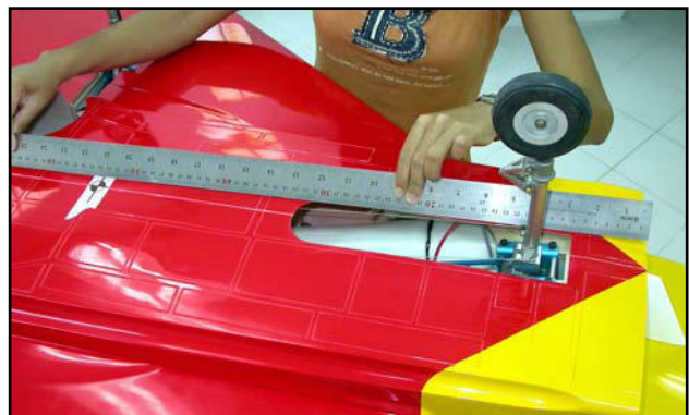
(above) Centre of Gravity for 1st flights is 540mm back from the front of the inlets, with empty main fuel tanks.
