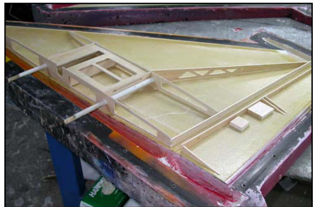
(above) The 'New EuroSport' wing structure in the mould before the wing halves are joined. The landing gear mount, support structure and root ribs are now completely constructed from high-quality plywood for extra strength.
