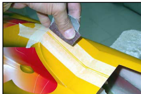
(above) Sand any raised seams for a flush fit of the canopy frame.
