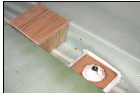
(above) 3mm balsa bridge made from milled parts supplied to cover the underside of the rudder extension cable socket.
