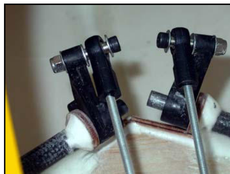
(below) View of the moulded carbon canard arms with linkages connected. Please fit one plastic washer between the Canard arm and the plywood 'P' plate. You may need to file a small slot under the each canard arm for clearance of the M3 locknuts on full 'down'.
