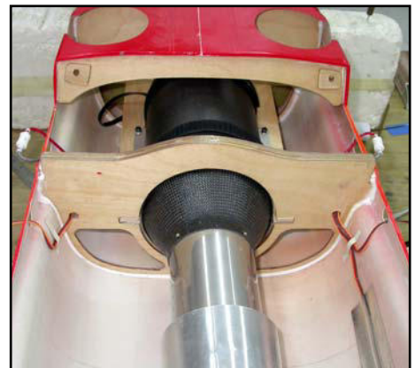
(below) View of the complete full-flow system, showing clean and simple installation.
