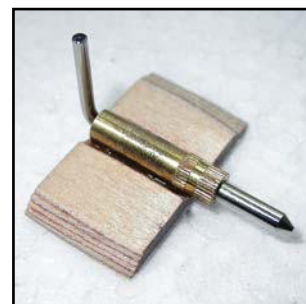
(above) The Hatch latch is glued to a plywood plate, and then into the fuselage with an epoxy/micro-balloons mixture. Use tape to secure until glue has dried.
