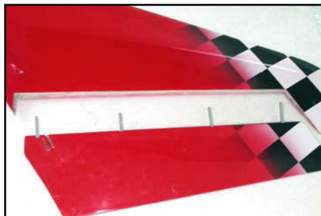
(above) 4 Robart pin hinges secure the Rudder to the Fin.
