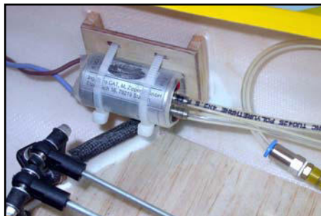
(below) We recommend installing the fuel pump in a position where it is easily accessible, but at least 15cms from the ECU and receiver.
