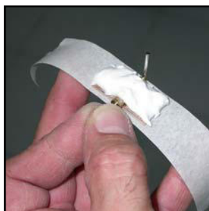
(above) The Hatch latch is glued to a plywood plate, and then into the fuselage with an epoxy/micro-balloons mixture. Use tape to secure until glue has dried.
