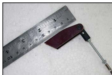
(below) Cut the large phenolic elevon horns as shown, about 55mm long, with a 30° angle on the bottom ends.
