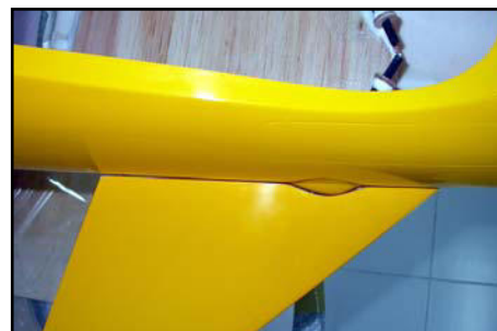
(above) The canard root should be about 1mm from the fuselage side.
