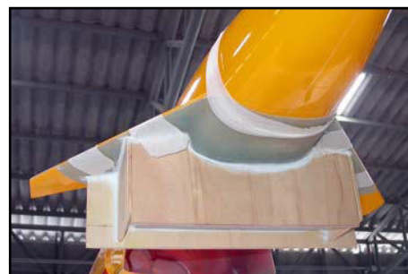
The canard shafts and tubes are carefully aligned and installed for you at the factory, using a specially moulded jig for accuracy.
