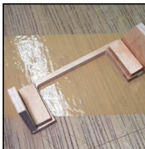
(below) Spare plywood can be used as doubler on back of mounts. Sand CA glue joints before securing with slow epoxy/milled-fibre mix.
