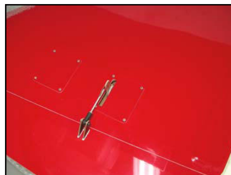
A single high-torque digital servo like the JR8511/8611 is more than enough for each elevon, but a second servo bay is moulded-in to allow dual servos if required.
