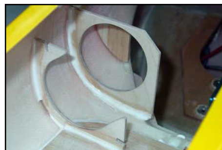
(below) The milled plywood supports for the hopper tank are included in the kit.
