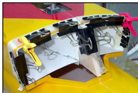
(above) The front edges of the inlet ducts are glued to the fuselage lip with epoxy/micro-balloons and clamped in position.
