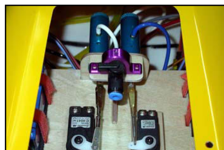
(below) One possible location of the optional Festo manual fuel shut-off valve. This is an important safety feature & should be fitted.
