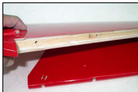
(above) The positions of the four rudder hinges are already marked in the Fin T.E. for you.
