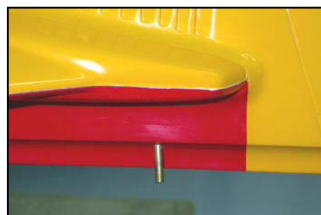
(above) Run the 'vent' from the 2 main tanks to a connection on the bottom of the model. (ie:: in the missile rail groove as shown here.)
