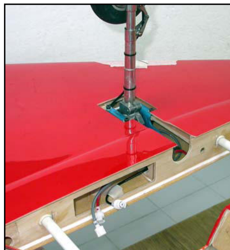
(below) 3 coloured tubes for gear up, down & brakes through an angled hole drilled in the balsa web behind each main gear unit.
