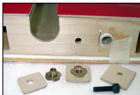
(above) Milled plywood parts and M6 allen bolts with blind nuts for the wing fixing.
