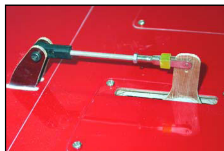
(above) Note the short length of Tygon tubing over the clevis to prevent it opening in flight. Use locknuts on the M3 bolts that hold the ball-links to the elevon horns, with a drop of Loctite to be sure !
