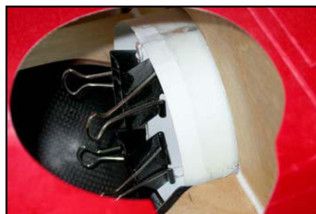
(below) Clamp the back edges of the ducts and balsa plate together while glue dries. Add a length of 1" glass tape over the joint also.
