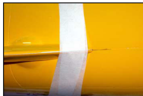
(above) The 'neutral' position of the canards is when the mould seam on the Leading Edge is on the moulded-in panel line.
