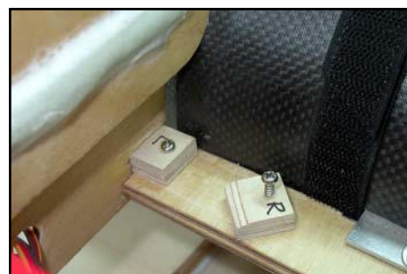
(above) The 2 wedges are made from the milled plywood parts supplied, and secured to the mounting rails with sheetmetal screws.
