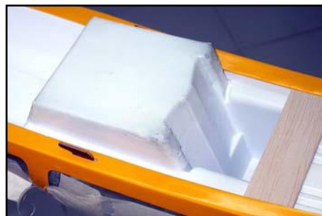
(above) The bottom surface of the cockpit tub can be reinforced with a piece of 80gm glasscloth and laminating epoxy to prevent any damage to it on the airfield.
