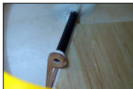
(above) Plywood 'P' plates are factory-installed on the canard tubes.
