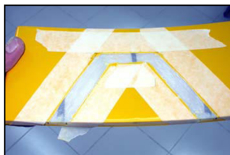
(below) Scuff up mating surfaces and glue in the curved plate above the inlet with 30 minute epoxy. tape in place until cured.
