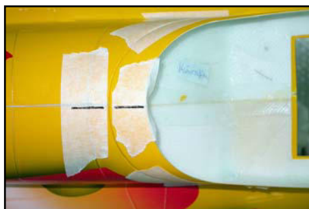
(below) Mark accurate centrelines on fuselage and canopy frame at back and front.
