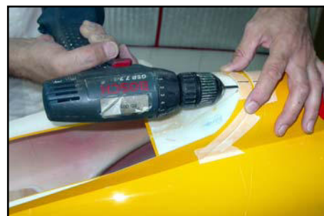
(above) Drill 3mm Ø through the back of the canopy frame into the fuselage for the hatch latch.
