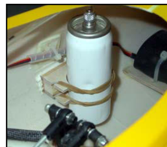
(above) On-board starting gas tank installed vertically in 2 small plywood hoops, with rubber bands.
