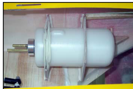
(above) The completed hopper tank installed, and retained with a rubber band in the slots of the front bulkhead.
