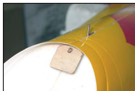
(above) The completed Hatch Latch should project through the plywood plate by about 1mm.
