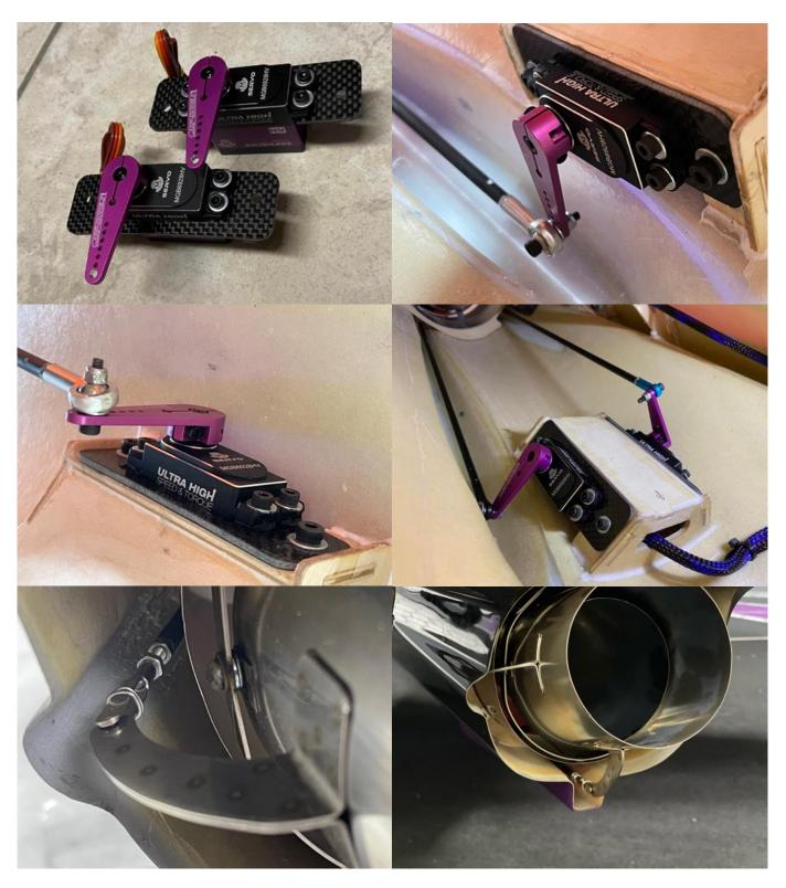
**Thrust Tube / Turbine Installation**
