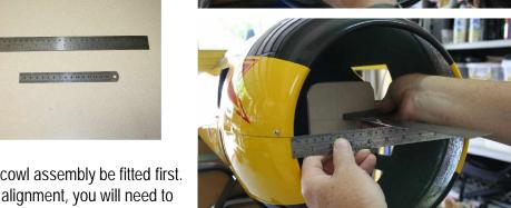
The engine installation requires that the cowl assembly be fitted first. In order to obtain correct engine to cowl alignment, you will need to get some reference marks that can only be obtained when the cowl is complete and fitted. The engine dome has right thrust already built
