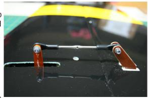
The stab tube is already complete and ready for you to use, no more needs to be done other than fit the tube to the stabs. The retention bolts have been pre fitted for you, and only requires you to fit the stabs to the fuselage. The stab tube may already be marked with L and R, to help you distinguish the correct orientation. If not, don't stress, it can only go one of two ways!
