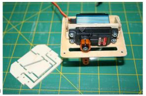
Assemble the push rods from the components in the parts bag. If necessary trim to length. The servo arm should exit the hatch at 90° to the hatch. Ensure that both the aileron servos are aligned like this. The push rods for both sides should be the same length. If you wish to use after market turnbuckles a 60mm or 2.5" item is required. Alternatively a ball link can be used in place of the alloy clevis.
