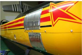
as the top layer when most of the shaping is done to add strength and a tough surface. Use some card to get the basic shape you require, and then trace the shape onto the balsa. The thin ply can be easily cut with scissors and the final shape trimmed with a sanding block. We used medium CA to glue the ply to the balsa.
