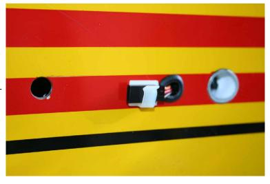
tion dowel. But it does need to be in line with both of these holes. However be aware there is a former just aft of the rotation dowel hole. A good location is 25mm forward of the stab tube.
