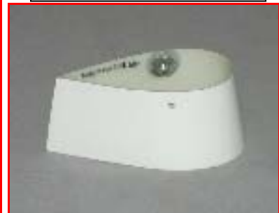
The Gee Bee now comes with a fiberglass tailwheel fairing. The fairing is secured using the TW axle. The axle is secured using the set screws at the bottom of each gear leg.
