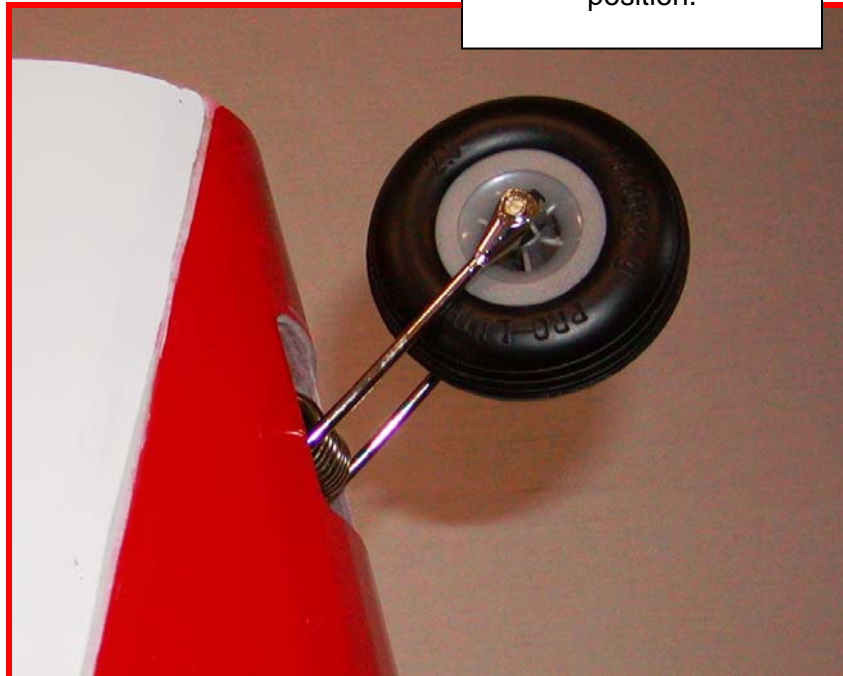
Completed tail wheel assembly epoxied into position.
