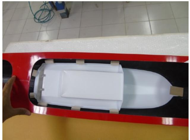
Then, when the glue has set, install the vacuum formed cockpit from inside, of course after you painted it to your liking. If you have a few instruments or side panels lying around, they would for sure enhance the looks of the cockpit. We have decided that the CARF-Models BOLT! looks too good to not boast a clear canopy and a cockpit, so that little extra work is well invested and you will love the result. use 6-8 scrap balsa blocks and a thin plywood in the front to secure it removable.
