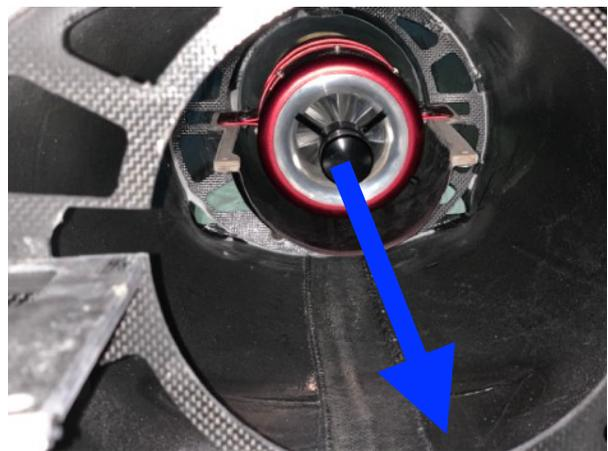
Once you are confident that you do not need to access the area inside the fuselage behind the engine formers anymore, bolt the integrated engine unit tight. Attach the rear fuselage cone to hold the thrust tube in center.
