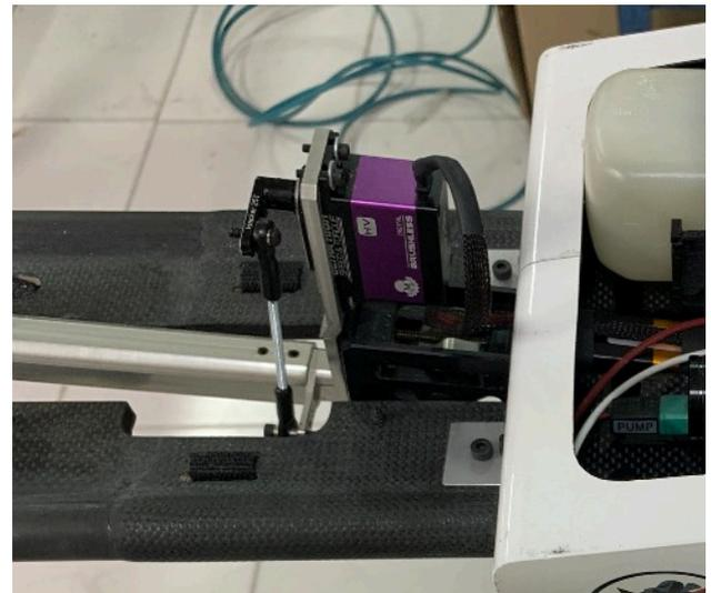
We include two 10 degree hard wood wedges in the hardware bag, these get glued to the gear plate at the correct position. Then the 4 mounting holes should be drilled with 3mm dia and the gear unit mounted with the self tapping screws.
