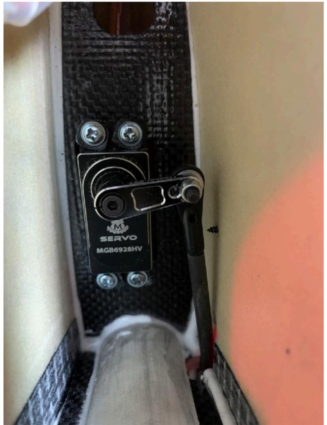
deflection of approx. 50 mm (2") right and left, measured at the root. The linkage should not hit or bind with the fin tube. You should set the neutral position of the servo arm not 90 deg to the servo, but 90 degree to the linkage, which is in an angle. That means, the servo arm is pointing slightly forward when the rudder is neutral.
