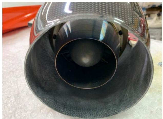
edge of the bypass cover to allow the wires to go through. We recommend to only notch the front edge of the cover, instead of drilling holes and feeding the wires through these holes to plug them into the engine, simply because in the tight space it is easier to put the bypass cover on AFTER the connectors are plugged in to the engine.
