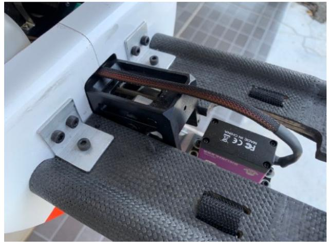
**forward**, away from the gear unit, otherwise it will rub or squash the wire when retracting. Also we strongly recommend to grind a flat spot in the gear pin, where the control arm is clamped. This arm has only ONE grab screw and this should have a flat spot. All other grab screws will not mandatorily need a flat spot because there are multiple ones applying a lot of force, creating sufficient friction.
