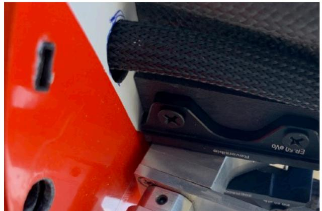
Now grind an opening in the vertical surface of the removable nose part exactly where the connector is to be placed. Then slide the female part on the connector in the fuselage, apply a little 5 min epoxy on it and slide the nose hatch over it. Wait 10 min until the 5 min Epoxy has set and then pull the nose off. Now you can create a nice fillet around the connector in order to have a very safe connection for the nose gear servo.
