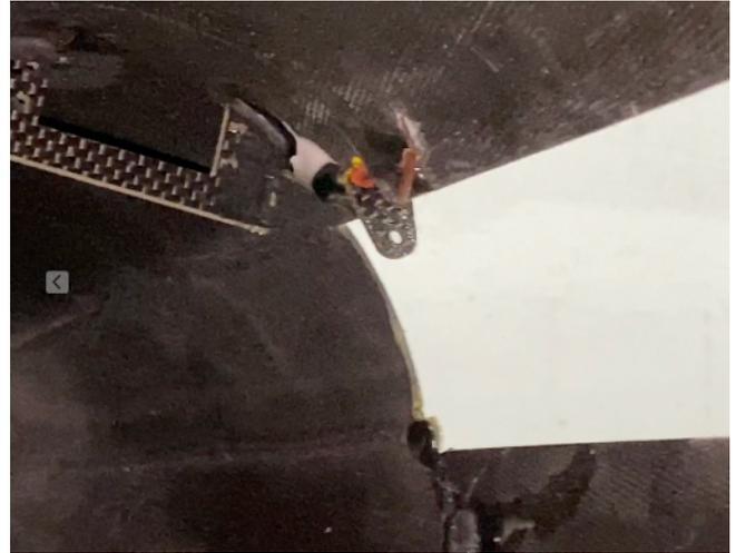
That keeps the load on the servo to a minimum and applies the highest holding power to the gear door. Because of the over-kneeing of the servo arm and linkage a single sided ball link must be used on the servo arm, so even here a metal arm is a must.
