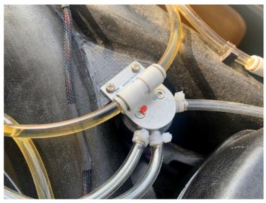
also take care that the smoke injector tube clears the canopy hatch when sliding it back into position on the main fuselage, and that it isn't in the way when removing the bypass cover to quickly access the engine. A bit tricky, but it can be done and it is the best way to do it.
