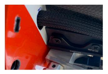
Now grind an opening in the vertical surface of the removable nose part exactly where the connector is to be placed. Then slide the female part on the connector in the fuselage, apply a little 5 min epoxy on it and slide the nose hatch over it. Wait 10 min until the 5 min Epoxy has set and then pull the nose off. Now you can crate a nice fillet around the connector in order to have a very safe connection for the nose gear servo.
