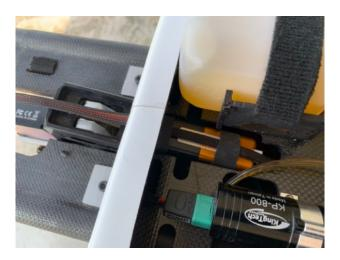
Make sure that the motor of the gear unit fits through the front face of the main fuselage and clears the RC equipment board inside. There should be a few mm clearance around the motor, that under no circumstances this motor could be hit or bent. As you see, you can slide the nose dual carbon tube unit in and out easily and just secure it with two M4 bolts through the aluminum angle brackets.
