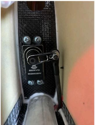
deflection of approx. 50 mm (2") right and left, measured at the root. The linkage should not hit or bind with the fin tube. You should set the neutral position of the servo arm not 90 deg to the servo, but 90 degree to the linkage, which is in an angle. That means, the servo arm is pointing slightly forward when the rudder is neutral.
