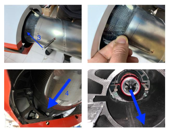
Once you are confident that you do not need to access the area inside the fuselage behind the engine formers anymore, bolt the integrated engine unit tight. Attach the rear fuselage cone to hold the thrust tube in center.
