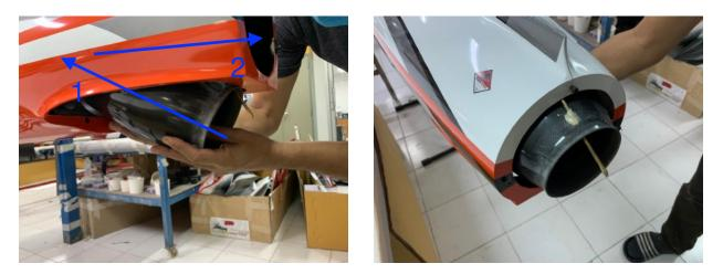
second pair of hands available, to channel the unit through the openings in the formers and then place it on the mounting rails.
