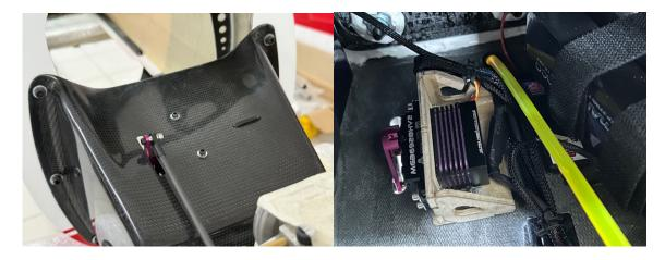
• Because you're already working on the engine dome you can install the ignition switch as well as the fuselage connector and the fuel line which connects the carburator and the fuel tank.
