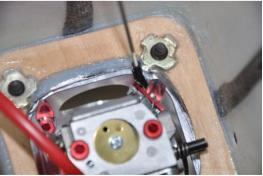
First install the throttle linkage. A DA-60 has already a throttle arm installed with a pre-drilled and tapped M2 thread. The CARF kit comes with a M2 pushrod
