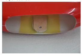
Once the epoxy has hardened, re-drill the hole with 7.5mm dia and at that time, also drill an access hole into the opposite side of the wheelpant. This access hole should be trimmed with a round file so that the head of the M6 axle bolt would fit through.
