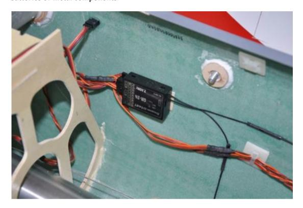
First create the elevator extensions. Determine the length and either solder them, or prepare readily confectioned lead extensions. Fix them to the fuselage wall with cable tie sockets. Don't forget to use a drop of thick CA glue to the center of the foam tape pad, otherwise they will fall off over time and might cause fatal malfunctions when the wires contact the hot tuned pipe.
