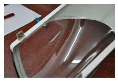
Now use 30 min epoxy and apply it from the inside along the edge of the canopy. Watch it soak in between the two surfaces. Hold the canopy frame inverted until the 30 min epoxy is cured.
