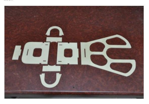
If you have your rudder cables permanently installed, you can simply cut the rear vertical former to get the cable through, before you glue the unit in place.
