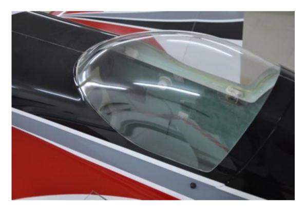
Then cut along the line and insert the canopy in the frame, to see how it fits. Be VERY CAREFUL for scratches along the side of the canopy, when you insert it into the frame.
