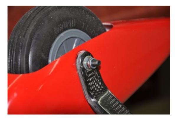
In this photo please look at the final result. The wheel is perfectly centered in the wheel pant and safely mounted to the landing gear. Please use packs of 6mm washers or collars, depending on which tyre you house. You might have to use collars/washers on both sides of the wheel to center it properly.
