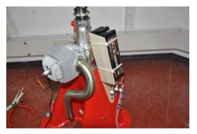
Most importantly use rubber grommets around the edges of the cable holes. You can use slotted fuel tubing and glue this around the edges. This is vitally important for the flight safety. If you do not use protection grommets the wires will be cut within a few flights, and electric failure will occure ultimately. Do the same with the ignition cable on both the motor dome and the cowling!
