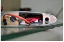
It is a very tight space in the stab. Standard size servos like JR 8911 or 8711 do fit! But definitely a little patience and some careful sanding might be needed, to remove excessive glue or wood burr. Slide the servo in and prepare yourself to cut the slot for the servo arm into the bottom skin.
