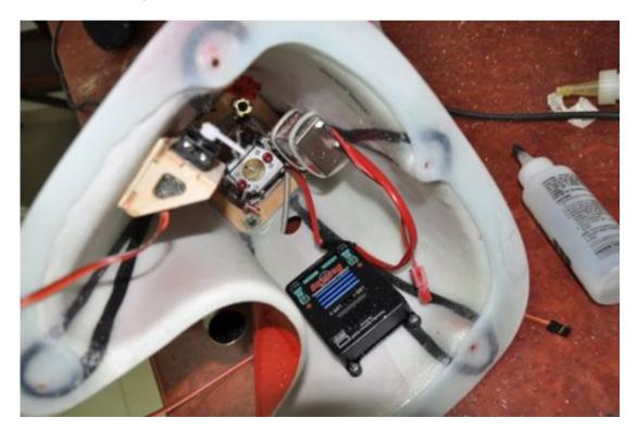
The ignition module can be mounted inside the motor dome as well. We slot the skin in 4 places and use two cable ties to fix it. For additional safety, you should
