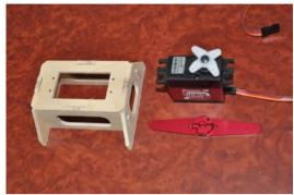
Now you have to decide whether you want to use a full tuned pipe or a canister. To compensate for the weight of the long pipe, it is recommended to mount the rudder servo as far forward as possible. The best spot is right behind the gear mount.
