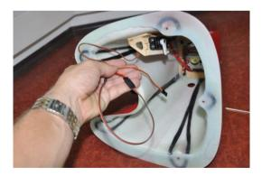
For the throttle servo, it would be wise to use a readily confectioned extension, giving you a chance for easy disconnection when having to take off the motor dome.
