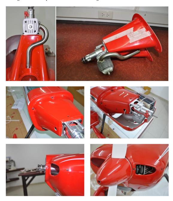
Use 6mm washers to set the perfect distance and thrust lines. Once the spinner backplane lines up perfectly with the cowling, the thrust lines will be perfect as well.
