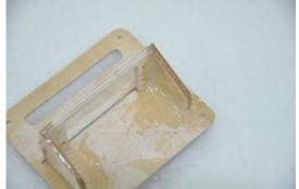
Glue the parts with thick CA first and once fit and function is checked, fill all joints with 30 minute epoxy. Fill the 30 min epoxy with some milled glass fibre or cotton flock. On the inside of the side supports you MUST use a patch of fiberglass cloth (included in the latest kits) to increase the gluing surface. You are going to install VERY powerful servos here and you risk them breaking lose from the hatch if you do not use the fiberglass patch to reinforce the joint!
