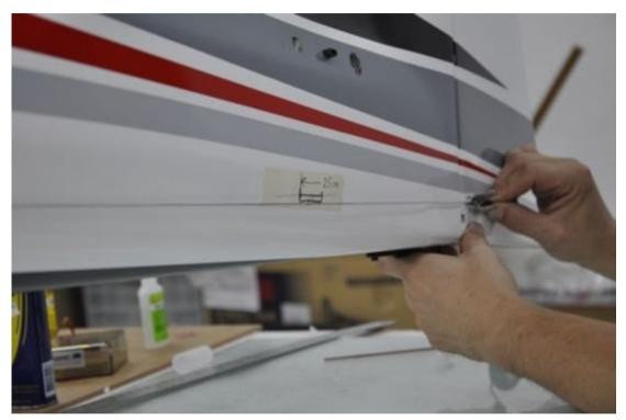
In longitudinal position, the front end of the slot should be 25 cm (10") forward of the read edge of the fuselage. Use some masking tape and a pencil to prepare the final position marking.
