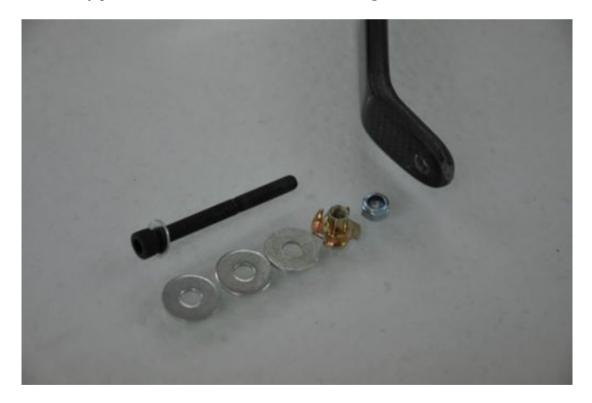
The suggested installation is extremely rigid, as the axle is made by a strong Allen Bolt with SHAFT, which is mounted with a T-Nut and a Safety Nut to the landing gear. The T-Nut is pre-inserted into the wheel pant and holds it securely in place as well. A pack of spacers, which could be M6 washers or even 6mm collars, depending on the withj of the wheel used, will then center the wheel in the wheel pant.
