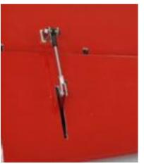
Cut the 2mm steel hinge pin to the correct length, bend one end 6mm (1/4") 90 degree, **grind/sand the other end pointed** and insert the pin **from the root**. This will secure the pin in place so that it can't slide out unintendedly.
