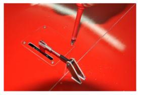
Finally check the movement of the aileron. With maximum servo travel you should be able to reach the max down deflection of the aileron, before it hits the spar. You do not need more up deflection than down deflection. The ailerons are VERY efficient. If necessary, enlarge the slots in the servo hatches slightly to allow maximum servo travel to each side.
