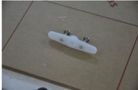
Mount the rudder in the same style as the elevators to the stab. Cut the hinge post to the required length, bend 6 mm (1/4") 90 degree, point the tip and insert from the top. Here we recommend to grind a groove into the top of the rudder so that the 90 degree bend can be counter sunk into the surface. Secure with a strong tape or a drop of 5 min epoxy.
