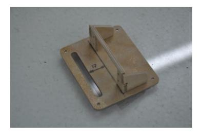
Clean up the milled plywood parts and check the fit. Sand edges and most importantly, the back side of the servo hatch well. Clean the sanded hatch from dust with Acetone or lighter fluid. Check with the servo you're going to use the distance of the servo frame to the slot. With Graupner/JR servos this is usually 20 mm to the center line of the arm, which means, 17mm between the frame and the close edge of the slot.
