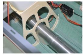
Now push the pipe on to the Teflon coupler. Don't forget to slide the two clamps over first. If you use a hot air gun to soften the Teflon coupler this is going to be very easy. Secure the joint with the two clamps. Then squeeze 4 pieces of the included silicone tubing into the T-shaped slots of the rear mount and permanently glue it with 30 min epoxy to the fuselage floor. Stiffen it with triangular scrap plywood pieces as vibration might brake it off quite easily.
