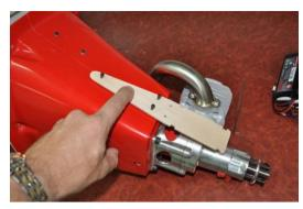
Next is the battery mount. Later kits have a readily milled part, others require the manufacturing of a simple plywood tray. The purpose of this tray is to mount the batteries as far forward as possible (even with the tuned pipe you do not need any additional weight if you follow these instructions!!!) Bolt it with 3 M3 bolts/T-Nuts to the side of the motor dome. Make sure the battery pack clears the cowling and as a thin layer of balsawood as a heat insulation from the header.
