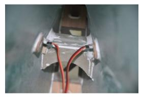
If not already done, extend the rudder servo wire so that it reaches the receiver safely. Here you have to be especially careful to route it away from the hot pipe and hold it close to the fuselage wall with cable ties and sockets.
