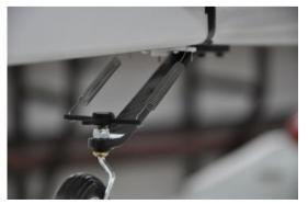
After the rudder is installed permanently, use the two springs and connect the tail wheel control arm with the servo arm you screwed to the rudder.
