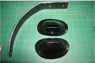
The undercarriage legs for the Composite – ARF Extra 330SC are very strong and very light, thanks to the laminated carbon manufacturing process that has been used. The legs are held in place with four - 6mm x 20mm cap head bolts, the legs are already pre drilled for you. The T-nuts are already pre fitted to the undercarriage mount plate for you at the factory. Two bolts are used on each leg, and are inserted from the bottom of the fuselage.
