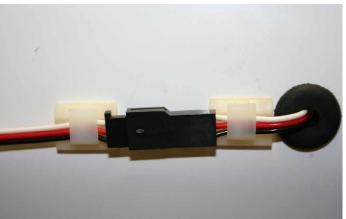
Don't forget to protect your servo and extension leads when and where they exit the wing or enter the fuse-
