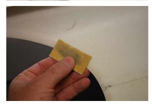
It's important that you fit the canopy while the canopy frame is attached to the fuselage, this will keep the frame properly aligned and not twisted. Masking tape is used to hold the canopy in position prior to gluing. It may pay to have another pair of hands available to assist you here. Perhaps you can bribe your best buddy with a beer, or two (after their assistance)!
