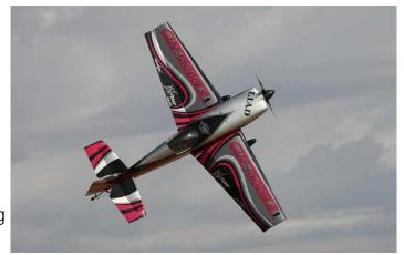
The result is an ultralight wing with an aileron allowing more than 30 deg deflection to both sides and driven redundantly by 2 servos. The outer servo has been moved inwards, to further move weight from towards the centre of the plane. This results not only in highest roll rate, but also even further improved snap-and-stop performance. Modified angles of attack of wing and stab reduce the knife edge mixing.
