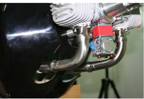
brands and styles of exhausts. Adjustable headers were also used to fine tune the positioning of our canister. Adjustable headers such as those produced by MTW and KS really make the canister installation process much easier. If you wish to use readymade headers you will need a set with a 75mm drop.
