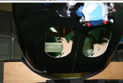
Mask off the bottom of the engine dome in preparation for marking out the desired cut out area. Again the area that needs to be cut out will vary dependant on your exhaust selection. It's important with a dual canister installation that you keep the centre seam area intact, try and leave at least 20mm on either side of the seam uncut.
