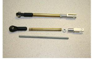
The stab tube is already complete and ready for you to use, no more needs to be done other than fit the tube to the stabs. The retention bolts have been pre fitted for you, and only requires you to fit the stabs to the fuselage. The stab tube may already be marked with L and R, to help you distinguish the correct orientation. If not, don't stress, it can only go one of two ways!
