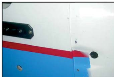
(above) Drill 10mm Ø holes in the fuselage to clear the back T-nuts that hold the top & bottom parts together.
