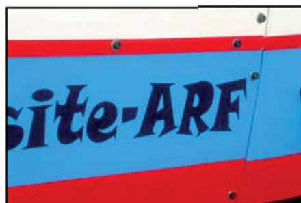
(above/below) The cowling is secured with M3 bolts and washers, into T-nuts that are glued inside the fuselage.
