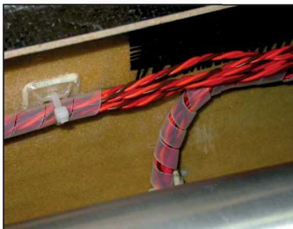
(above & below) It is very important to protect all tubes & wires where they pass thru' fibreglass or carbon parts, or near to composite milled parts, where they could be damaged due to vibrations. Use grommets or split silicone tube around the edges of holes in composite material, and plastic spiral-wrap.
