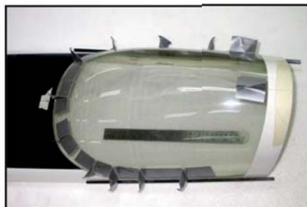
(above/below) With the clear canopy tacked into place with the frame on the fuselage, carefully remove it & complete the gluing on a flat table. Secure all around the inside edges with epoxy and micro-balloons mixture.
