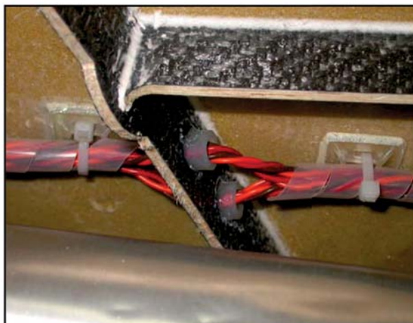
(above & below) It is very important to protect all tubes & wires where they pass thru' fibreglass or carbon parts, or near to composite milled parts, where they could be damaged due to vibrations. Use grommets or split silicone tube around the edges of holes in composite material, and plastic spiral-wrap.
