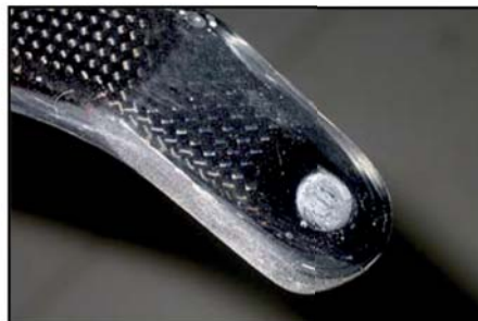
(above) The moulded dimple in the bottom of the carbon legs. Drill a central hole of 6mm diameter.
