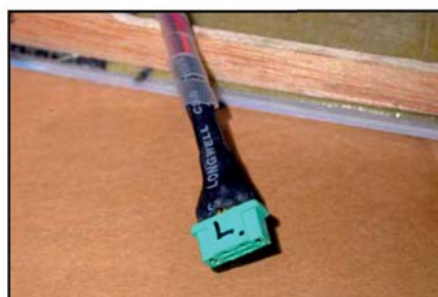
(above/below) We use these 6-pin Multiplex connectors for all the removable connections between wings/stabs and fuselage.
