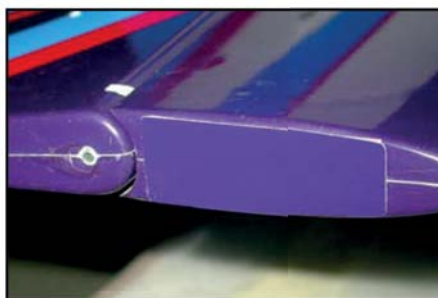
(above) Servo access hole in stab tip is covered with pre-painted tip fiberglass sheet included in the kit.
