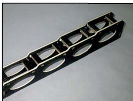
(below) The completed rudder tray is light and very stiff.
