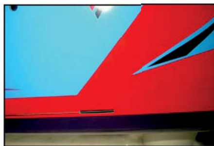
(above) Cut the slots for cable exits with a sharp knife. If the rudder tray is in the standard position, then the back of the slot will be 355mm from back of fuselage, and 48mm up from bottom of fuselage.
