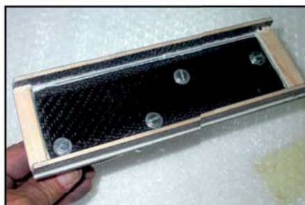
Top and bottom views of the rear tuned-pipe support.
