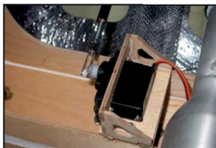
(above) The throttle servo mount is made up from the milled plywood parts supplied in the kit.
