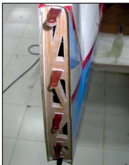
(above) The phenolic hinge points are all factory-installed and aligned, with double-thickness at the top and bottom positions.
