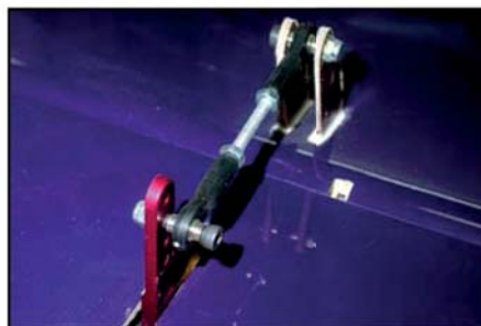
(above) If required for alignment you can use a single-sided ball-link on metal servo arms only .
