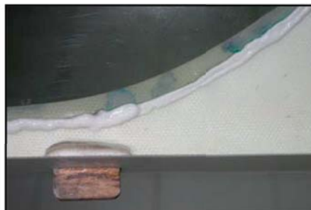
(above/below) With the clear canopy tacked into place with the frame on the fuselage, carefully remove it & complete the gluing on a flat table. Secure all around the inside edges with epoxy and micro-balloons mixture.
