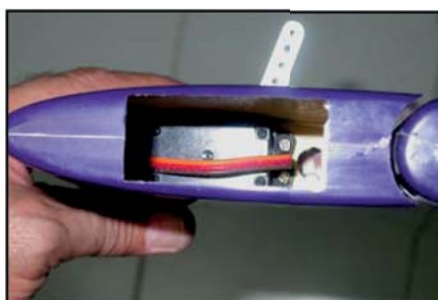
(below) Outer servos are fitted inverted, with output shaft towards the stab trailing edge.
