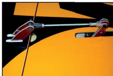
(below) The completed 3rd aileron servo horns and linkage, installed using a very long screwdriver from the root rib. A little fiddly to do - but neat.
