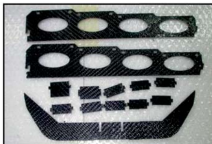
(above) The milled carbon/balsa parts for the rudder tray, and the end support bulkhead.
