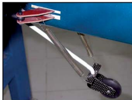
(above) Connect the steering arm to the rudder horns with springs for steering option if required. SuperXtra shown here.
