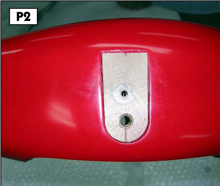
Milled plywood plate glued to wheelpant.
