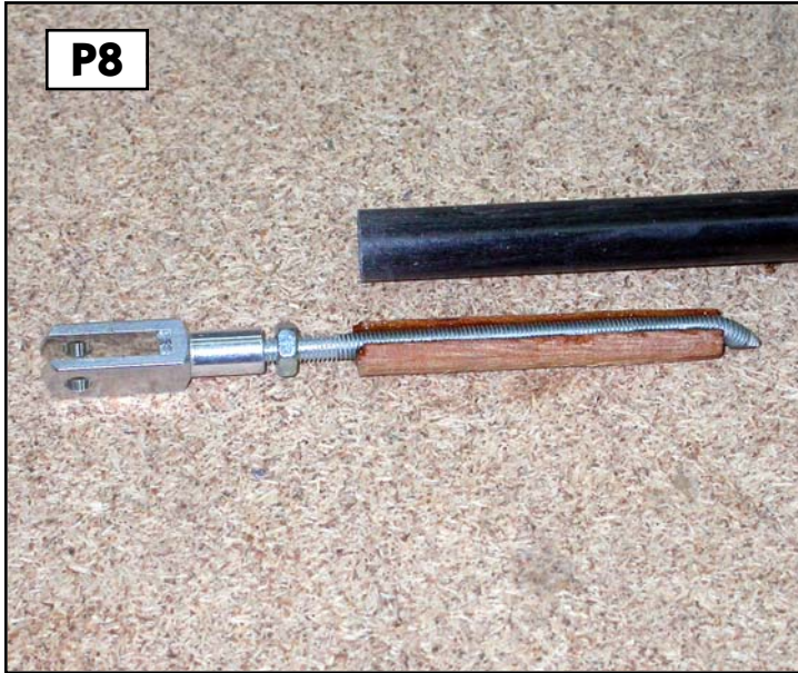
M3 threaded rod in wood dowel glued into carbon pushrods. (below) Cable separator and pushrod supports.
