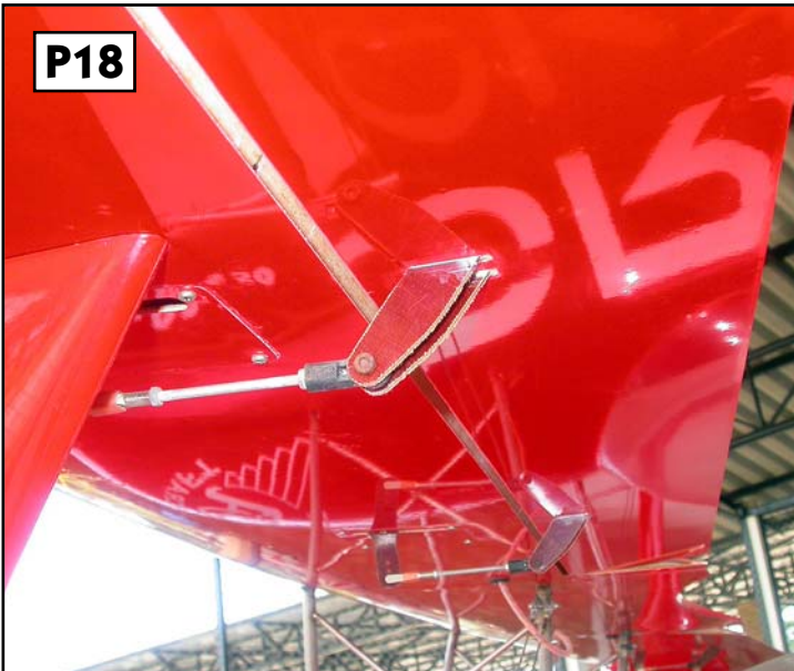
Aileron linkages on top left wing. (below) Silver-solder the M3 extenders onto the braided flying wires.
