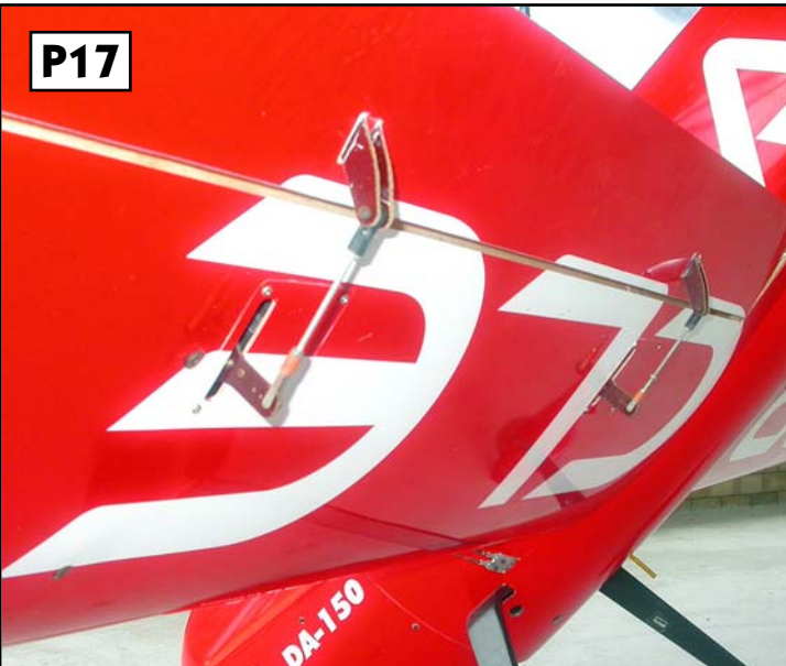
Aileron linkages on bottom left wing. (below) Aluminium inserts in outer struts fit into moulded pockets in wings.
