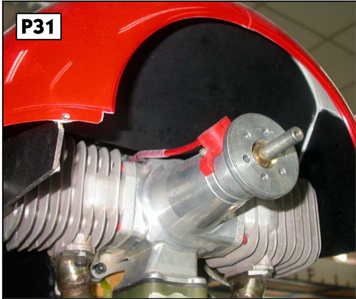
View to show engine baffles for DA-150. (below) Typical tuned-pipe tunnel construction.
