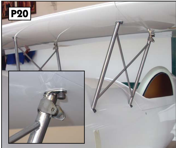
General view of stainless steel cabane struts and connection with M4 bolt into blind nuts.
