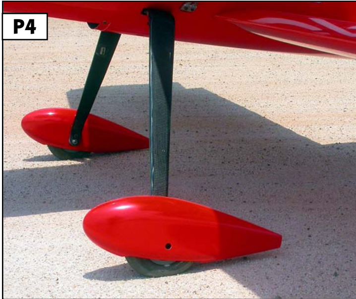
Wheelpant angle set so that back end just clears the ground.
