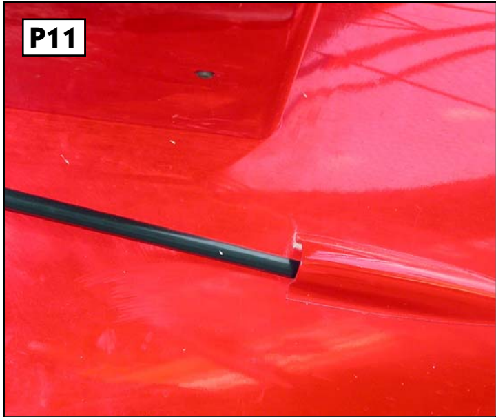
Shows elevator mounting plate angle supports and carbon rovings. (below) Elevator pushrod exit covers.
