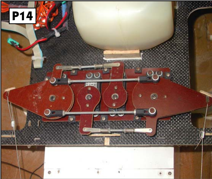
Completed rudder servo linkages. Note phenolic arms also secured with minimum 2 sheetmetal screws each.
