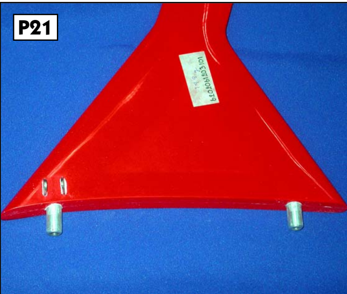
Aileron linkages on bottom left wing. (below) Aluminium inserts in outer struts fit into moulded pockets in wings.
