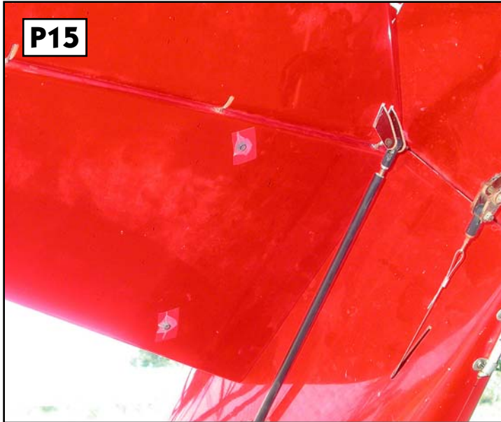
General view of elevator and rudder linkages, also shows stab retaining bolts and clear tape.
