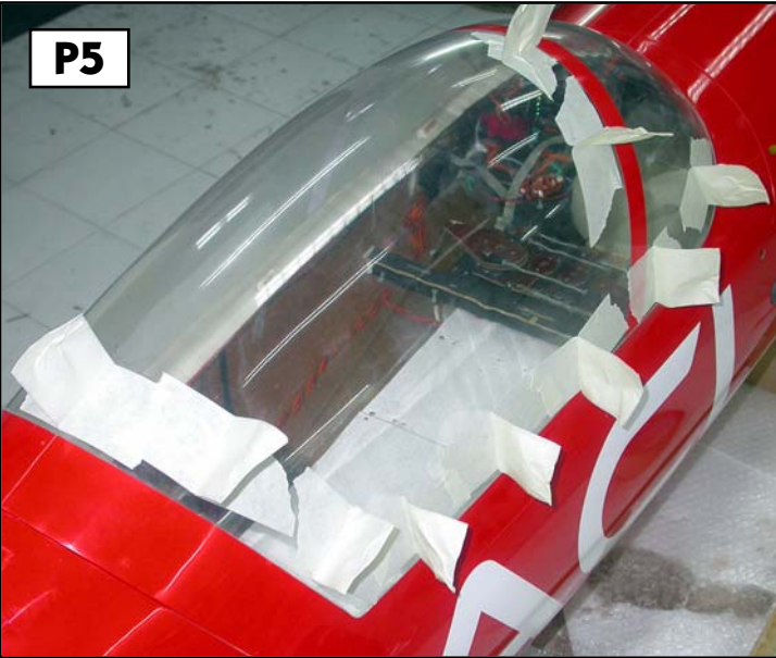
Tape handles to aid gluing clear canopy into frame. (below) Elevator linkage details (brass tube not shown)
