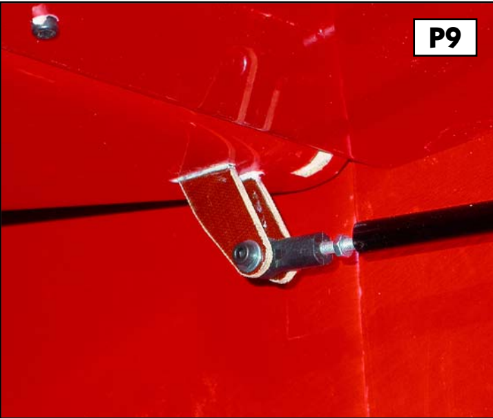
Tape handles to aid gluing clear canopy into frame. (below) Elevator linkage details (brass tube not shown)
