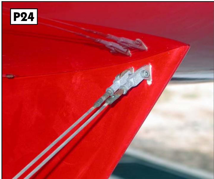
General view of stainless steel cabane struts and connection with M4 bolt into blind nuts.
