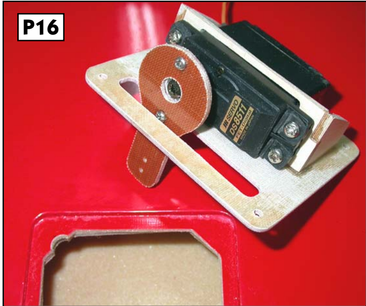
Typical aileron mounting from cnc milled ply parts. Make sure you secure with a fillet of epoxy all round the joints.
