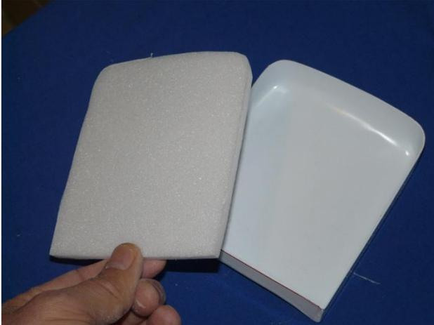
Before painting, the plastic surfaces should be “keyed” with a light sanding or wiping with Acetone (CAUTION: Acetone will dissolve the plastic if too much is used! Practice with a piece of scrap - very little is needed for this step).
