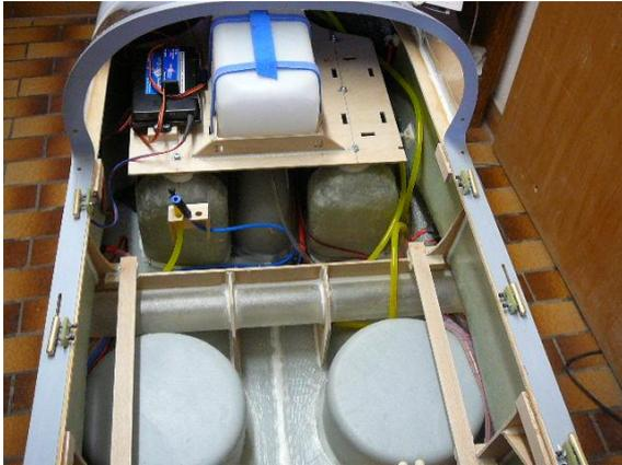
In the standard fuel tank setup, the tank is placed on the mounting platform, within the previously glued-in locating frame, and secured with the supplied hook-and-loop strap. The slots for the strap are pre-cut in the platform.
