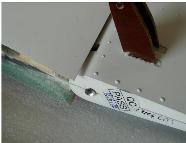
After trimming the hinge-pin to length (from the end opposite the flared end), it can be inserted and secured with a bit of tape over the flared end.
