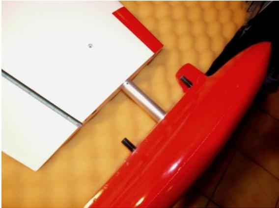
The wingtip tanks are factory ready for final installation with a single 3mm (M3) screw. The aluminum mounting tube is pre-threaded.
