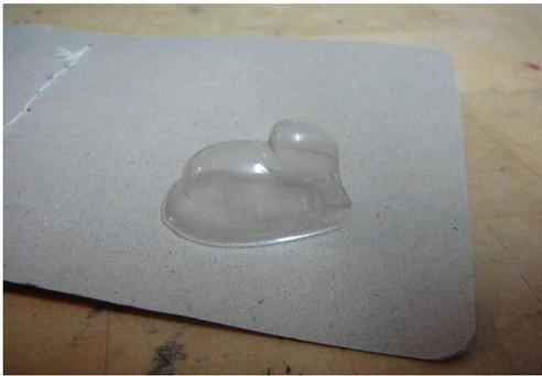
The shape of the position light cover dictates the shape of the baseplate that the lamps are attached to (some covers are simple teardrop shaped).
