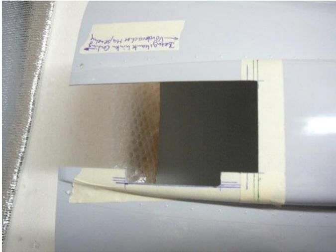
When making the cutout, be sure to take into account the movement of the servo with the gear leg!
