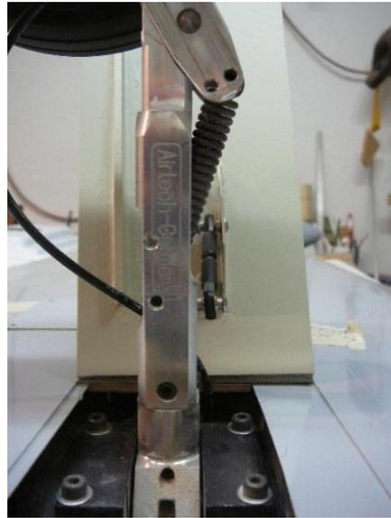
To prevent the main gear cover from fluttering and to assure a more positive sit within the recess, we added a lengthwise reinforcing strip. The final positioning is by trial and error to ensure that it does not interfere with the closing of the cover. It must not contact any part of the gear unit or airframe.
