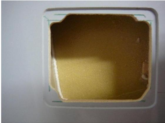
The servo opening must be opened up in order that the servo fits cleanly. Leave enough material in the corners to take the attachment screws.
