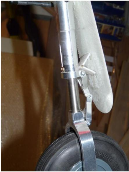
To prevent the door from fouling the scissor-link during gear cycling, a simple spacer can be made with a spare hinge, epoxied in place as shown. This simple fix assures appropriate clearance.
