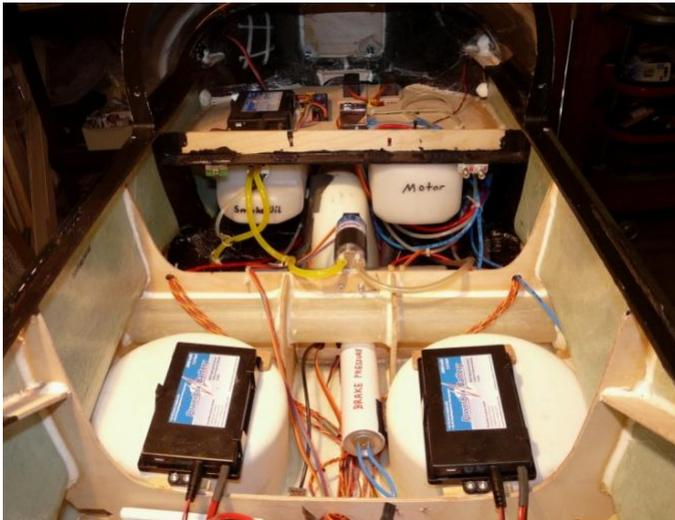
Shown here are the two 7.2V 2800mAh LiPo batteries. We recommend waiting till the build is in the final stages before installing them in a permanent location, as the relatively high weight can be used to advantage when setting the Center of Gravity.
