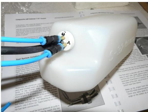
In our example here, FESTO fittings are used in the vent/overflow and fill/drain lines with the appropriate tubing (blue tubing in photo).
