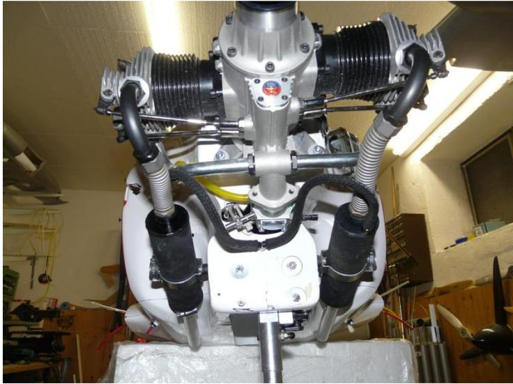
For the Moki installation, the oil-feed line is routed above the nose-gear unit, into the engine compartment, and from there to each muffler ("T" or "Y" fitting).
