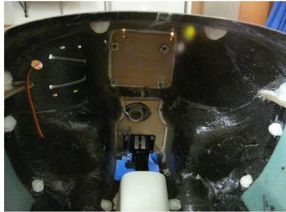
The opening beneath the motor bulkhead is for the carburetor air intake (from fuselage).
