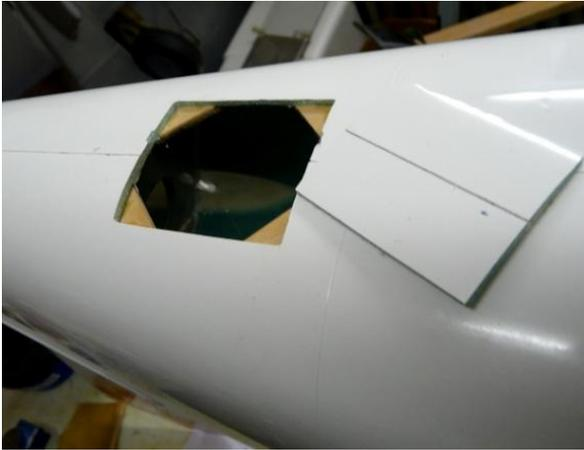
A hatch for the rudder servo is worked into bottom of the fuselage rear, with cover. This cover will be secured later with a screw in each corner.
