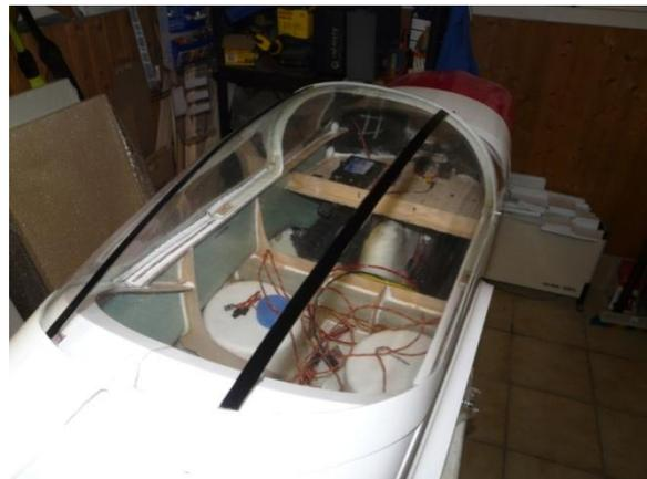
Once the cockpit glazing has been cleanly glued in and the glue is dry, it is time to fit the rear canopy braces. The attach points are marked on the canopy bow and the rear base frame. Before gluing, these parts are to be painted to match the documentation, dependant on the variant modeled. In the case of this particular model, gloss black.
