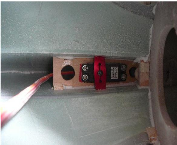
The rudder servo is installed into the pre-fabricated servo mount within the fin. The slots for the servo arm must be determined and cut. This is easily accomplished with the aid of a small, bright light (LED flashlight works well). The silhouette cast (visible on the outer skin) gives a good indication of the servo arm and rotation axis. A slot is then cut large enough to assure unrestricted movement of the arm and linkage.
