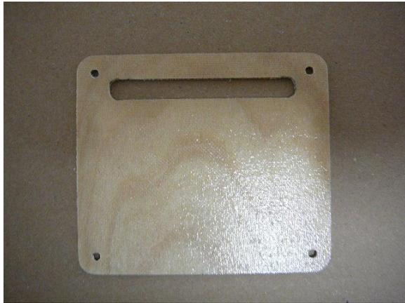
The servo is installed directly to the hatch cover with a plywood frame (frame glued to cover with 30 minute Epoxy) from parts included (see photo).
