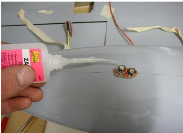
The baseplate is then glued to the tank using CA or Epoxy.
