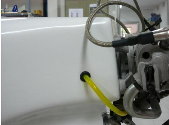
The opening for the fuel tubing can now be drilled in the right side of the motor dome.
