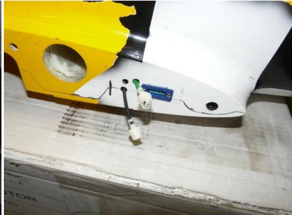
Photo: Wing connections (electric and pneumatic)
