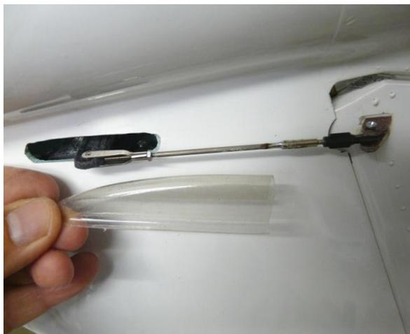
View of the rudder linkage (fuselage is on its back).
