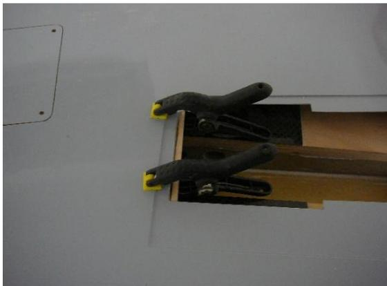
Rough up the inner gluing surface, cut a 3mm strip to size (90 x 15 mm) and glue into position with thickened 30 minute epoxy. Use clamps to secure till cured.
