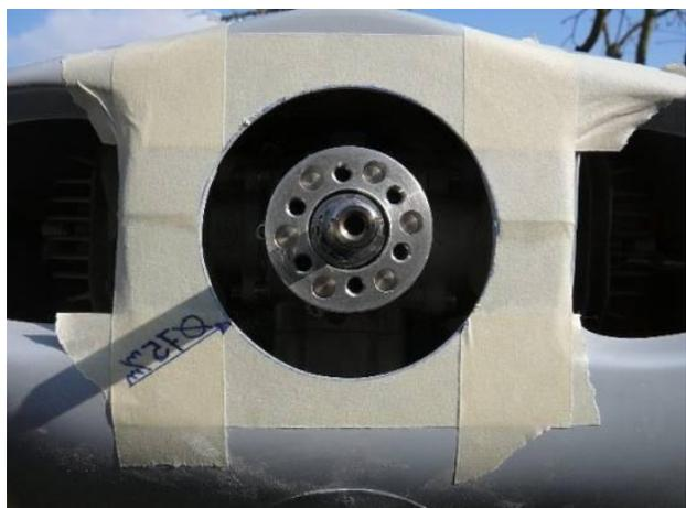
If a landing light is to be used, the corresponding marked area of the cowl must be cut open and cleanly sanded out to size.
