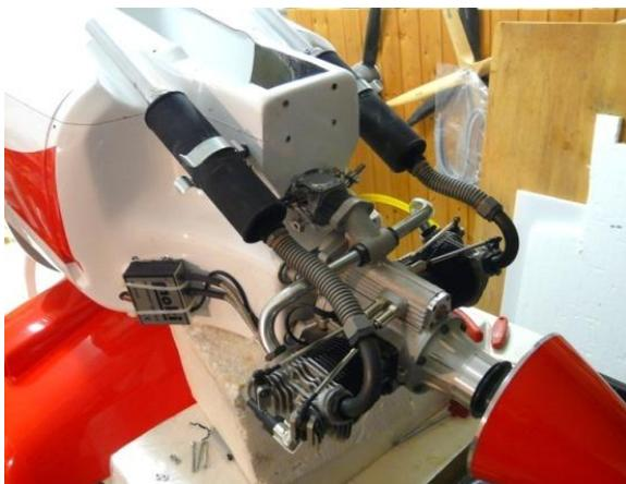
...and here it is with the stock mufflers (model shown on its back) and manifolds with flex extensions. These manifolds can be ordered, fitted for the SF-260.
