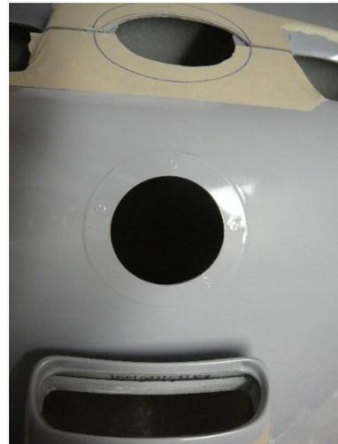
The gluing areas of the oil cooler scoop moulding - below the landing light - and the intake lip are lightly scuffed and cleaned prior to gluing. The lip is then glued to the main body of the scoop.
