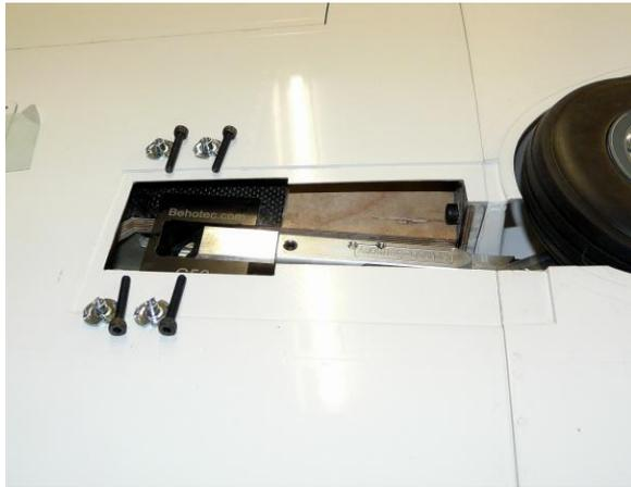
The socket-head screws and blind nuts for installing the gear are included in the accessory pack.
