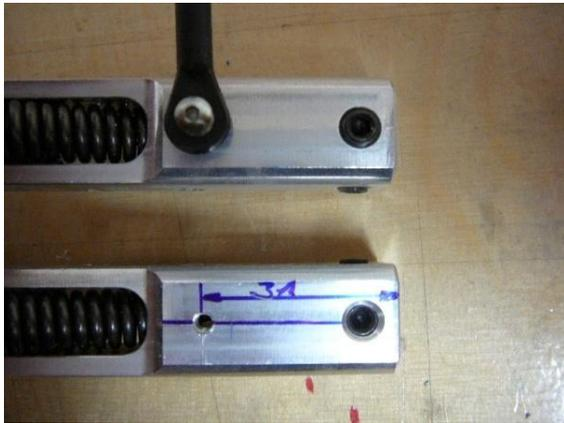
Before installing the set screws, we recommend filing/grinding a small flat at each point where they contact the steel axles, to prevent twisting in use. The gear leg itself is secured with four (4) screws, making this step uncritical.
