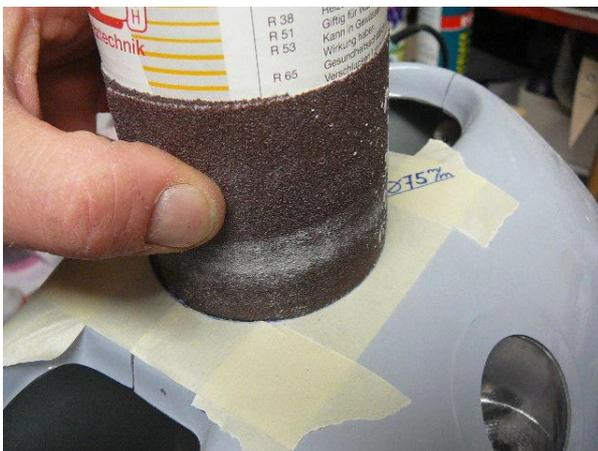
A good way to get a clean opening, is to use a sandpaper roll – somewhat slow, but accurate and easy on the paint. Or, if you've a steady hand, a rotary grinder will make short work of it.
