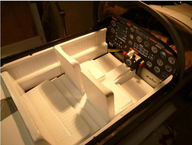
The proper fit of the side panels to the floor are best determined by trial fitting, as shown here. Before painting, the attachment points should be determined.
