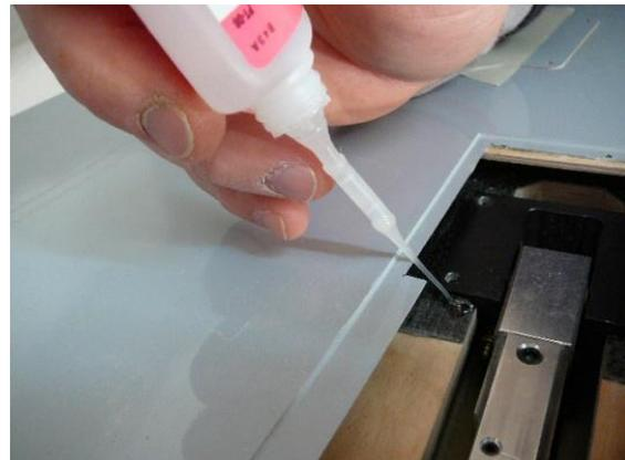
With the gear is aligned, a tiny drop of CA adhesive can be applied to the black mounting brackets to temporarily hold things in place. Use a bit of accelerator to keep the glue from wicking too far under the aluminium brackets. After drilling the mounting holes, the gear can then be popped loose.
