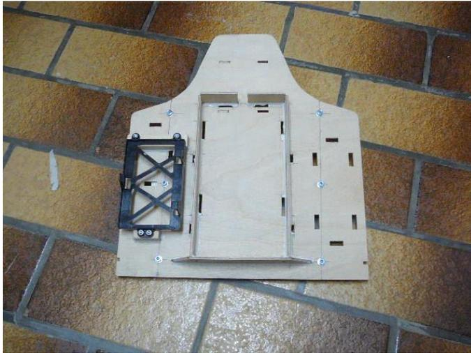
After mounting the motor, we recommend that the large plywood bulkhead (for securing the tank and other items) be installed in the proper position. Beforehand, the location for the throttle servo and the (optional) choke servo must be marked and cut out.
