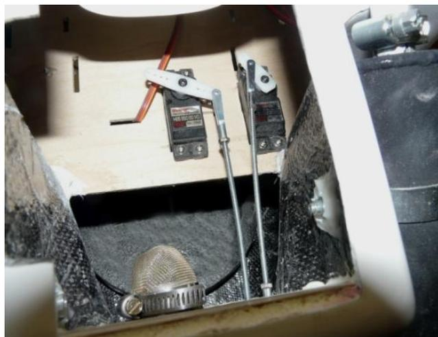
The pushrods for the throttle (shown here with the choke set-up) should be installed before installing the nose gear unit, as you have perfect access from the wheel well to the front part of the fuselage and the servos. The photo also shows an intake filter made from a tea strainer that has been trimmed and “hand formed” to size, attached to a carb intake ram tube (optional accessory).
