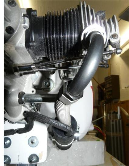
**NOTE! Use only special, heat resistant rubber tubing (generally included with the smoke pump kit) between the "T" fitting and the mufflers!**
