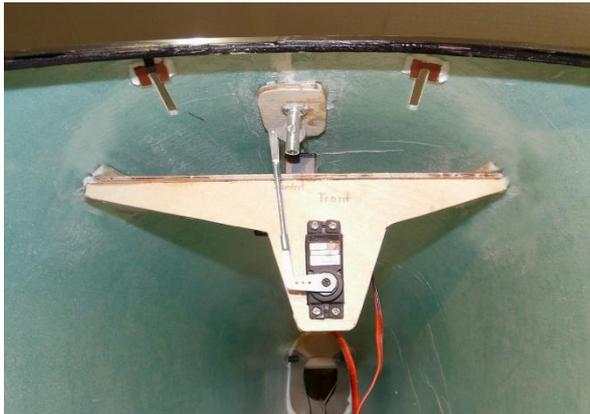
The servos can be mounted once the glue has dried/cured. The rudder servo is installed first, with the output arm oriented toward the fuselage bottom and fixed in place, as one of the mounting screws will be partially blocked by the (optional) tow release servo. Install the tow release servo only AFTER this step, if applicable.
