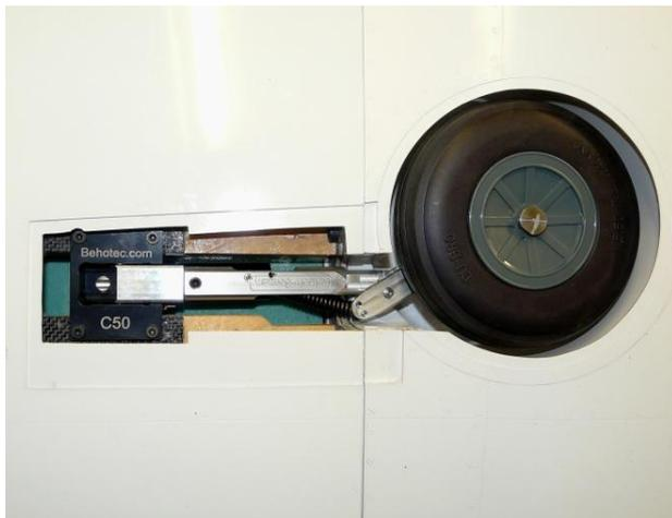
Once the Epoxy has cured, the bolts can be removed, the gear is set in place and secured.
