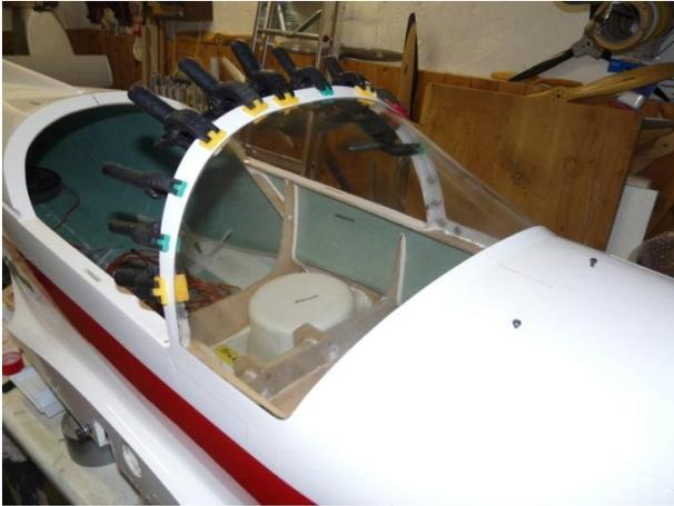
For holding the “glass” in place during gluing, small spring clamps can be used, or even better, strong magnets. The lower edges of the “glass”, and where the windshield fairs to the front fuselage, magnets are the better choice.
