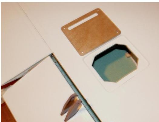
The aileron hatch covers and wood reinforced openings are pretty much ready for servo installation.
