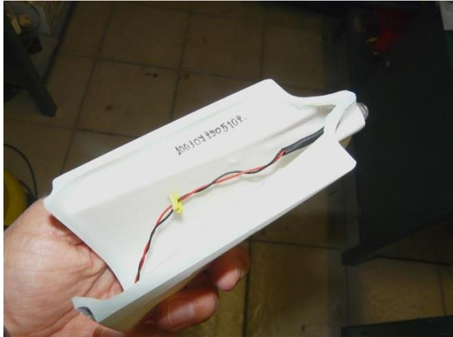
The (optional) white tail light should be installed before fitting the tail cone. The tail cone can be attached however preferred with silicone adhesive or screws (attachment materials are not included).
