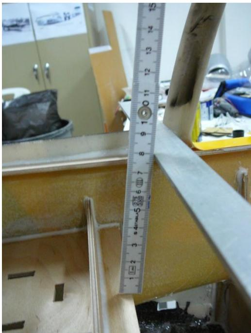
motor dome bulkhead. Ideally, the Moki air filter would be used. Its size, however, presents clearance issues with the nose gear retraction.
