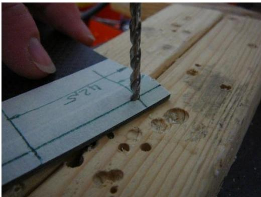
Then, remove the cover and open out the hole to 3mm (ONLY in the cover).
