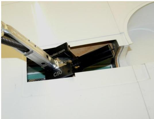
The gear assembly can now be slipped into place from the wheel well at a slight angle.
