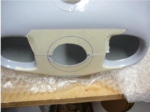
The horizontal separation line is also on the centerline of the opening for the propeller drive washer/shaft.
