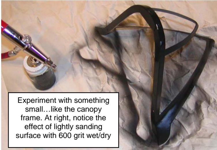
Experiment with something small...like the canopy frame. At right, notice the effect of lightly sanding surface with 600 grit wet/dry
