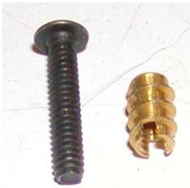
A black anodized button head machine screw (6-32) and brass threaded insert @US were used to secure the canopy. Once threaded to the correct depth, the brass insert is secured with a drop of CA glue.
