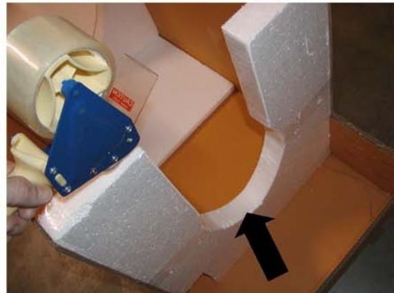
**Line cradles with packing tape to keep foam from crumbling.**
