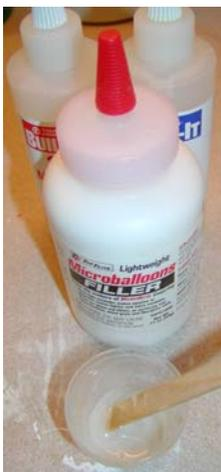
If you are satisfied with the fit and position of the baffles, make a thick mixture of epoxy and micro balloons and apply a narrow fillet to all baffle and cowl junctions
