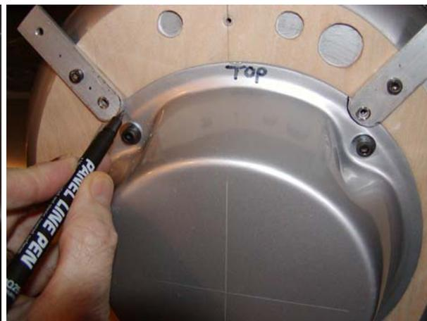
Remove the two upper cowl mounting brackets so the dome can be mounted temporarily. The ‘blind or T nuts’ will be installed on the opposite side of the firewall in a later step. Remount the cowl brackets and mark the areas of the dome that must be removed to clear the brackets. Use a sanding tool to relieve the dome for brackets.
