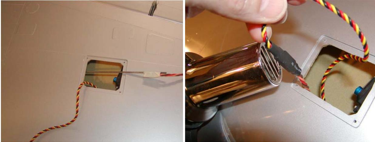
You should secure all hoses and leads in an orderly fashion so that they cannot interfere with the mechanical operation of the wing servos or retracts. Take care not to pinch the air hoses. Wires should be protected where secured and cable ties should be snug, but not overly tight:
