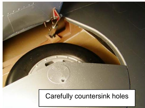
The wheels covers will most likely require spacing away from the gear legs for proper and secure fit. Using scrap wood, make spacers, contouring to shape until the wheel cover can be fastened using both screws; it should fit into wheel opening and not interfere with gear retraction.
