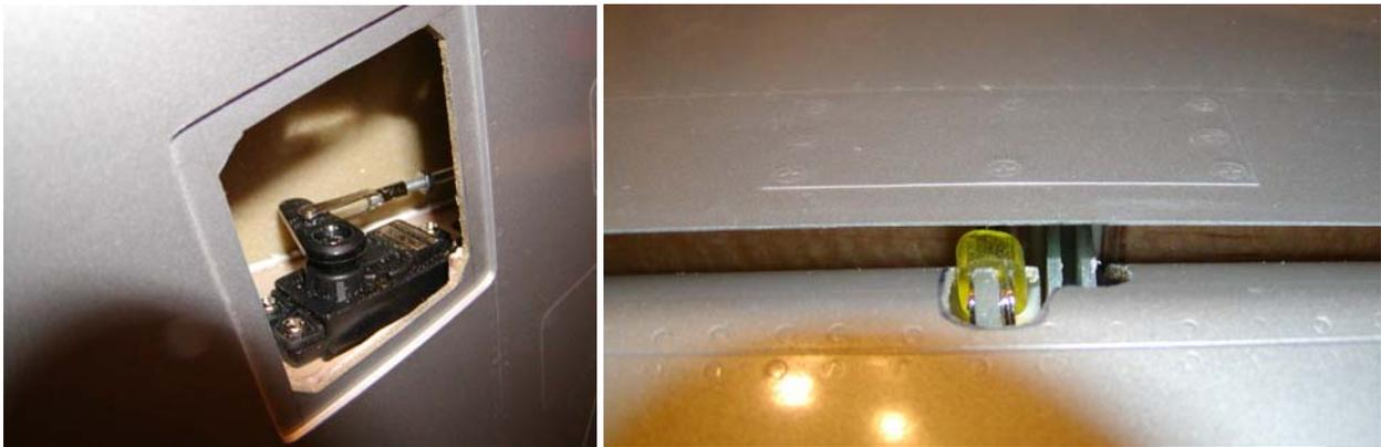
Aileron servo installed and pushrod connected to INNER hole. Aileron Horn is located on top of aileron next to center hinge. A short piece of gas fuel tubing is used to secure the clevis to the horn. Check for proper aileron deflection and no binding!
