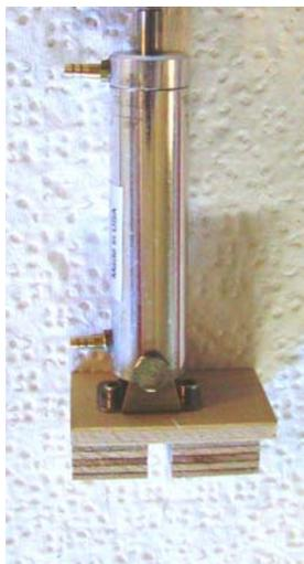
**Position and mount cylinder as pictured (left) then epoxy ply mount into position (right) to line up with gear door horn.**
