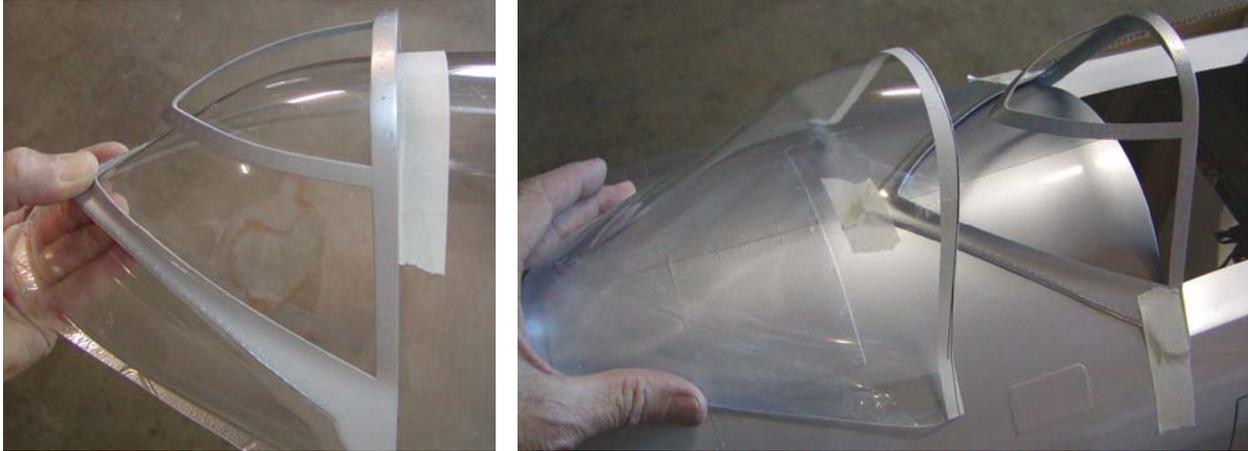
Use RC-56 @US or other clear drying, water clean up, multi-purpose glue to adhere the clear plastic to canopy frames. A mixture of epoxy and cut glass can be used around the plastic and canopy frame edge for a more solid bond if desired.
