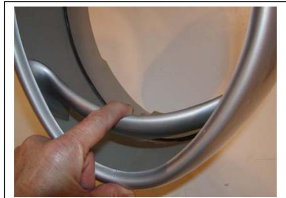
With the cowl mounted, tape the baffle into position. Look at a 3-view of the Thunderbolt if you are unsure of the correct positioning. When satisfied, mark the location and remove the cowl. Lightly sand the gluing surfaces; clean with alcohol; apply epoxy; remount cowl and tape to hold while the epoxy sets.
