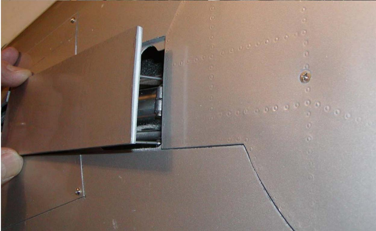
The hinge pin wire is cut to length a little bit at a time until the proper length is achieved such that the strut cover will lay perfectly flat when the gear are fully retracted:
