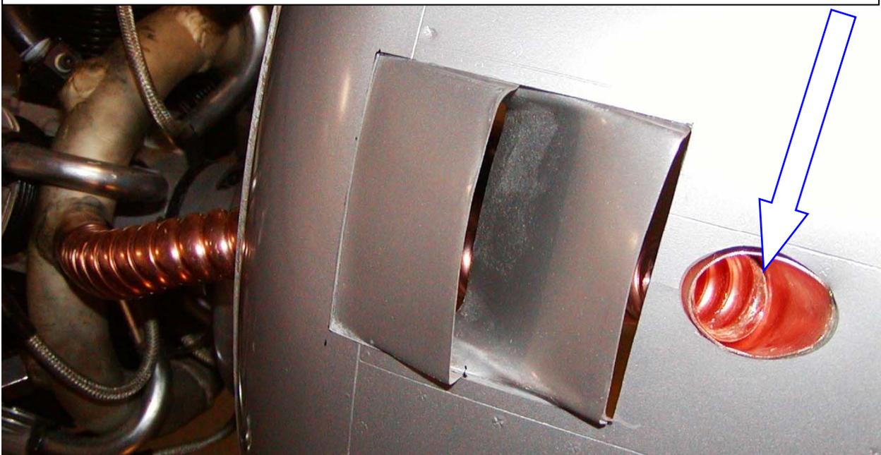
**\*\*hard solder** - using alloys that melt at greater than 450 degrees C. This includes brazing and high temperature solders. 'Hobbyist' solder will not survive Moki exhaust temperatures.
