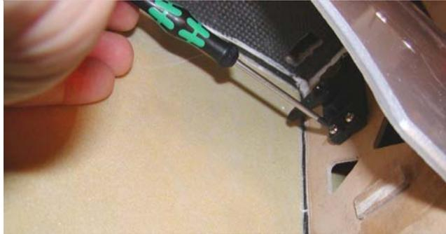
**The flap pushrod clevis is secured to the flap tiller arm by way of a retention pin and 'E' clip.**
