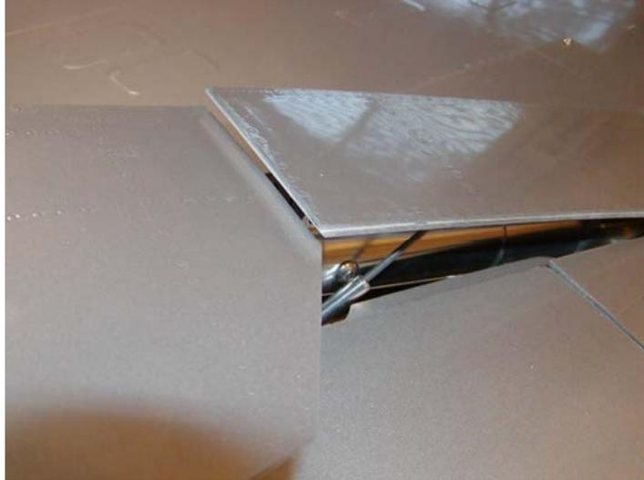
When 100% satisfied with the operation of the strut cover, abrade the hinge pins and clean with alcohol. Apply epoxy and cut glass mixture to pins and ball links. Insert pins, wiping any excess epoxy. Retract the gear fully and tape the strut cover tightly closed. Allow to dry.
