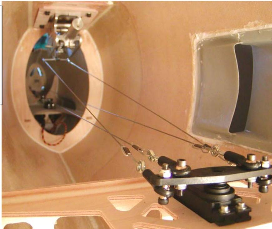
**NOTE:** Rudder servo ball links must be removed then reinstalled throughout this process as the cable loops are created and secured. Patience and perseverance are integral to successful completion. Be sure to allow extra adjustment on both the rudder clevis and servo ball link eyelet to take up what little cable slack remains once cables are properly completed.
