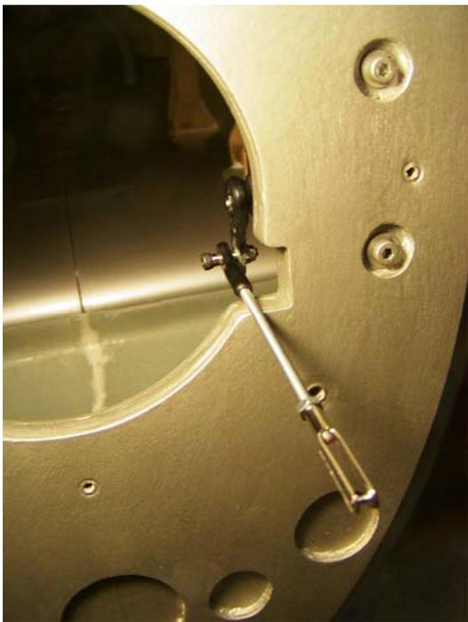
Throttle servo and pushrod installed
