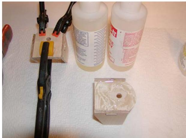
Side and top pieces are clamped then thick CA is used to glue side supports to top mount. Use epoxy to glue top mount doublers. Epoxy is used liberally and parts are tightly clamped to allow excess to squeeze into open spaces. Four mounts are constructed using the supplied wood parts. Once epoxy is set, sand and set aside.
