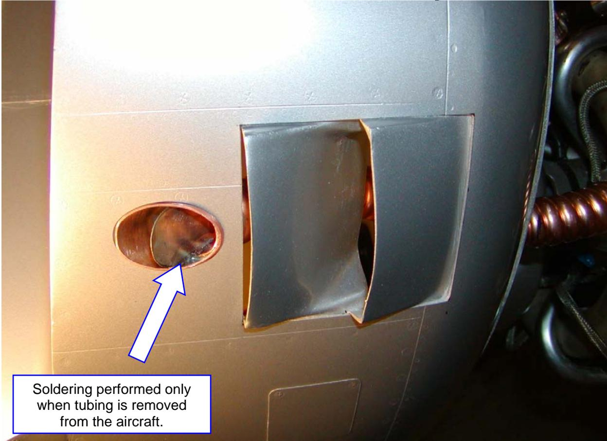
'Hose clamps' are utilized to secure the exhaust extensions to the Moki outlets. Slots should be cut into the copper pipe so that it can collapse under clamp pressure to fit tight and secure.
