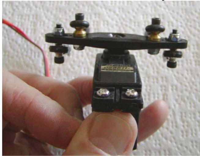
Mount the rudder servo in the pre-installed tray using the provided servo screws. Feed one tail wheel cable forward and through the ball link 'eyelet.' Grasping the excess cable from the tail wheel opening, PULL the cable tight to create a bend in the cable. This provides a marker for cable loop and length.
