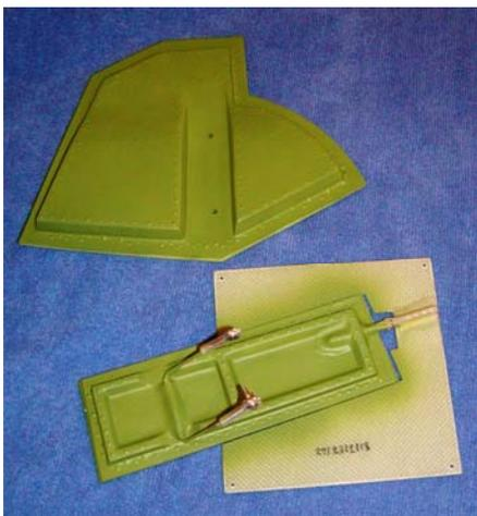
Water-based acrylic paints are very easy to use. By thinning with isopropyl alcohol, the paint dries extremely fast; fumes and overspray are kept to a minimum, and clean-up is fast and easy using soap and warm water. These paints add almost no weight and usually have a very opaque pigment that covers extremely well.
