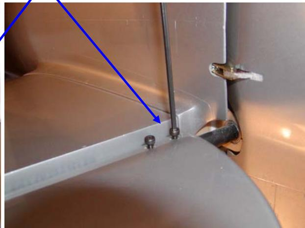
**Elevator retention bolts are threaded into the carbon fiber elevator torque rod. It is equally important that you NOT cross-thread or in any way force these bolts! If necessary, remove**
