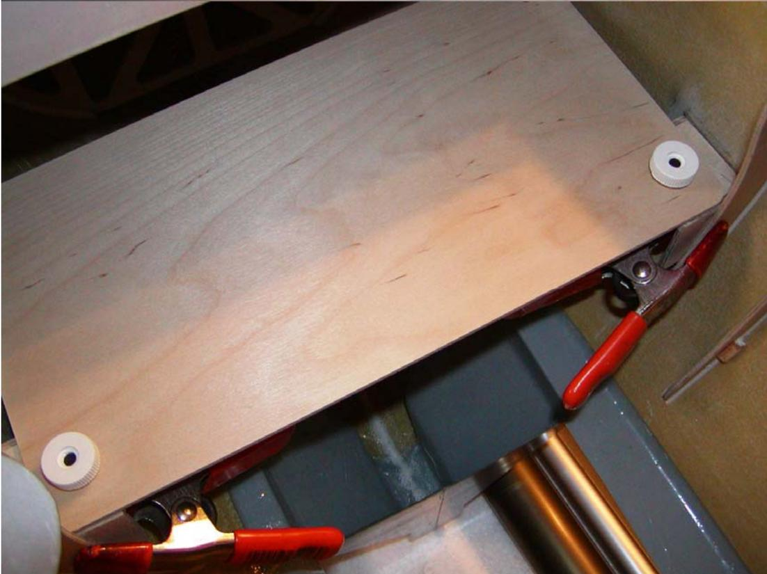
When the epoxy has set on the front mounts, locate the position of the rear mounts; mark the mounting holes and enlarge them to line up with the tray. Mark the position of the rear mounts; remove the tray; sand, clean and epoxy rear mounts in the same manner as the front mounts.
