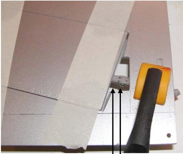
NOTE the distance from the bottom edge of strut cover to hinge pivot point – Approx. 6mm (1/4")
