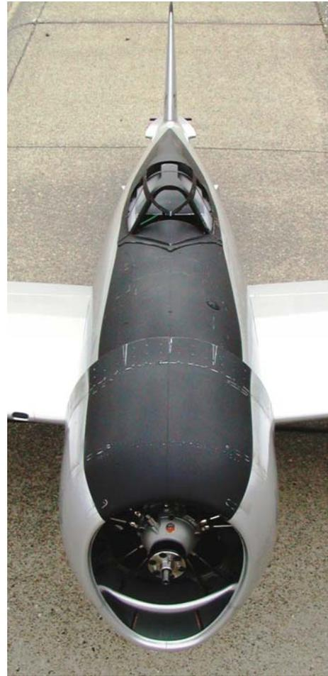
If your subject aircraft has a bare metal finish (and is not a polished museum exhibit), you can create the look of a “used” metal finish with an abrasive pad. The most common type is “Scotch Brite” – sometimes referred to as “scruffy pads.”
