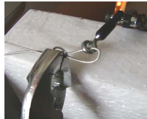
Perform this same procedure with the other tail wheel cable, making sure the tail wheel and rudder servo are **CENTERED BEFORE** crimping and cutting.
