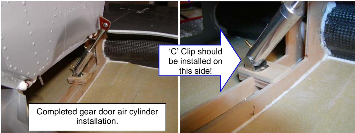
**Check gear door for proper open/close using hand pump. Main gear must also be checked for proper gear door clearance. NO RUBBING, NO TOUCHING! If it rubs on the ground, it will HANG UP in FLIGHT!**
