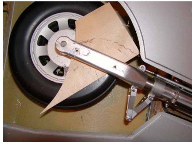
Once holes are drilled through the wheel cover and a few millimeters into gear legs, remove wheel cover. Insert scrap ply between gear legs and wheels to protect from drill bit and finish drilling holes. Holes are then tapped for the 3mm countersunk wheel cover screws.
