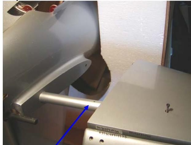
**DO NOT** cross-thread or in any way force stab or elevator bolts when installing. IF any resistance is encountered, REMOVE stab and elevator and verify bolts will easily thread into their respective locations.
