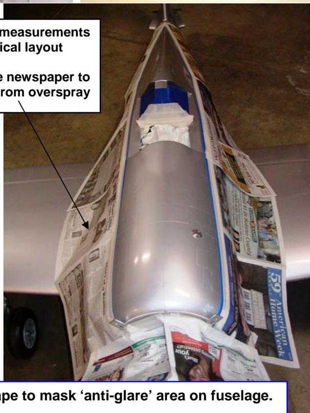
Using flexible automotive painters tape to mask ‘anti-glare’ area on fuselage.
