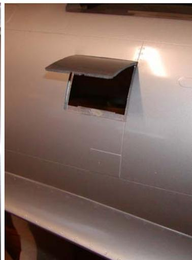
**Air Outlet and Turbo-Supercharger Outlet Covers**
