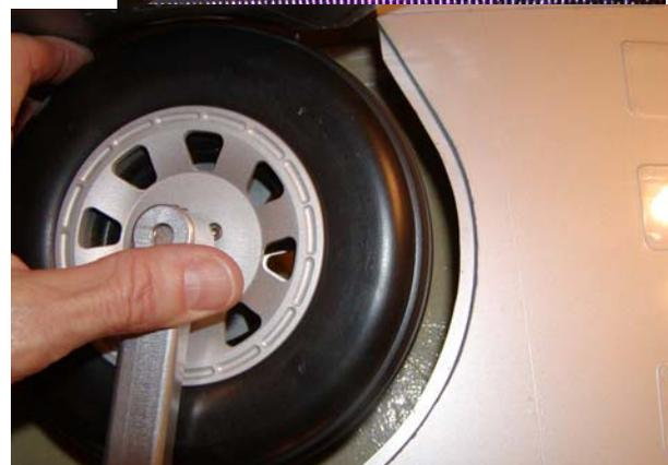
Check and re-check for proper clearances and smooth gear retraction.
